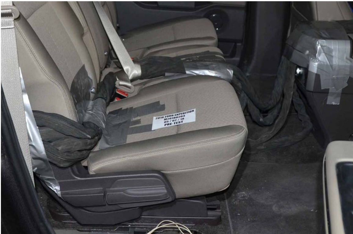
FIGURE 28. Pre-Test Dummy Cable Routing
