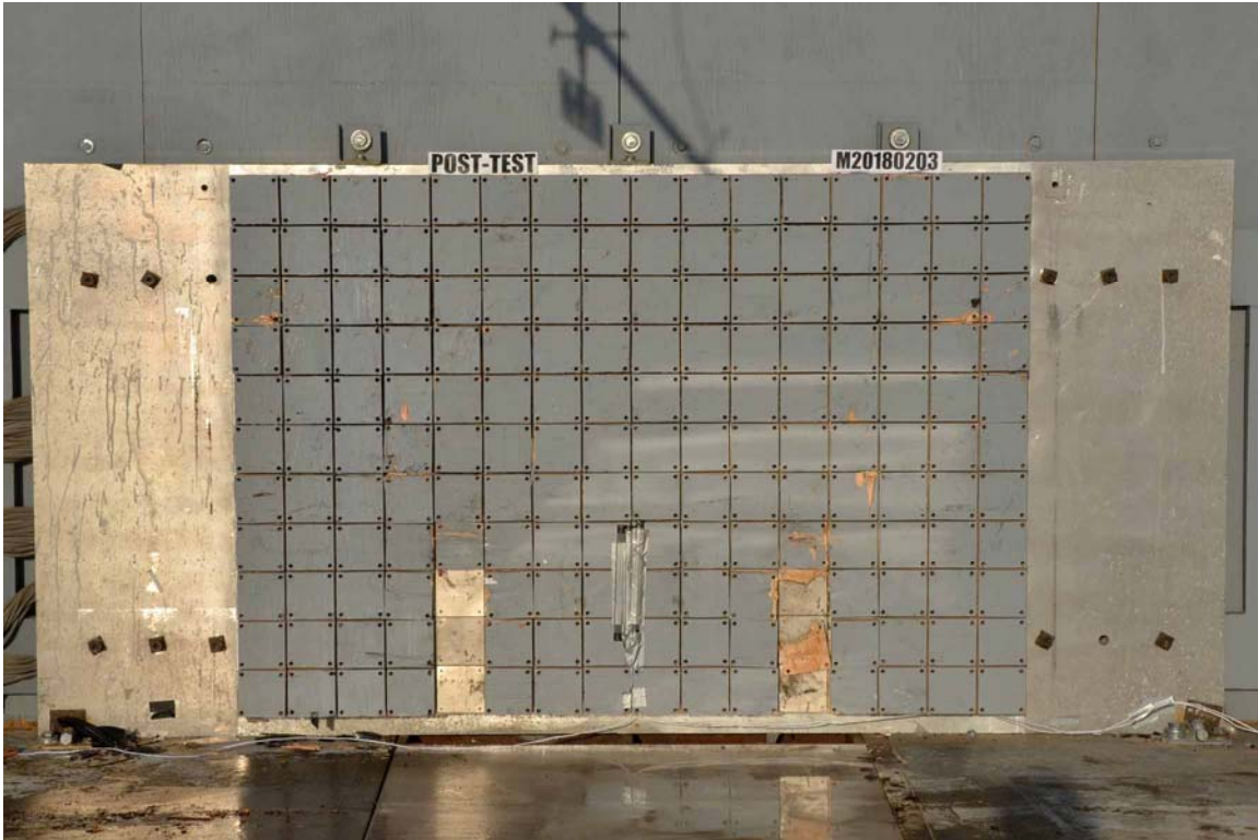
FIGURE 3. Post-Test Load Cell Wall
