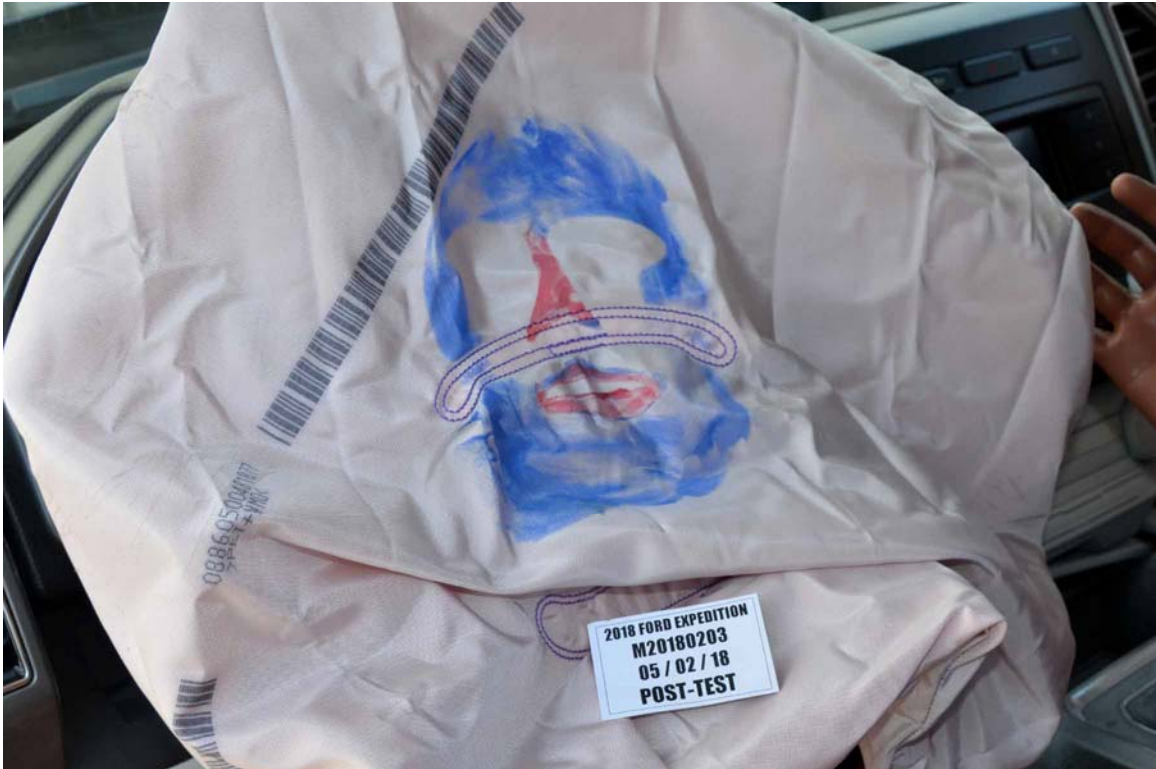
FIGURE 47. Post-Test Driver Dummy Contact with Airbag
