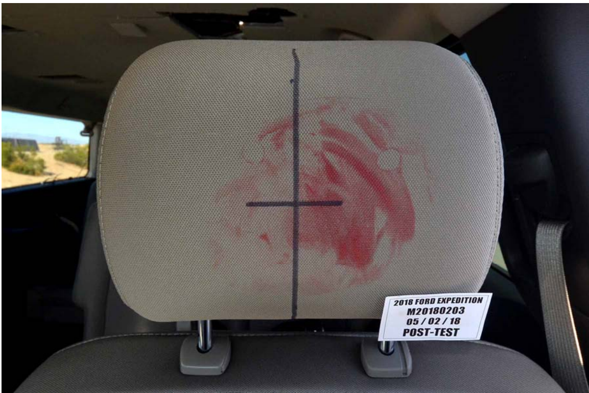
FIGURE 48. Post-Test Driver Dummy Contact with Headrest
