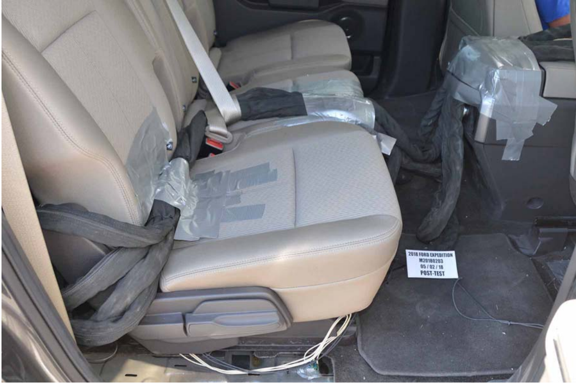
FIGURE 29. Post-Test Dummy Cable Routing
