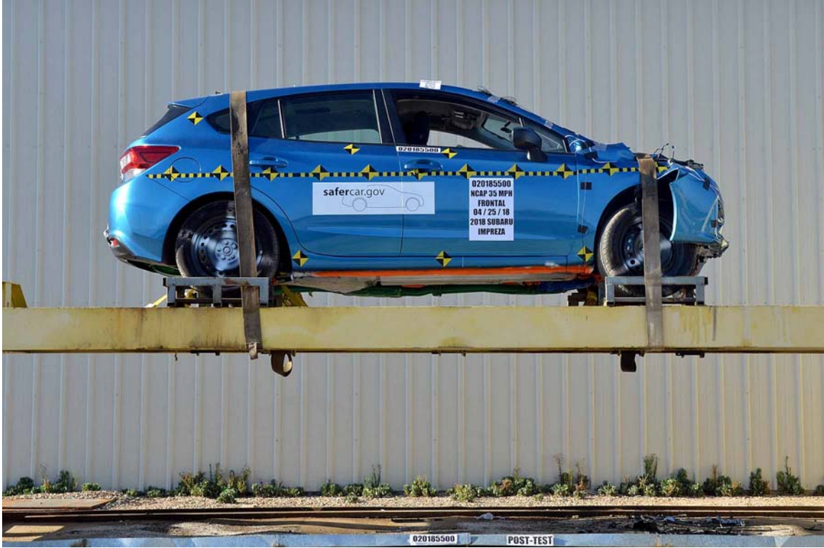
FIGURE 77. Vehicle at 360° on Static Rollover Device
