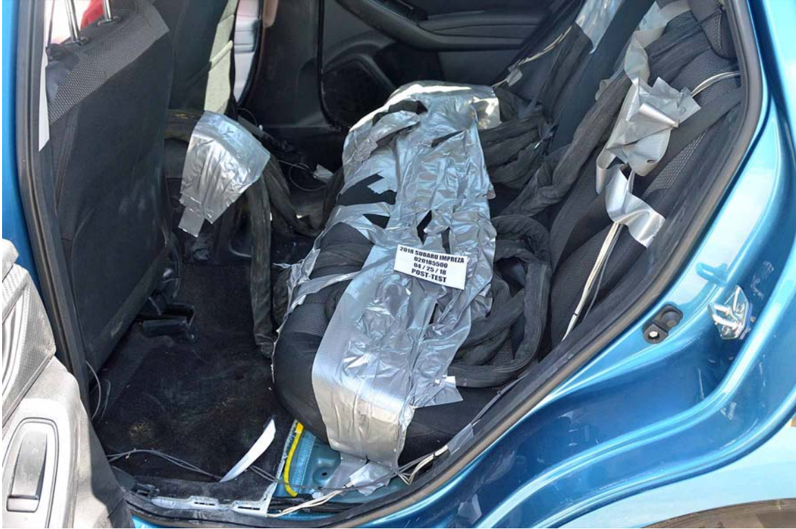
FIGURE 29. Post-Test Dummy Cable Routing
