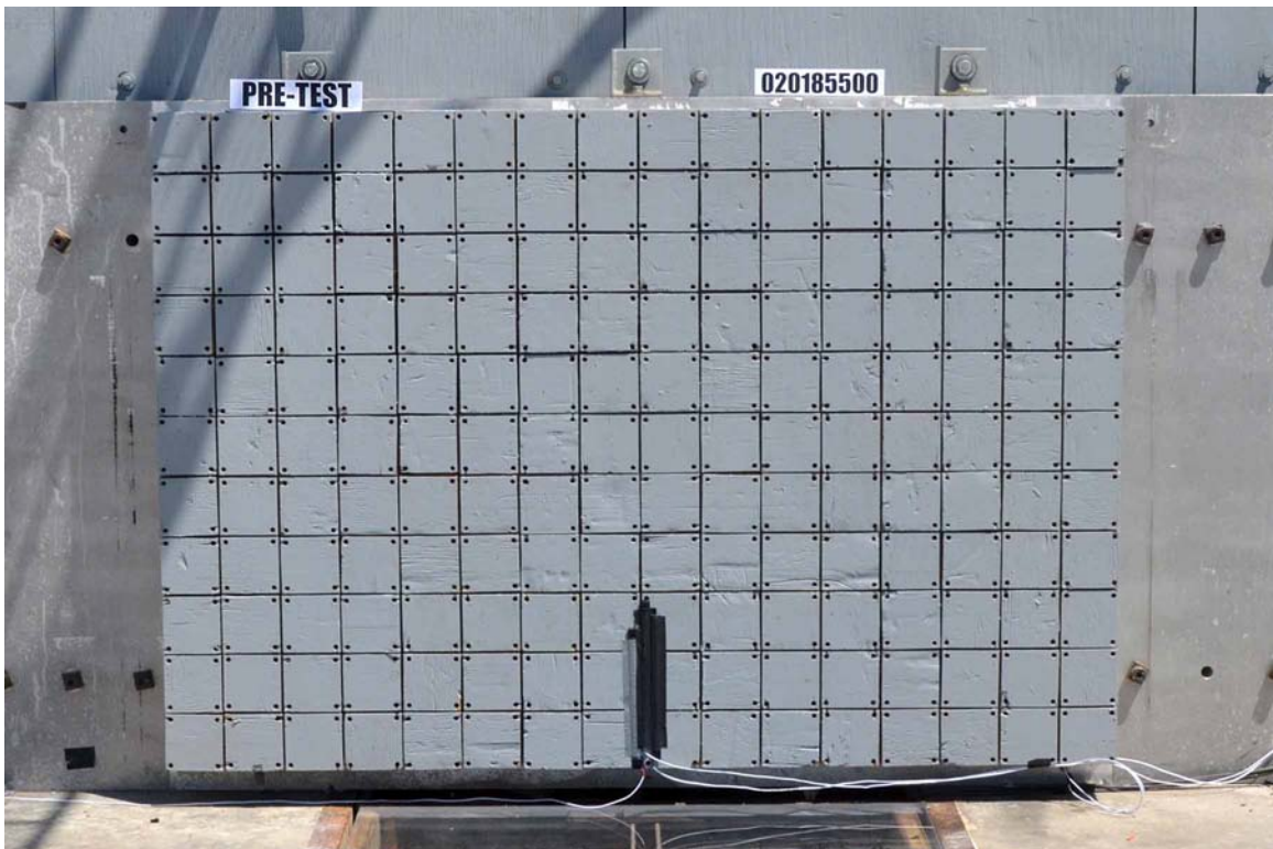
FIGURE 2. Pre-Test Load Cell Wall
