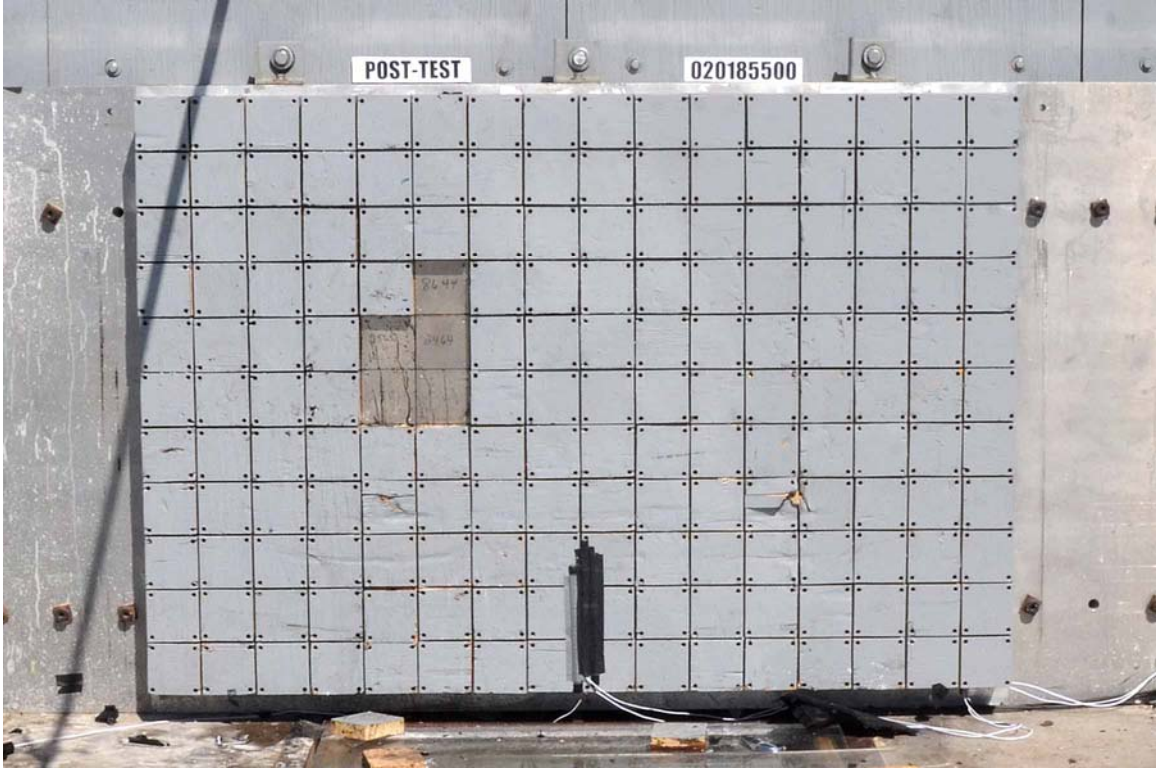
FIGURE 3. Post-Test Load Cell Wall
