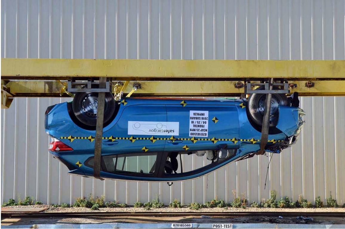
FIGURE 75. Vehicle at 180° on Static Rollover Device
