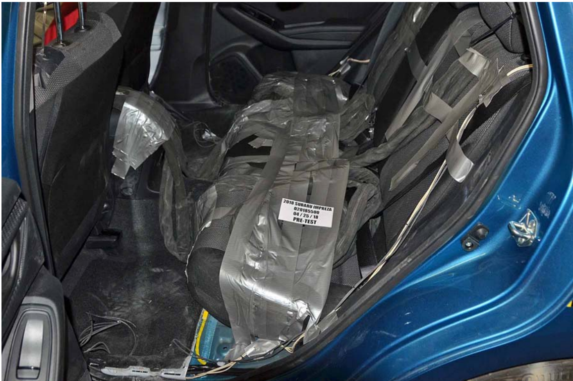
FIGURE 28. Pre-Test Dummy Cable Routing
