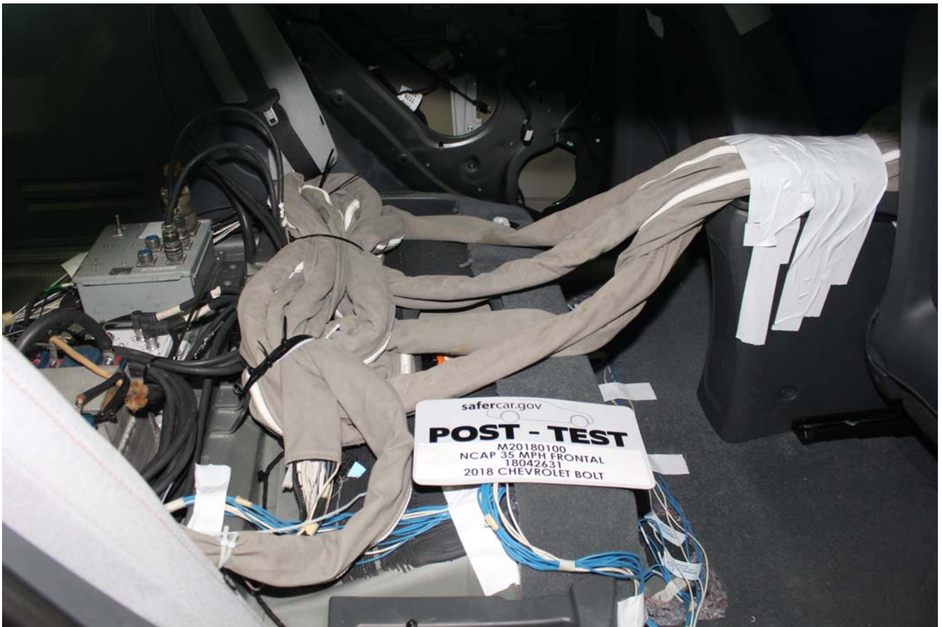
Photo No. 029 - Post-Test Dummy Cable Routing
