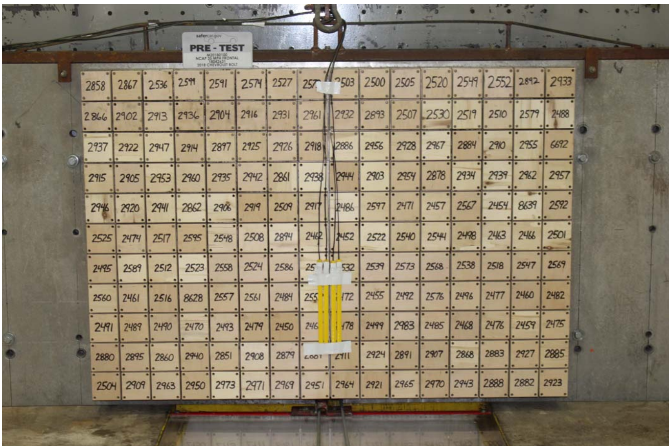
Photo No. 002 - Pre-Test Load Cell Wall
