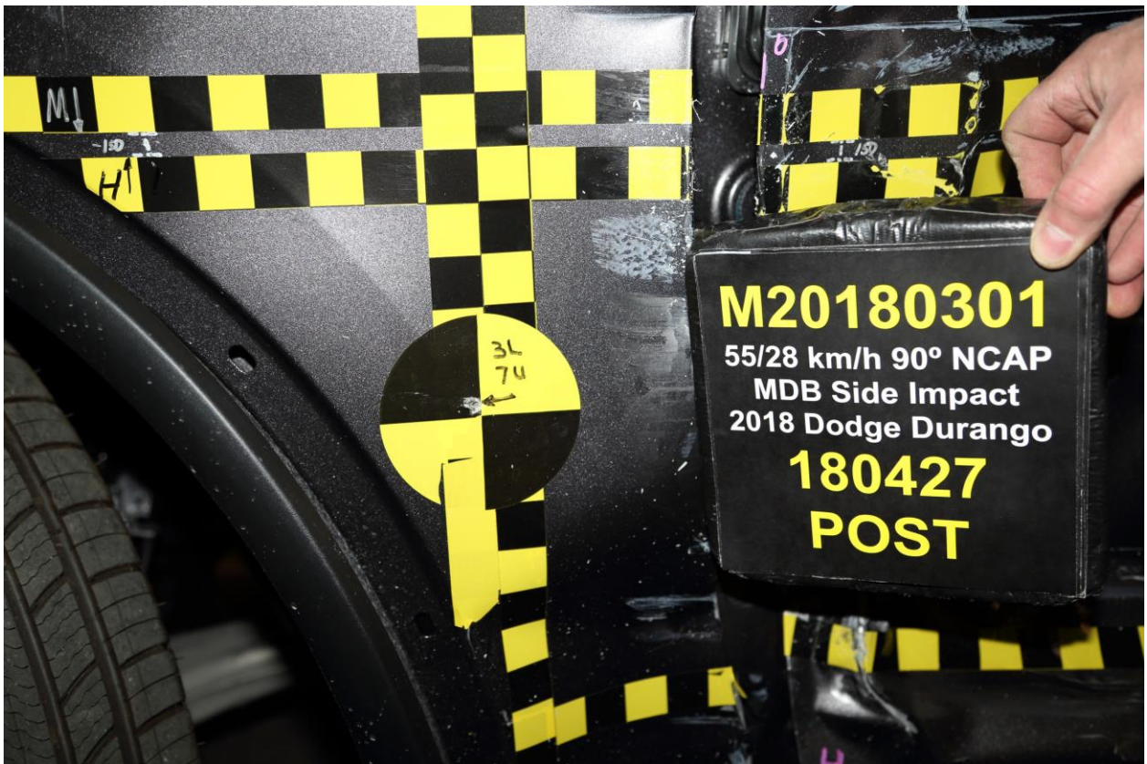
020 Post-Test Close-Up View of Impact Point Target
