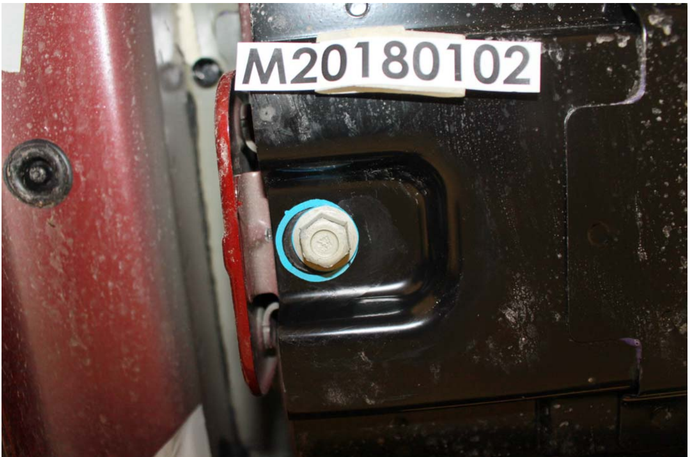
Photo No. 035 - Post-Impact View of Battery Module Movement or Retention Loss
