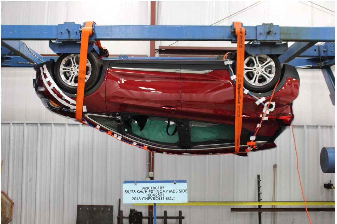
Photo No. 028 - FMVSS No. 305 Static Rollover at 180°
