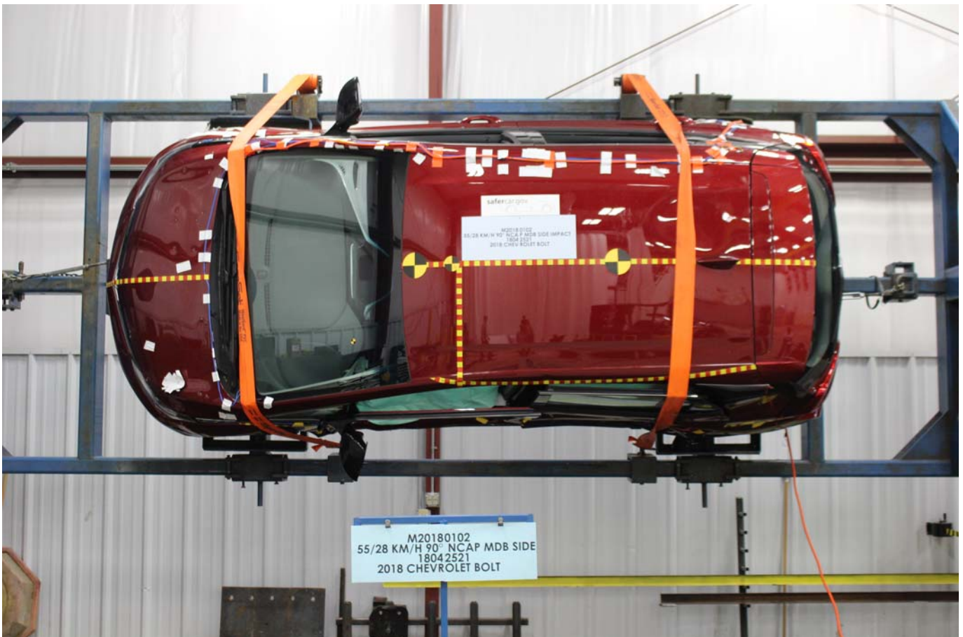
Photo No. 027 - FMVSS No. 305 Static Rollover at 90°
