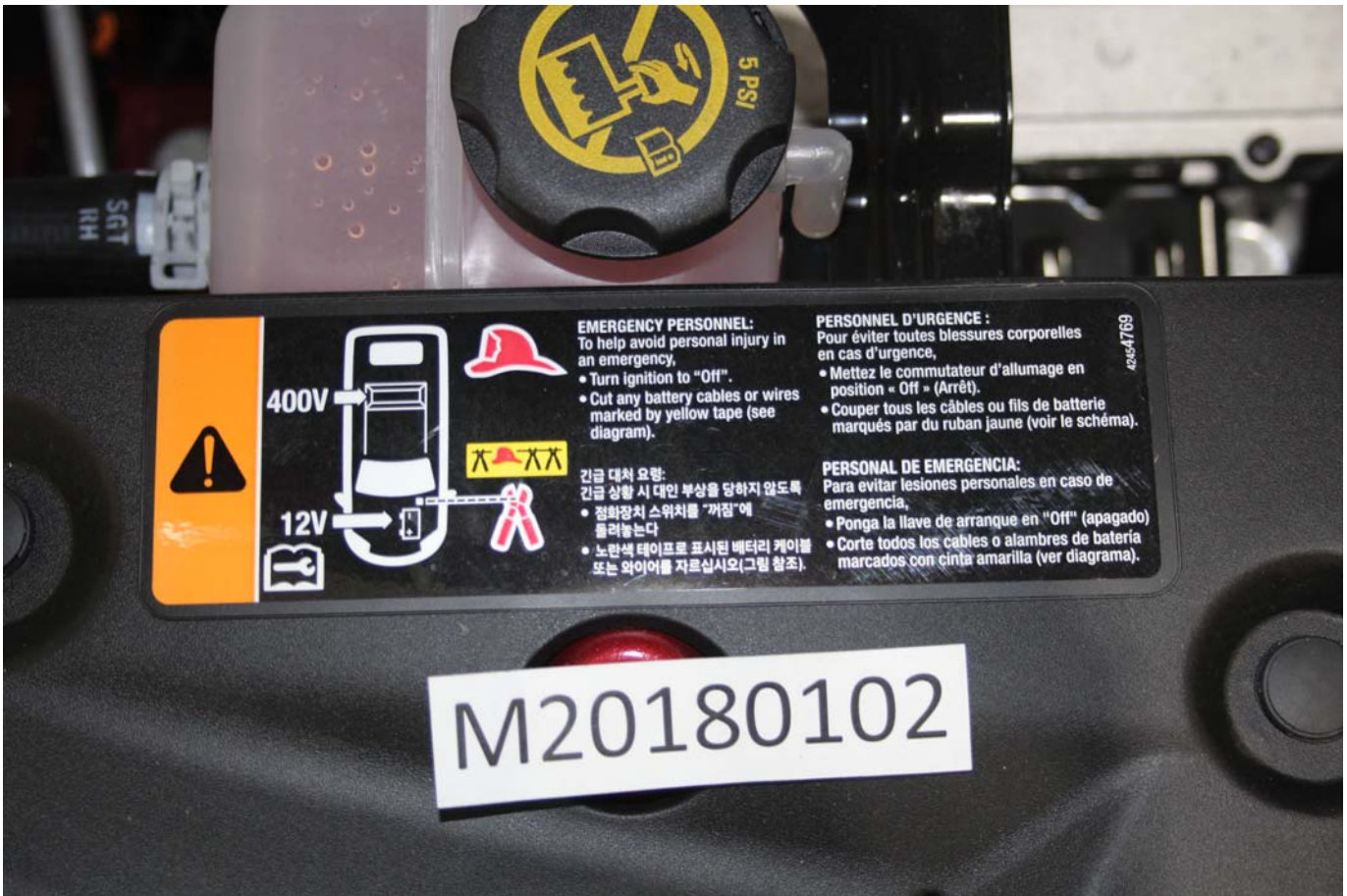
Photo No. 003 - First Responder Warning Label
