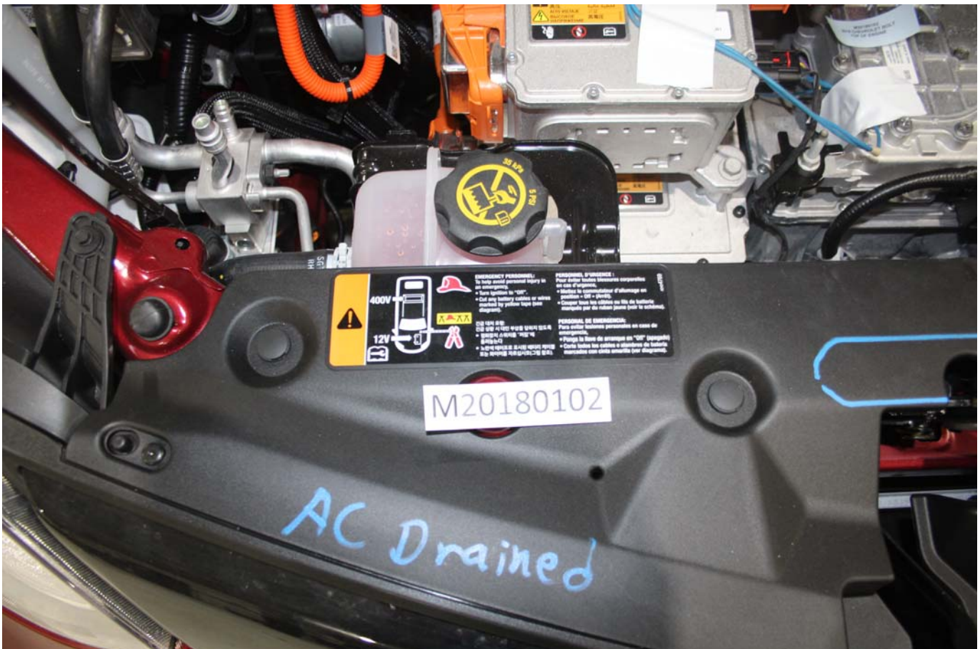
Photo No. 004 - First Responder Warning Location
