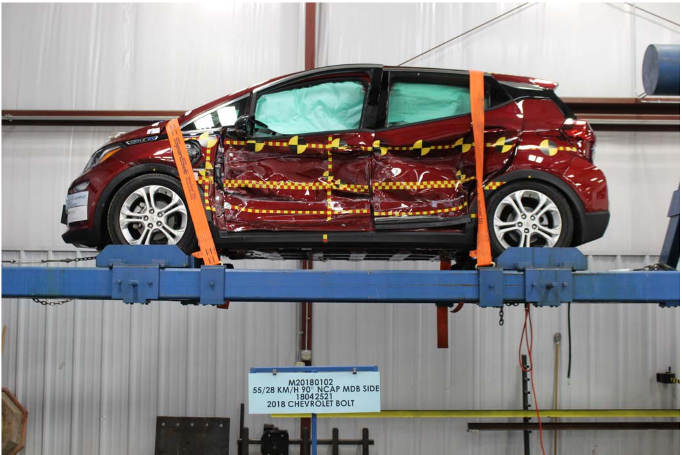
Photo No. 030 - FMVSS No. 305 Static Rollover at 360°
