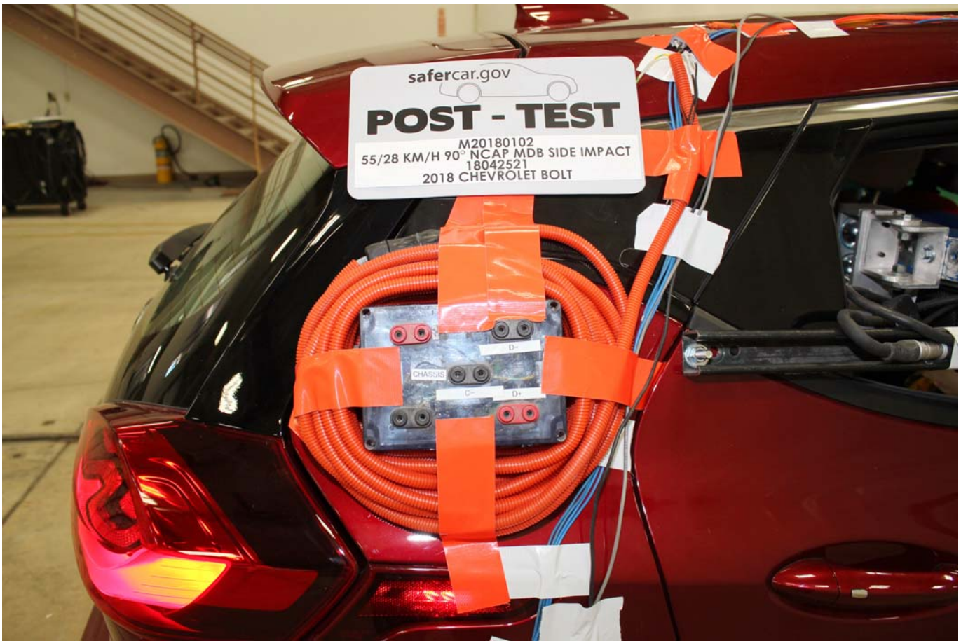
Photo No. 024 - Post-Impact View of Installed Impact Interface Port
