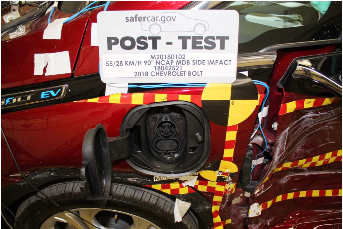
Photo No. 083 - Post-test Fuel Filler Cap-Charge Port View
