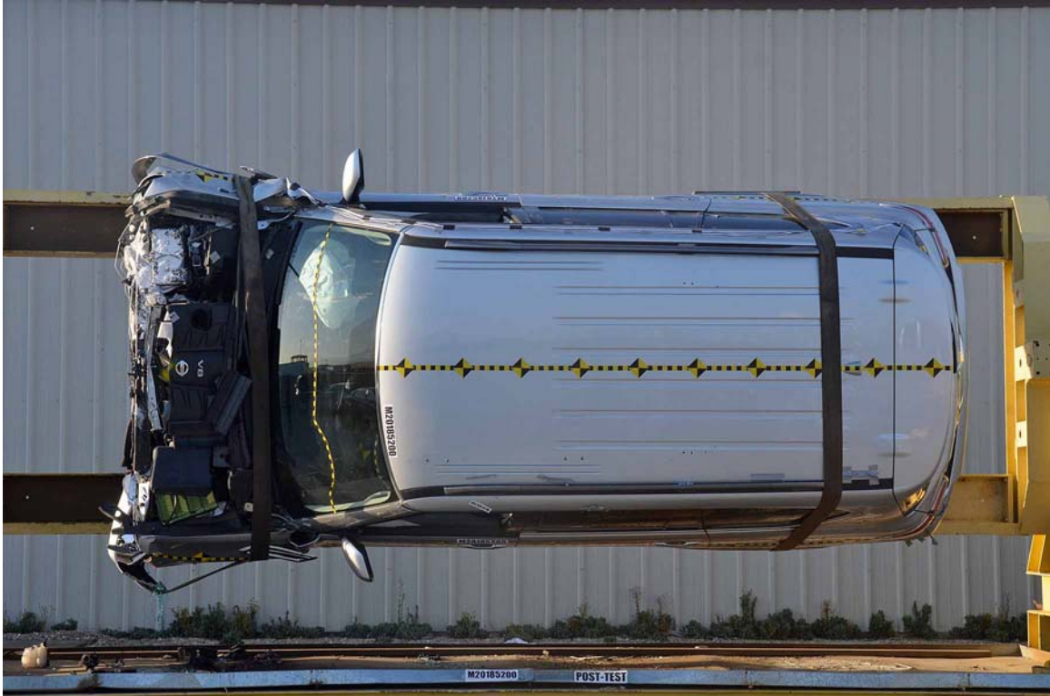
FIGURE 74. Vehicle at 90° on Static Rollover Device
