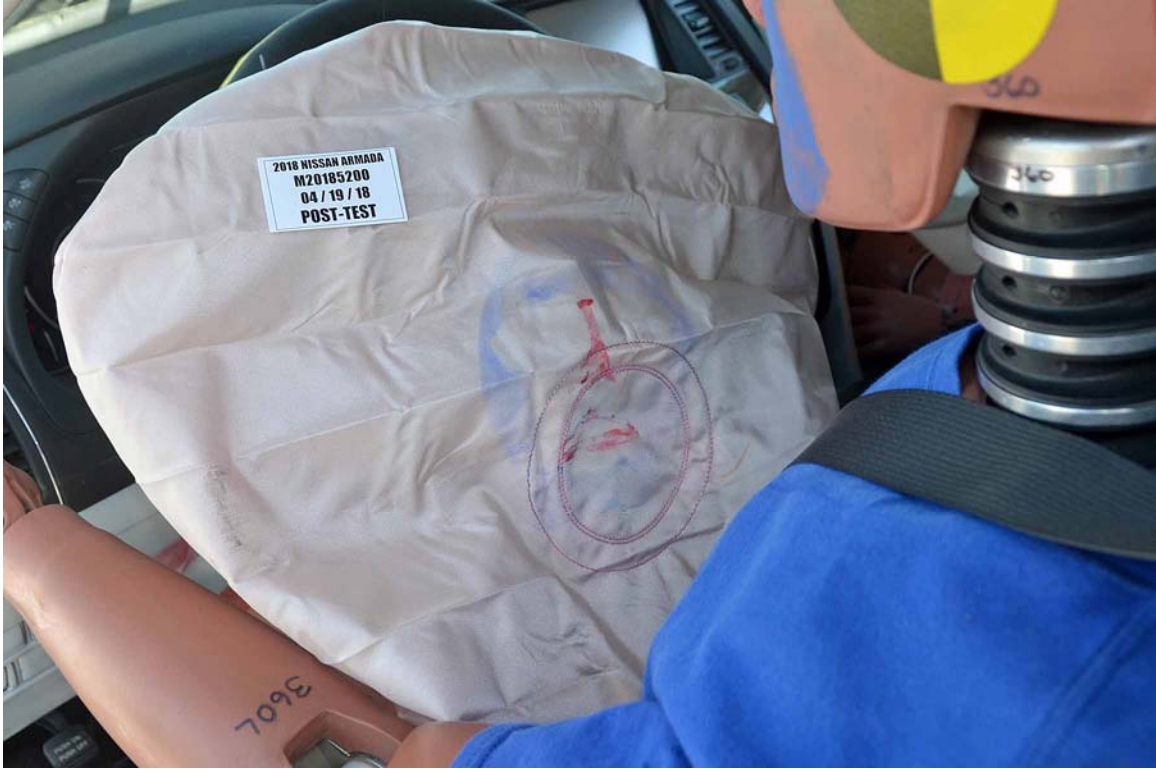
FIGURE 47. Post-Test Driver Dummy Contact with Airbag
