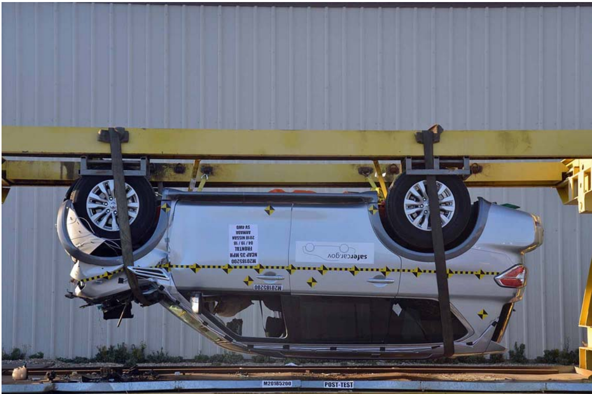
FIGURE 75. Vehicle at 180° on Static Rollover Device
