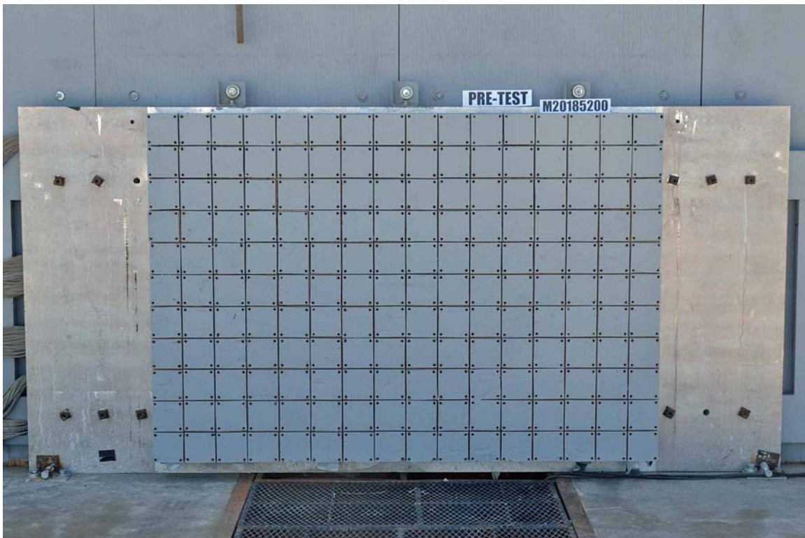
FIGURE 2. Pre-Test Load Cell Wall
