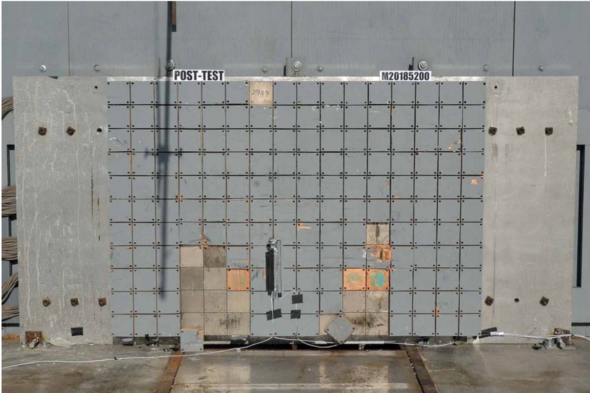
FIGURE 3. Post-Test Load Cell Wall
