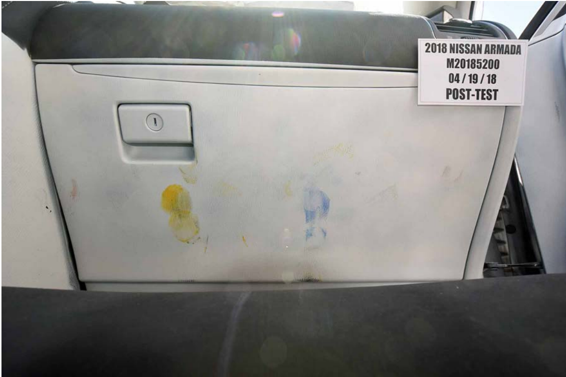
FIGURE 64. Post-Test Passenger's Side Knee Bolster
