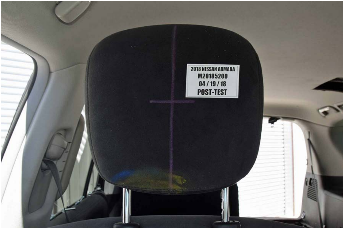
FIGURE 69. Post-Test Passenger Dummy Contact with Headrest
