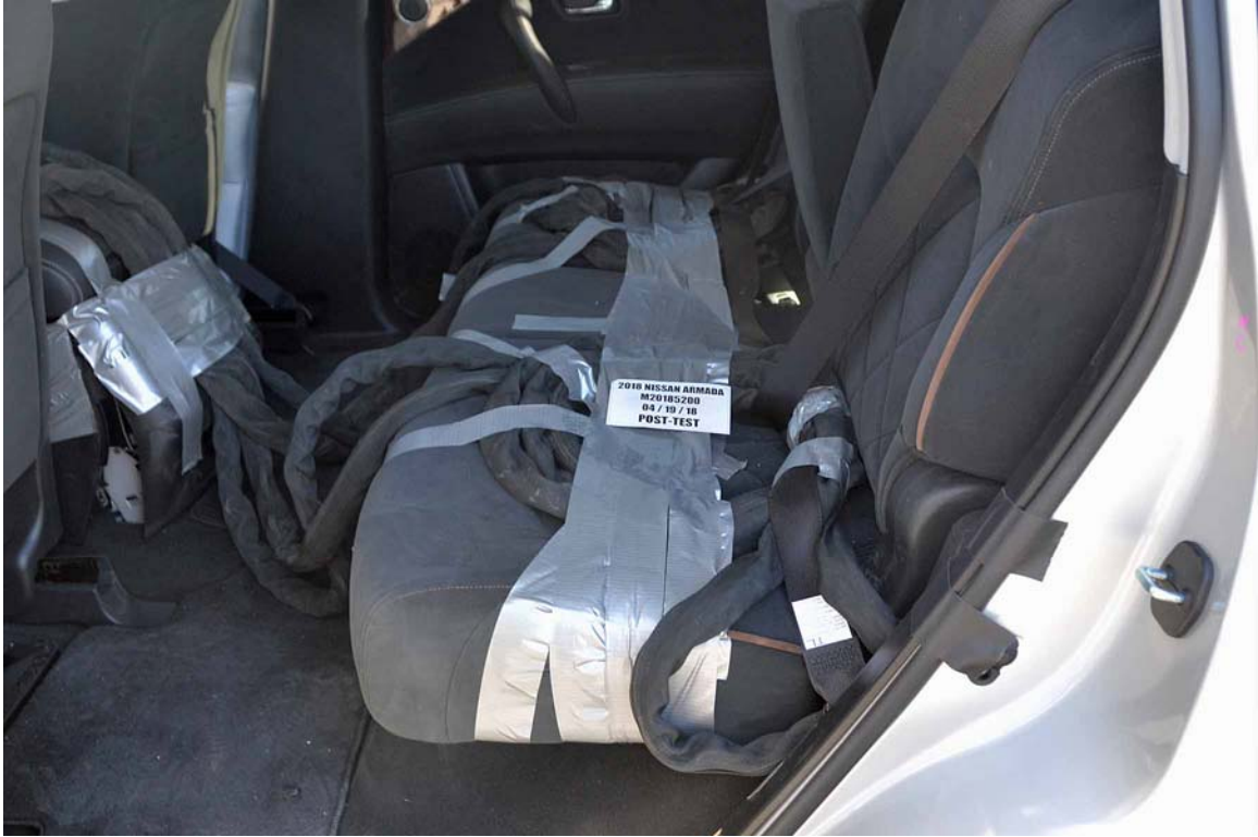
FIGURE 29. Post-Test Dummy Cable Routing
