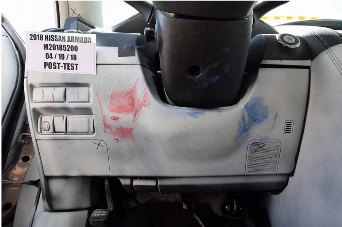
FIGURE 43. Post-Test Driver's Side Knee Bolster
