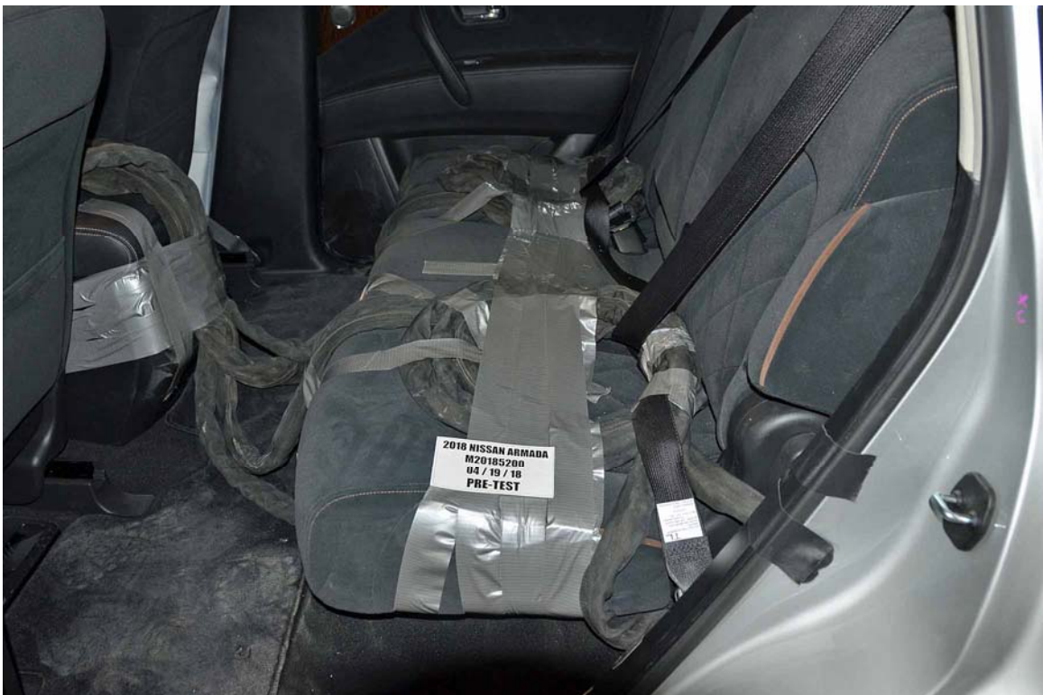
FIGURE 28. Pre-Test Dummy Cable Routing
