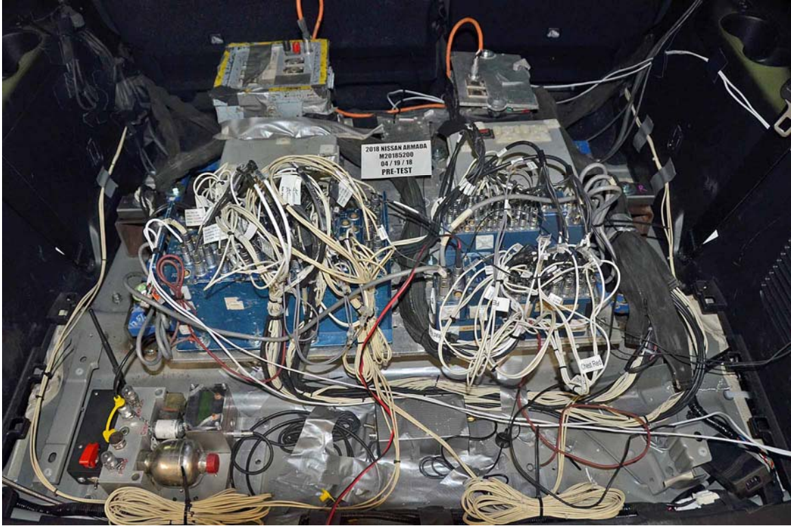
FIGURE 70. Photograph of Ballast Installed in Vehicle
