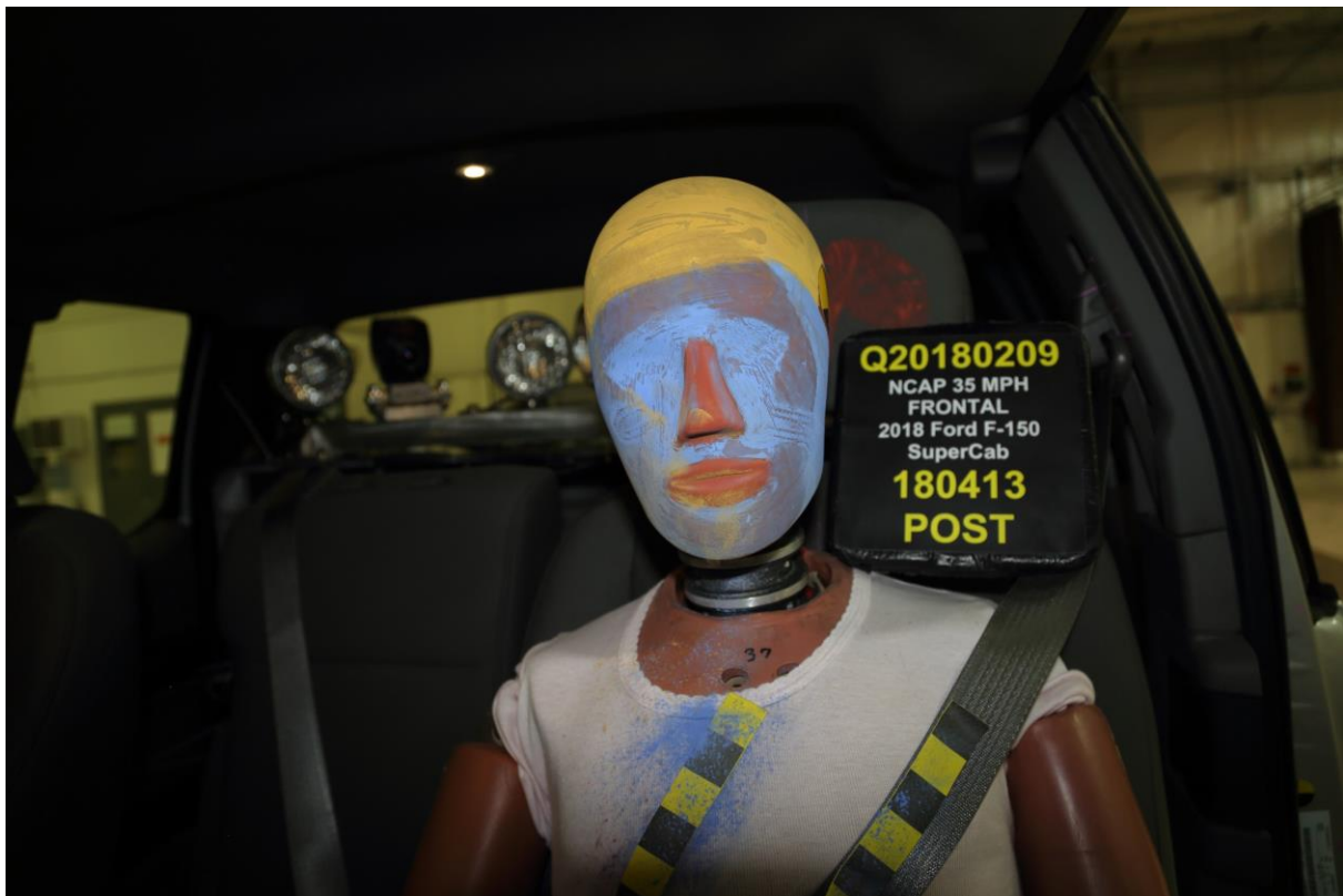
046 Post-Test Driver Dummy Face
