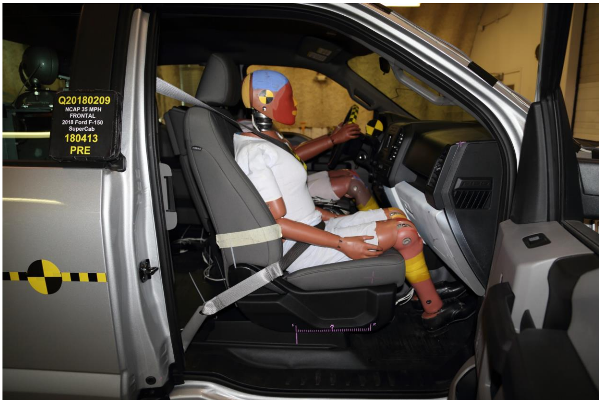
055 Pre-Test Passenger Dummy and Vehicle Interior View
