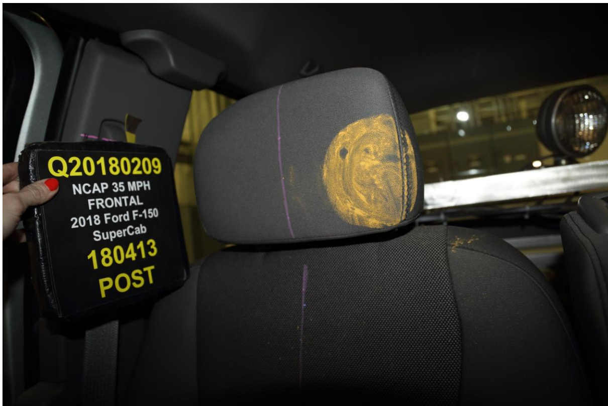
069 Post Test Passenger Dummy Contact With Headrest
