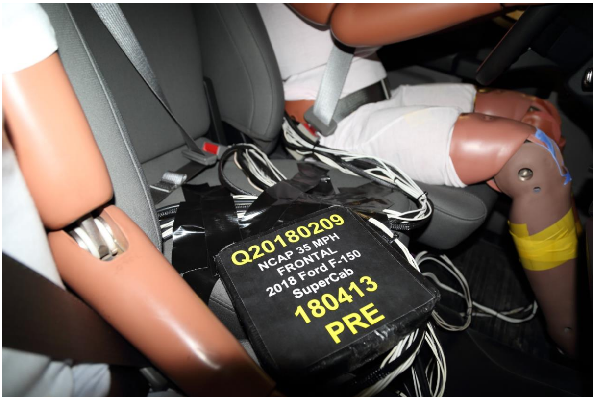
028 Pre-Test Dummy Cable Routing
