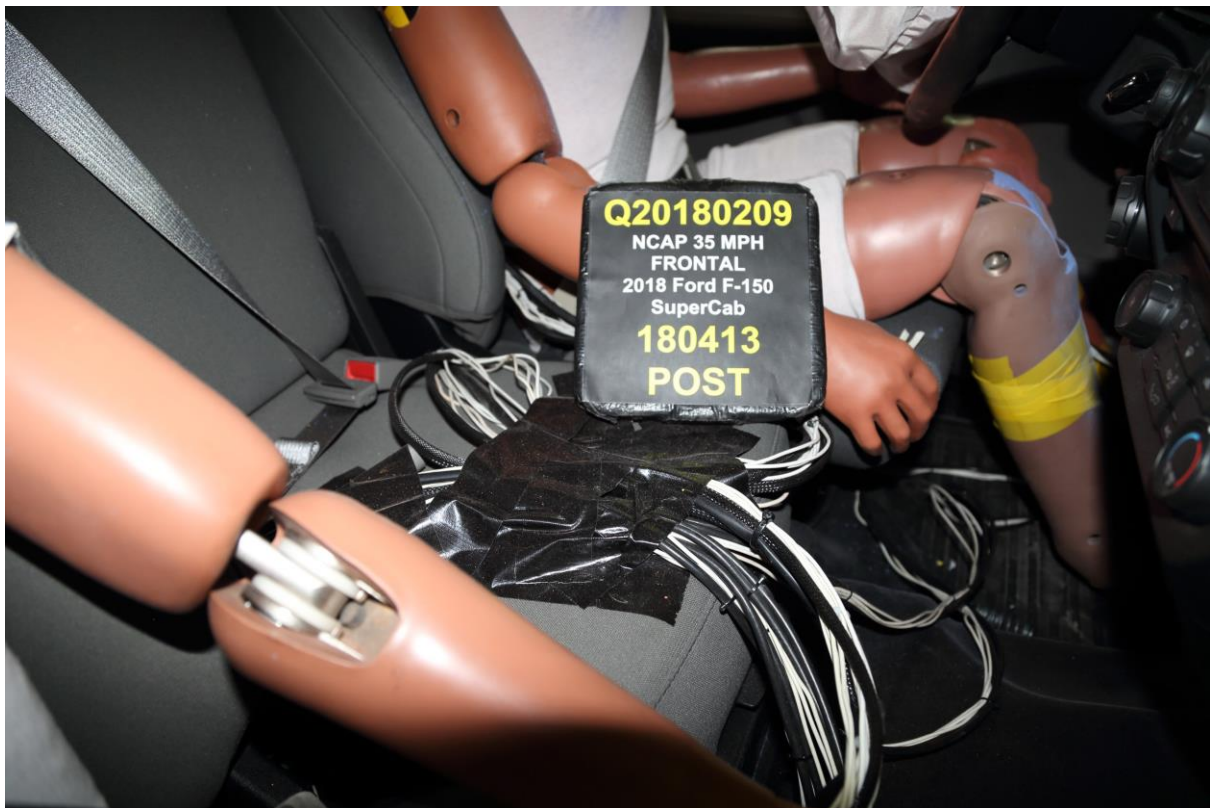
029 Post-Test Dummy Cable Routing
