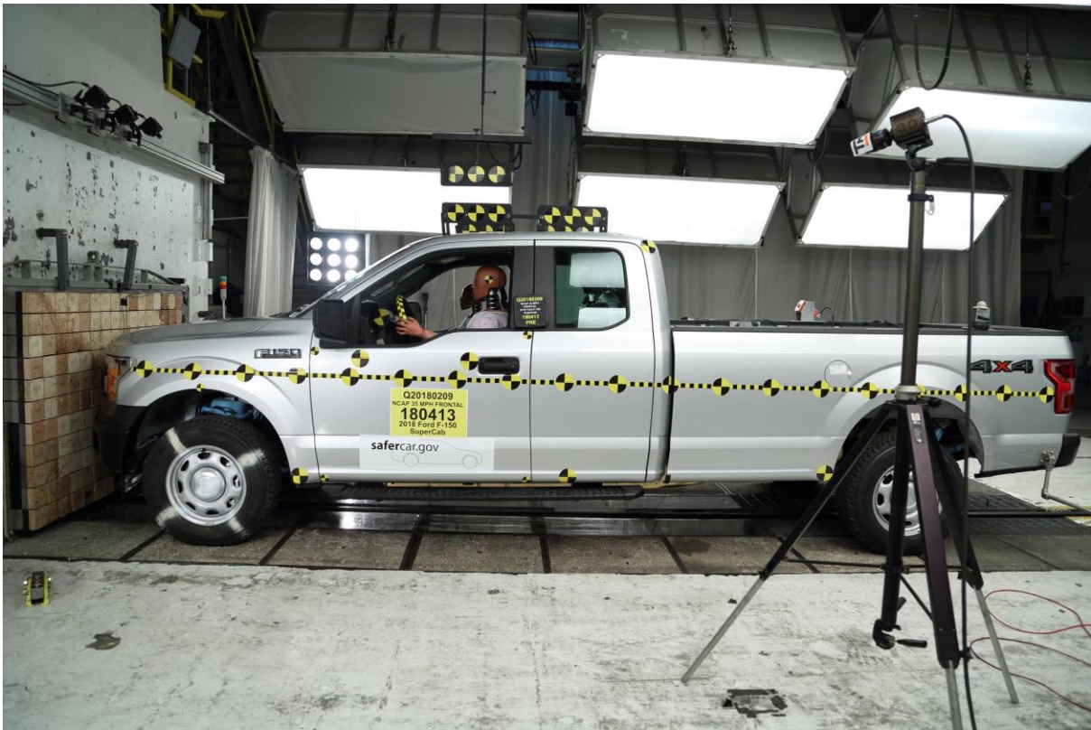
010 Pre-Test Left View of Test Vehicle
