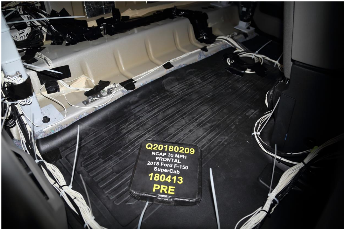
028a Pre-Test Dummy Cable Routing
