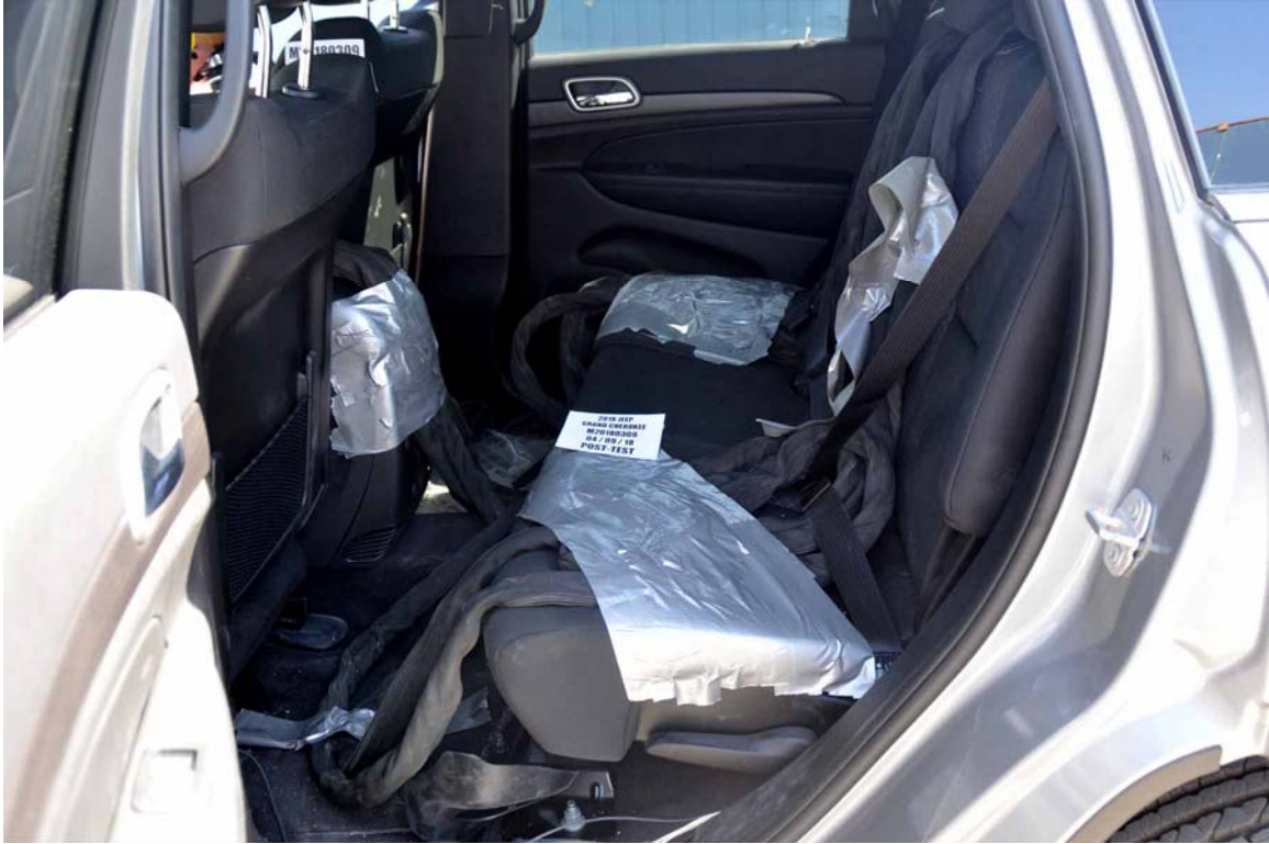
FIGURE 29. Post-Test Dummy Cable Routing
