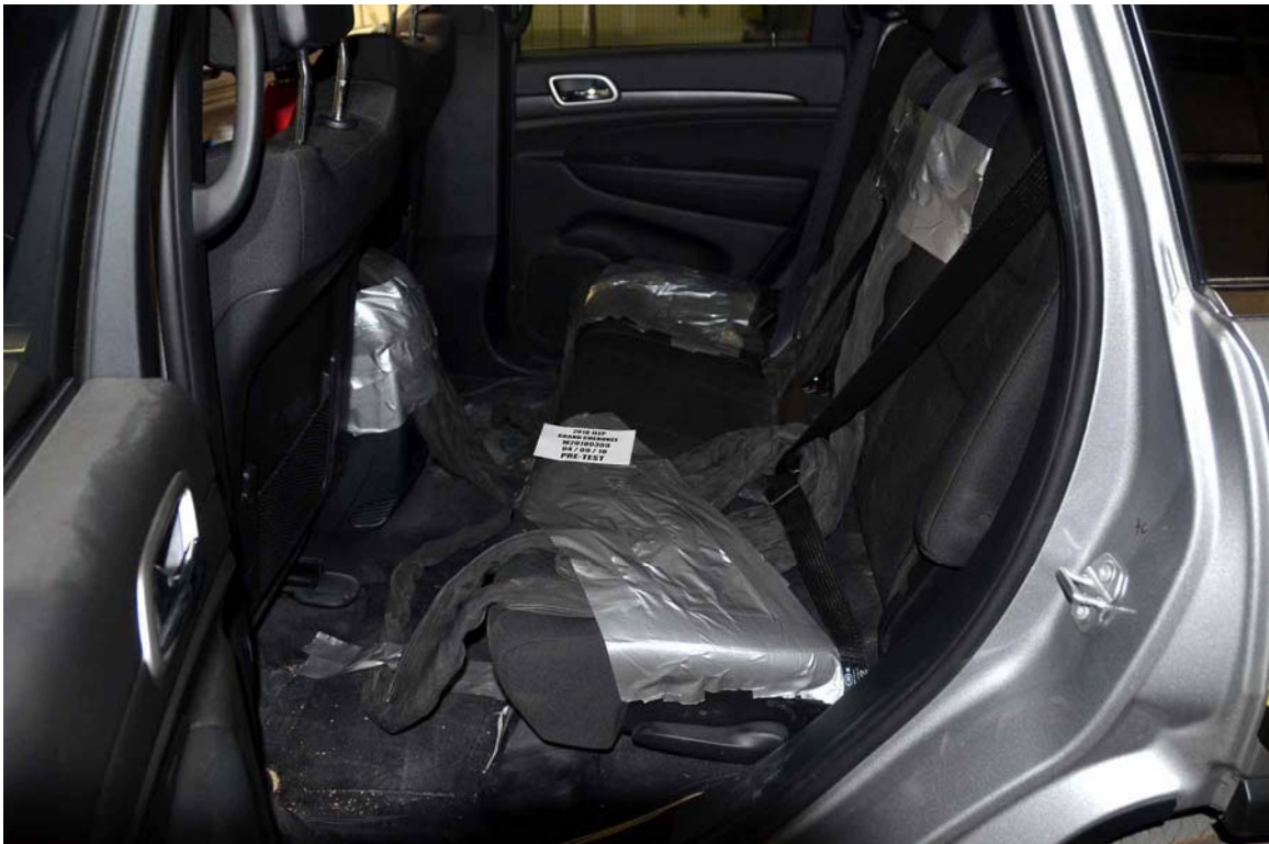
FIGURE 28. Pre-Test Dummy Cable Routing
