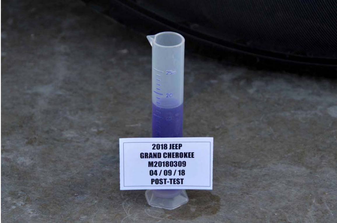
FIGURE 71b. Post-Test Stoddard Solvent Spillage Location View
