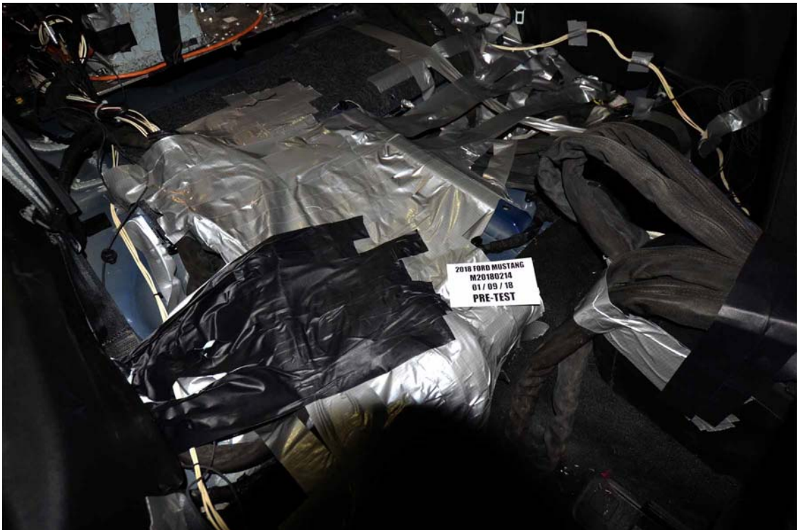
FIGURE 28. Pre-Test Dummy Cable Routing
