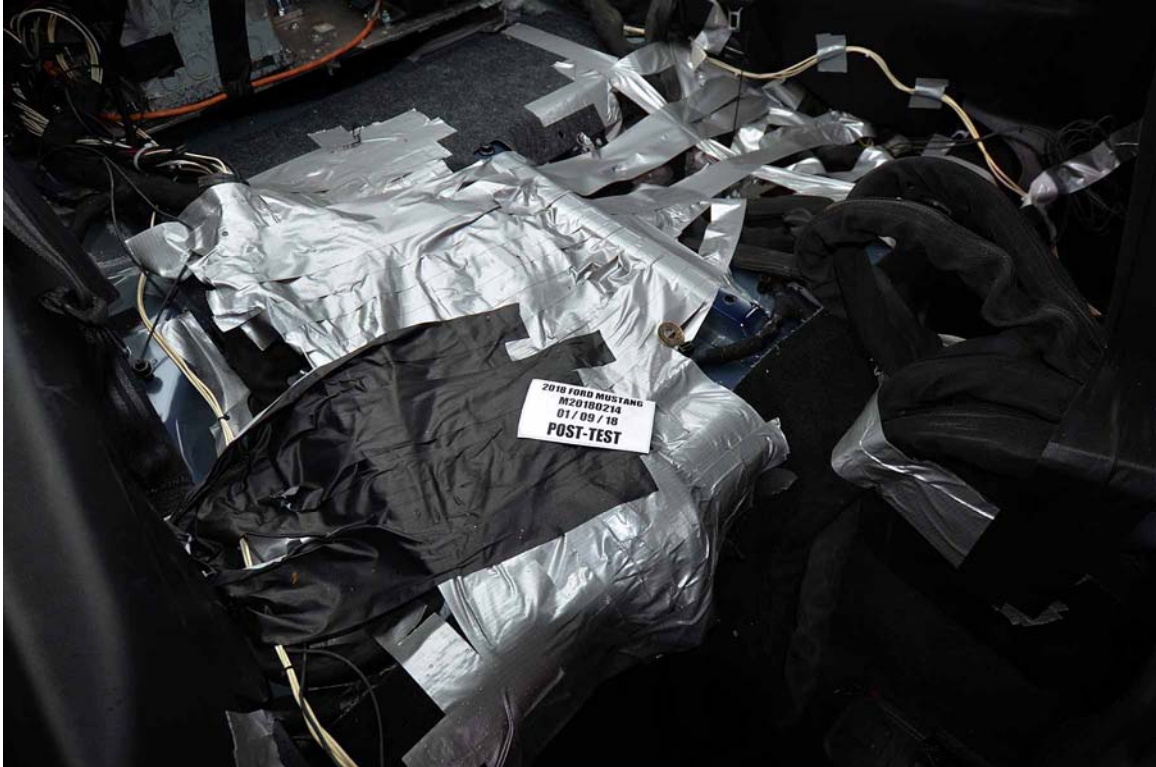
FIGURE 29. Post-Test Dummy Cable Routing
