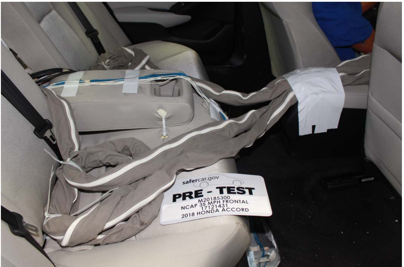
Photo No. 028 - Pre-Test Dummy Cable Routing
