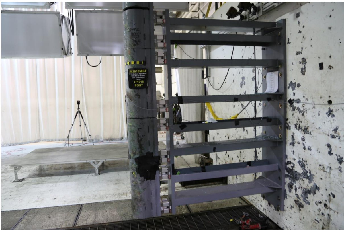
No. 060 Post-Test Pole Barrier Side View
