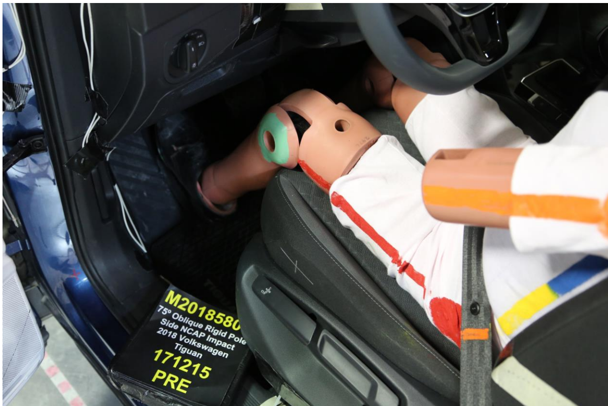
No. 032 Pre-Test Placement of Dummy Feet
