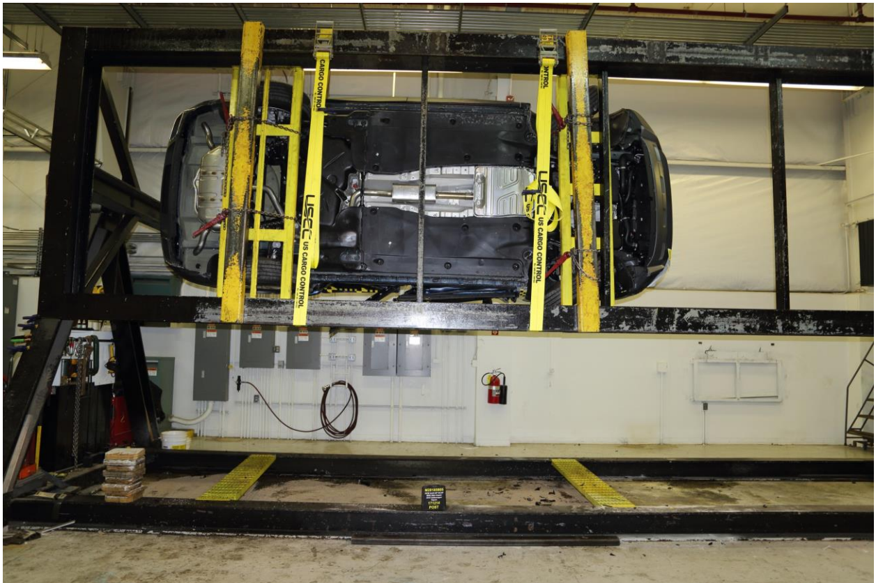
099 FMVSS No. 301 Static Rollover 270 Degrees
