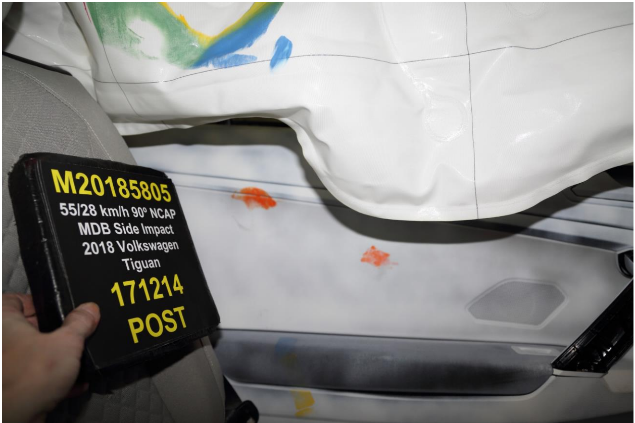
077 Post-Test Rear Passenger Dummy Close-Up Torso Contact with Vehicle Interior View
