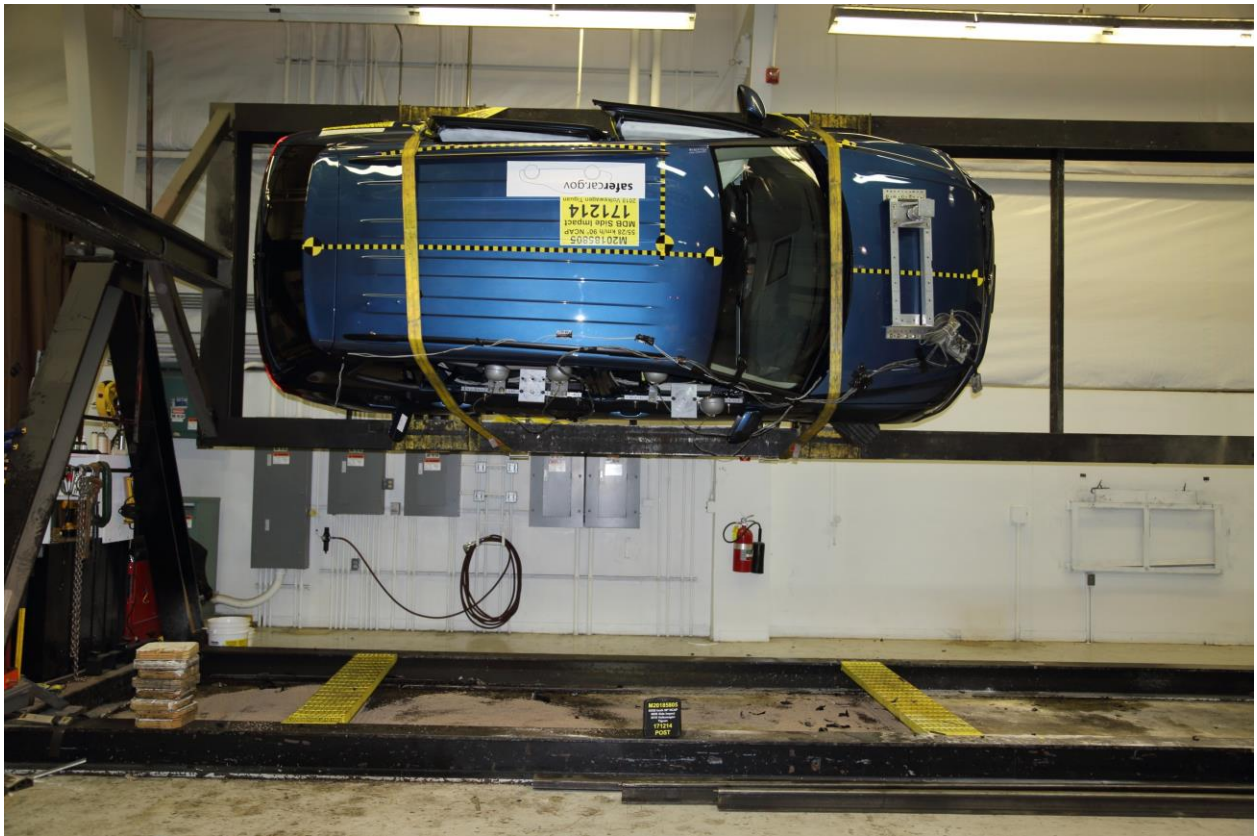
097 FMVSS No. 301 Static Rollover 90 Degrees
