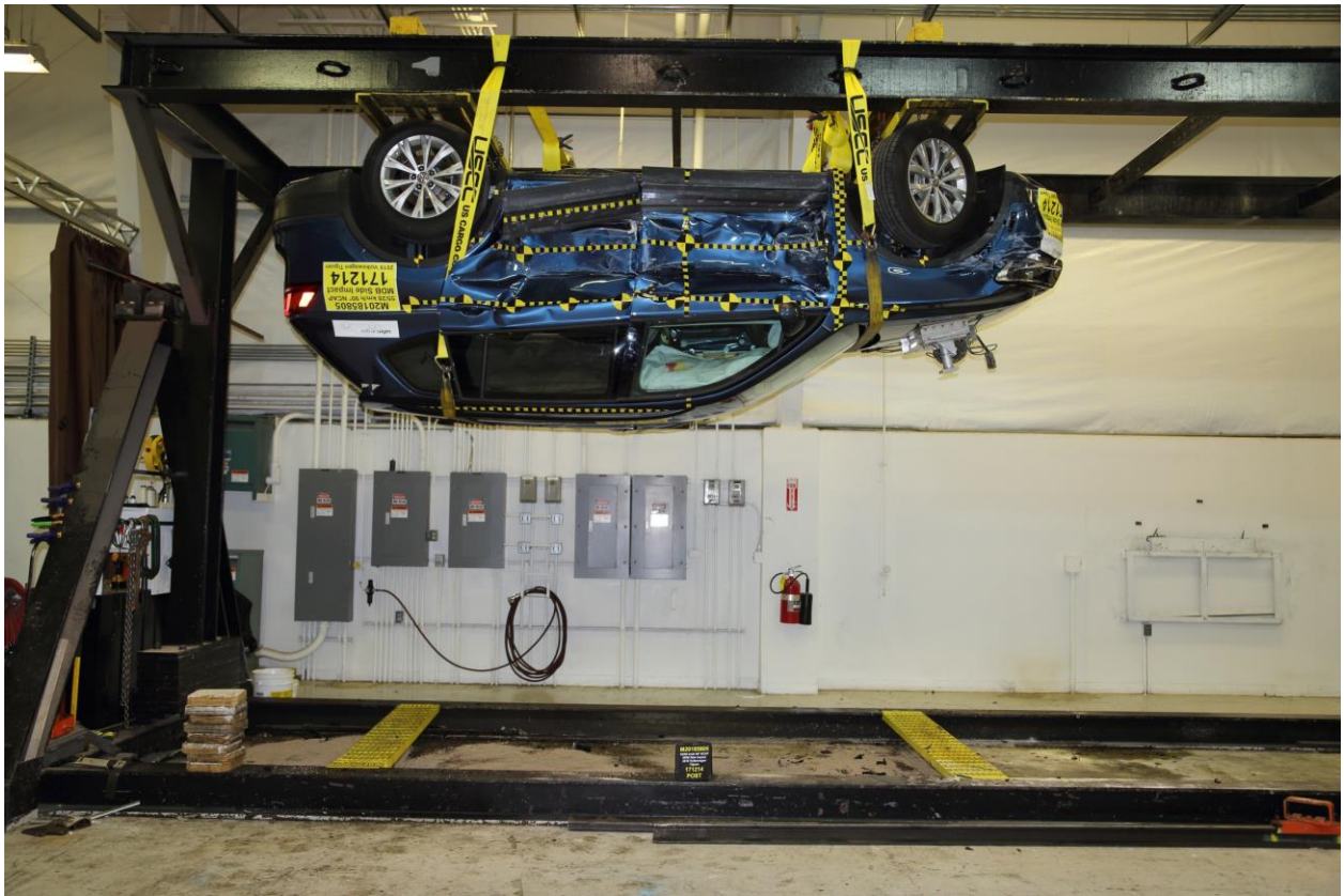
098 FMVSS No. 301 Static Rollover 180 Degrees
