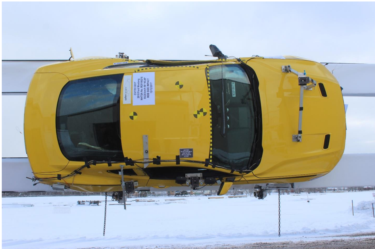
Figure A-99: FMVSS No. 301 Static Rollover 270 Degrees
