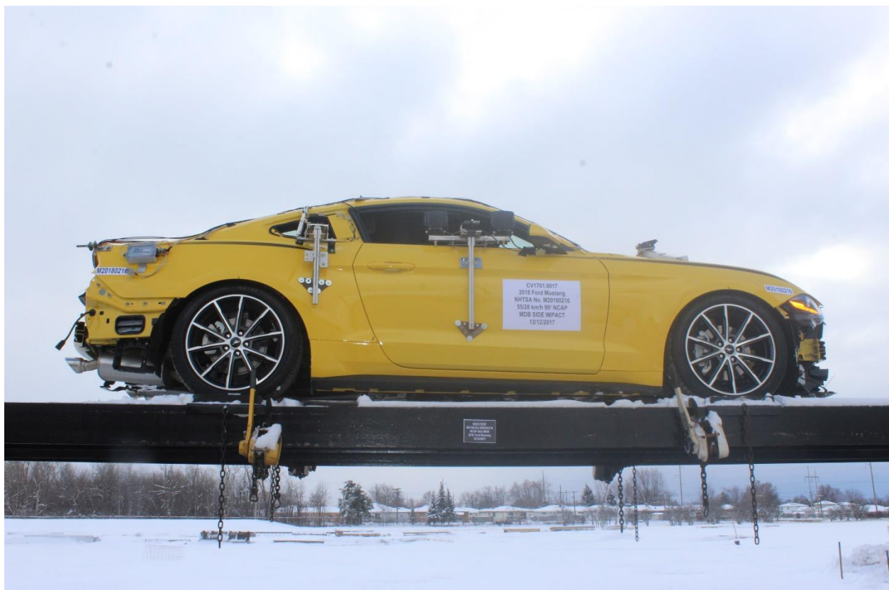
Figure A-100: FMVSS No. 301 Static Rollover 360 Degrees
