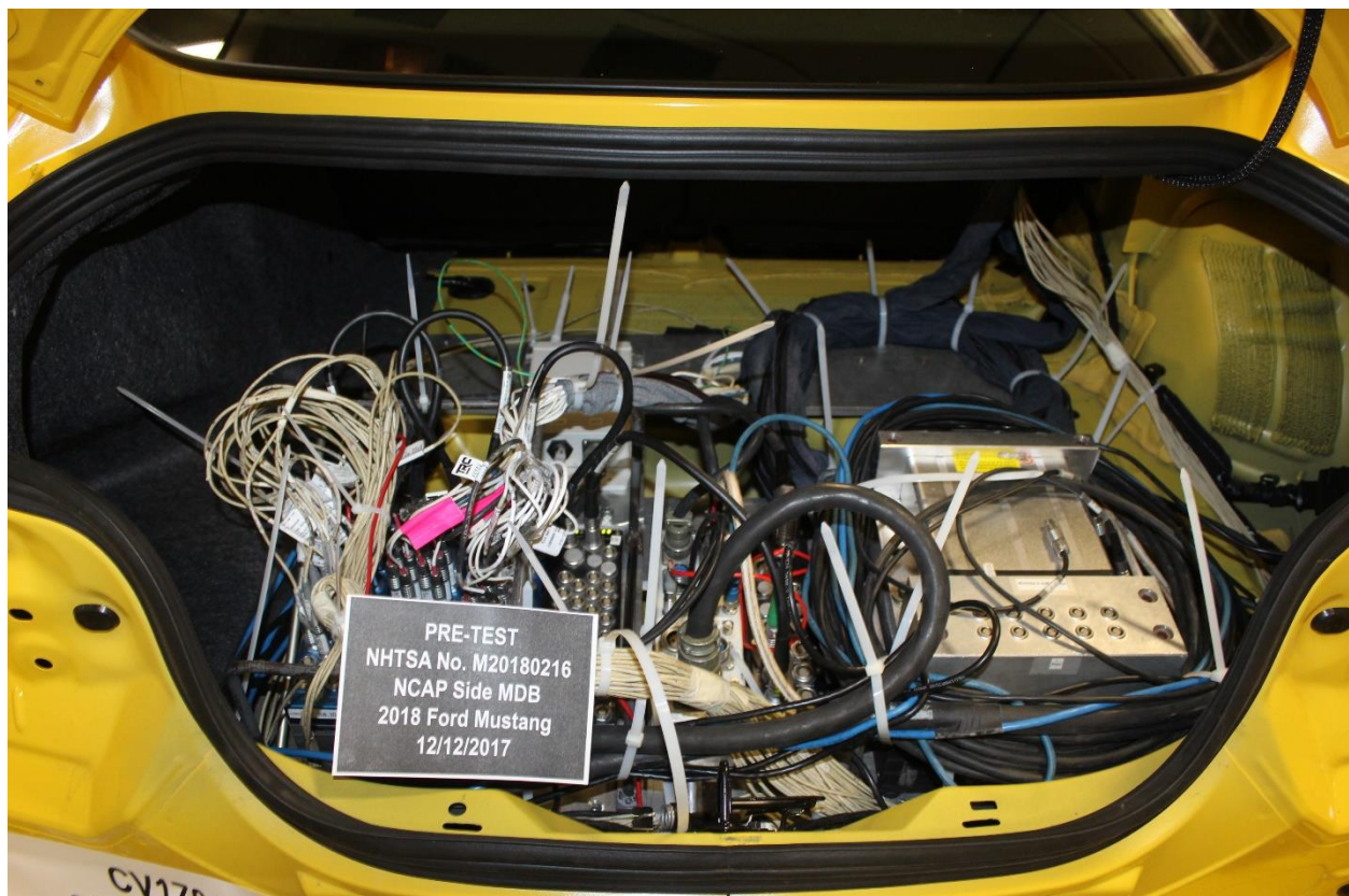
Figure A-94: Pre-Test Ballast View
