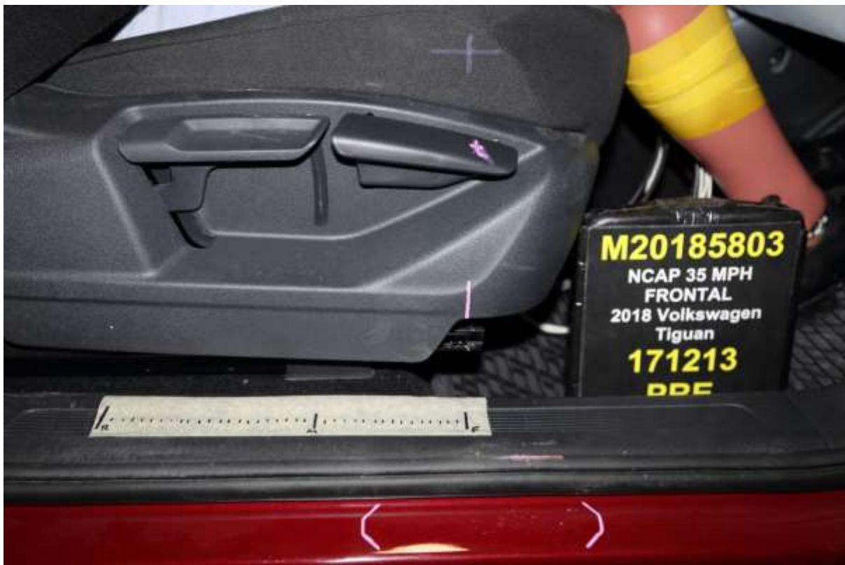
057 Pre-Test Passenger's Seat Fore-Aft Markings
