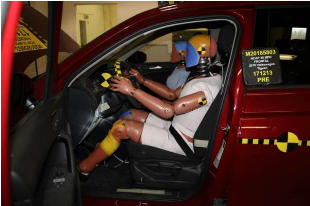
034 Pre-Test Driver Dummy and Vehicle Interior View
