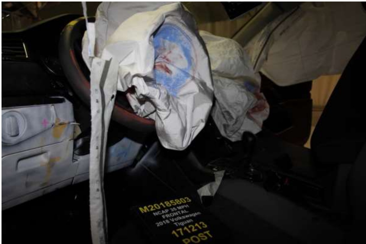
047 Post-Test Driver Dummy Contact With Airbag
