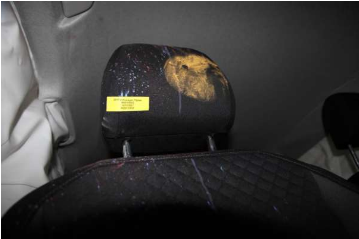
069 Post Test Passenger Dummy Contact With Headrest
