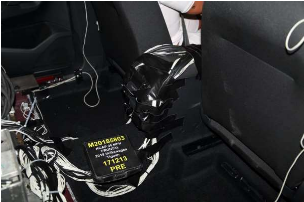
028 Pre-Test Dummy Cable Routing
