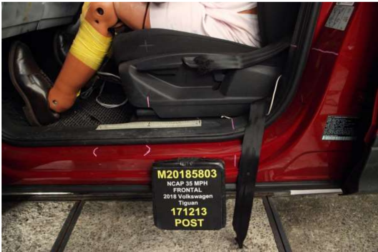
037 Post-Test Driver's Seat Fore-Aft Markings
