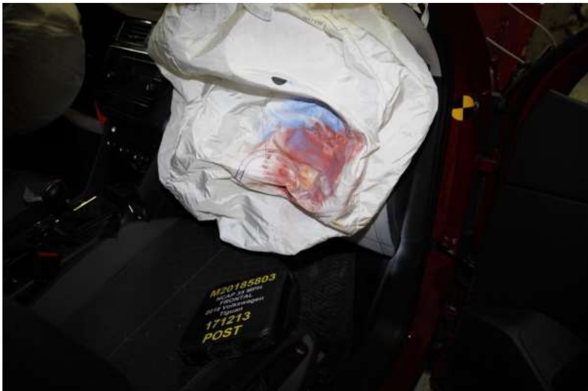
068 Post-Test Passenger Dummy Contact With Airbag
