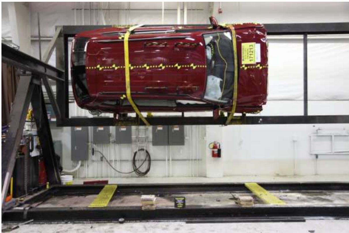
074 Vehicle at 90° on Static Rollover Device
