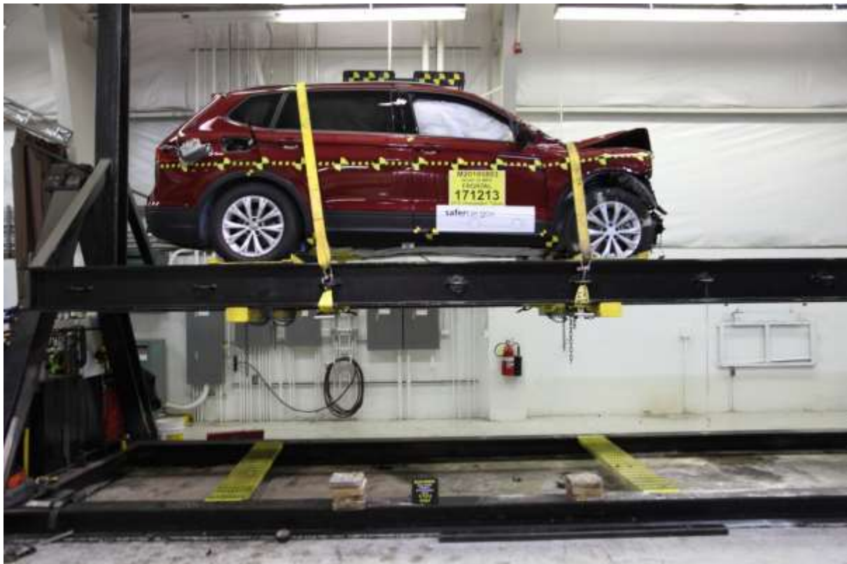
073 Vehicle at 0° on Static Rollover Device
