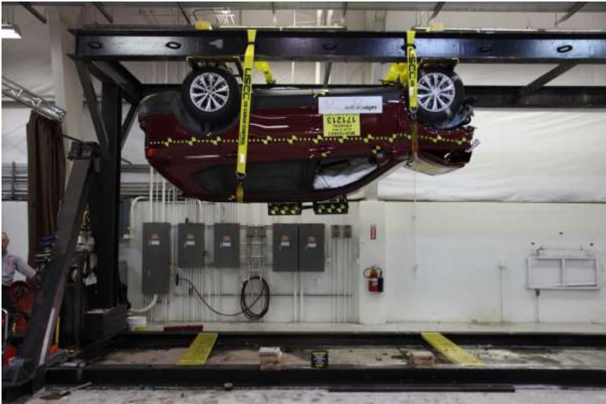
075 Vehicle at 180° on Static Rollover Device
