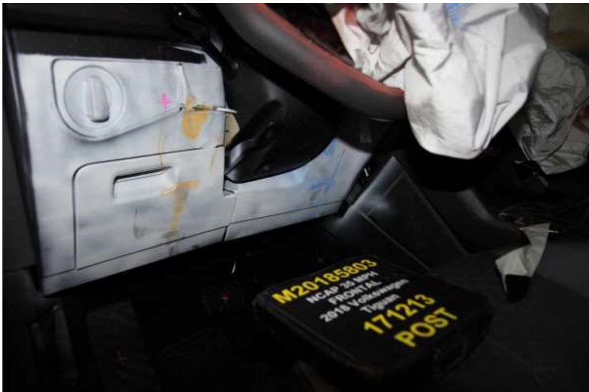
043 Post-Test Driver's Side Knee Bolster
