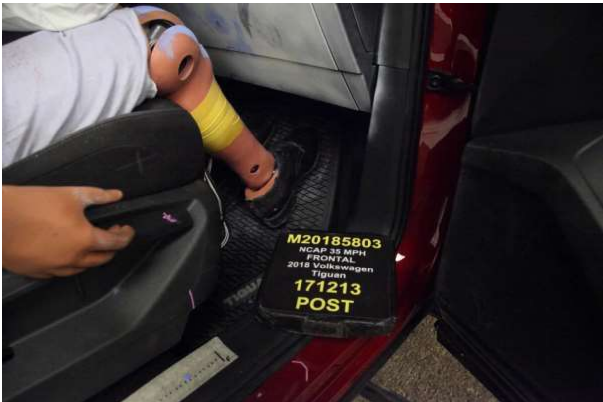
062 Post-Test Passenger Dummy Feet
