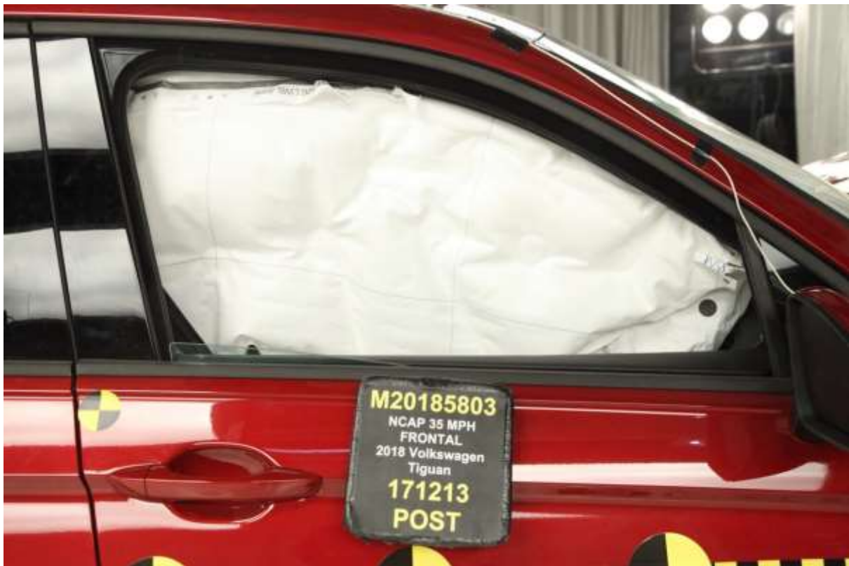
054 Post-Test Passenger Dummy Window View
