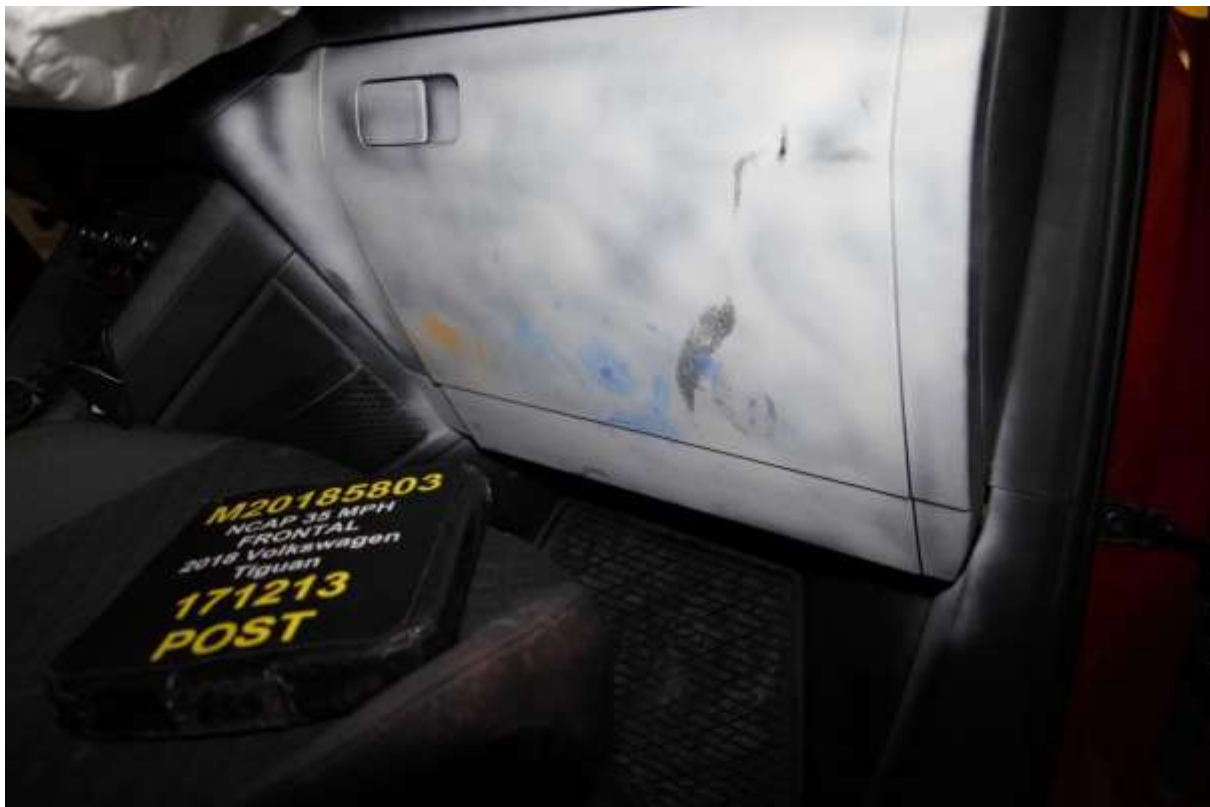
064 Post-Test Passenger's Side Knee Bolster
