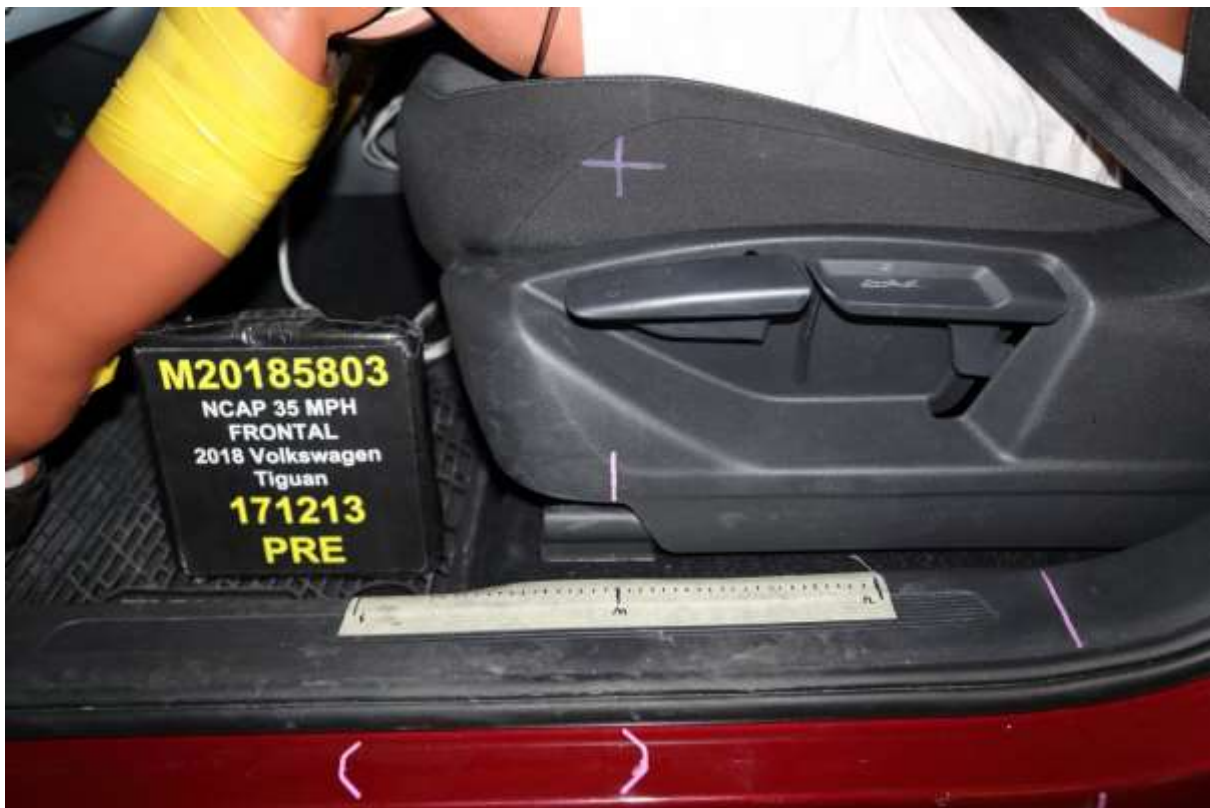
036 Pre-Test Driver's Seat Fore-Aft Markings
