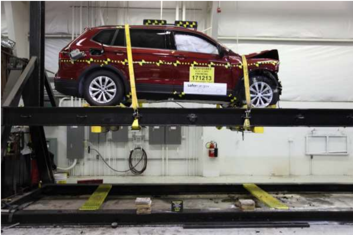
077 Vehicle at 360° on Static Rollover Device
