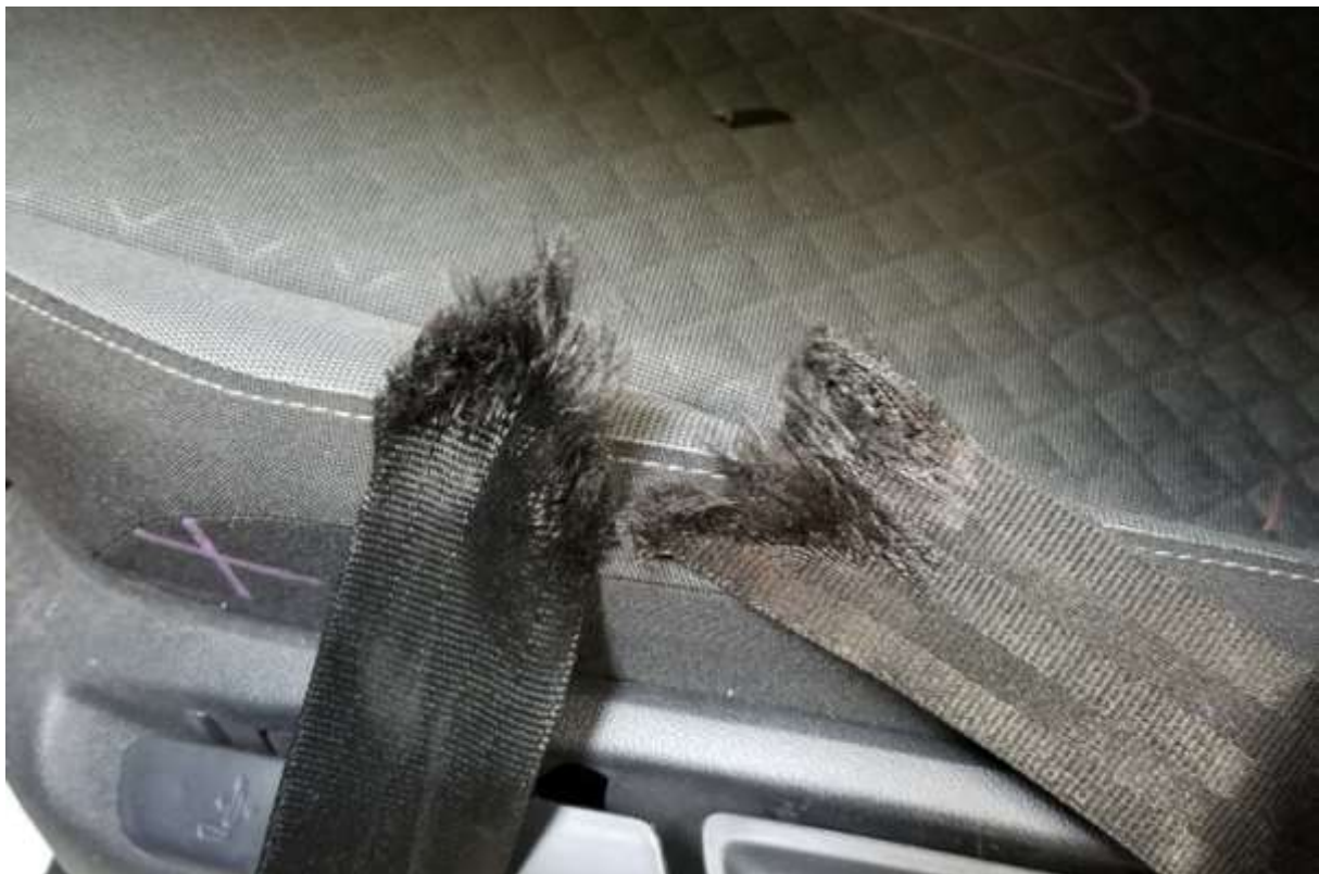
080 Post-Test Driver Seat Belt Separation
