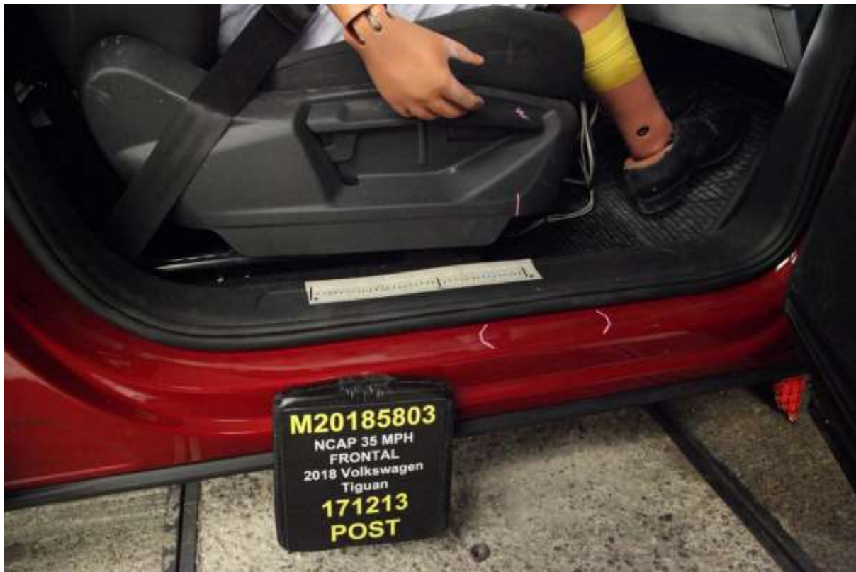
058 Post-Test Passenger's Seat Fore-Aft Markings
