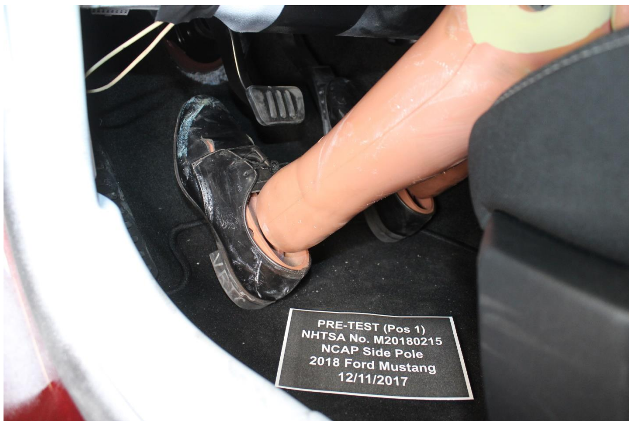
Figure A-32: Pre-Test Placement of Dummy's Feet
