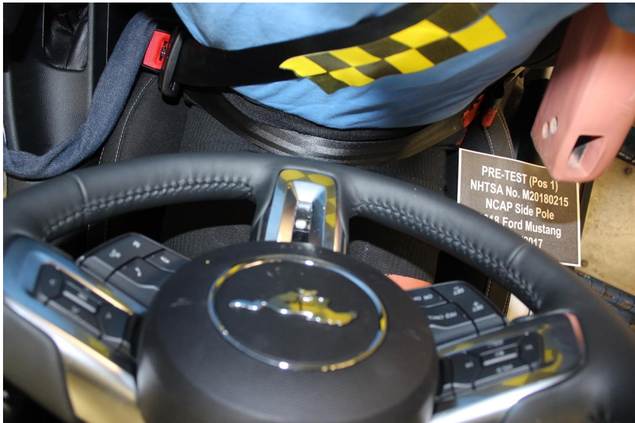
Figure A-29: Pre-Test Overhead View of Dummy Thighs on Seat Pan
