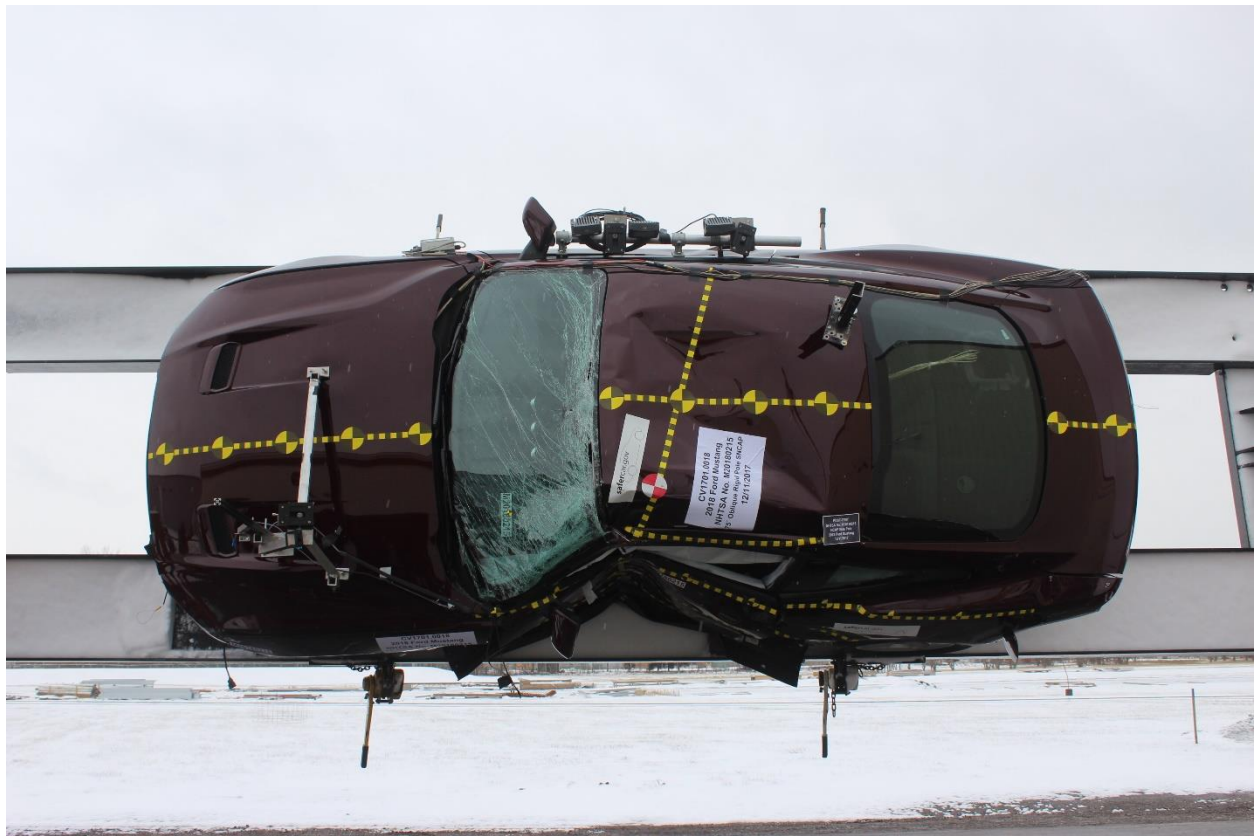
Figure A-64: FMVSS No. 301 Static Rollover 90 Degrees
