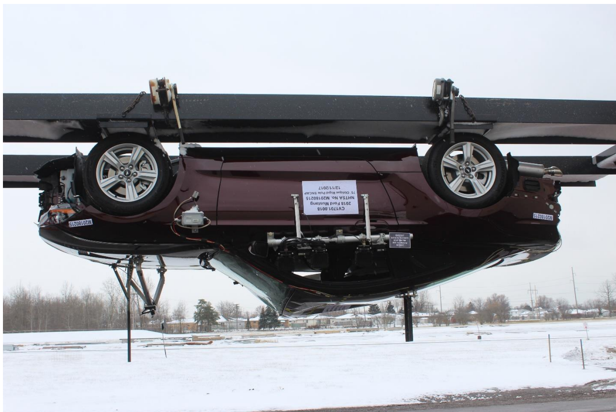
Figure A-65: FMVSS No. 301 Static Rollover 180 Degrees
