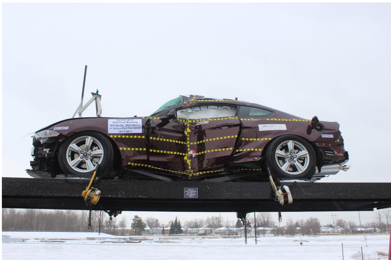
Figure A-67: FMVSS No. 301 Static Rollover 360 Degrees
