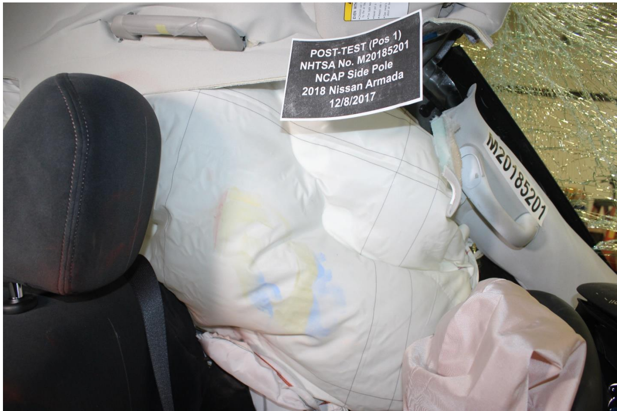
Figure A-47: Post-Test Dummy Close-Up Head Contact with Side Airbag View
