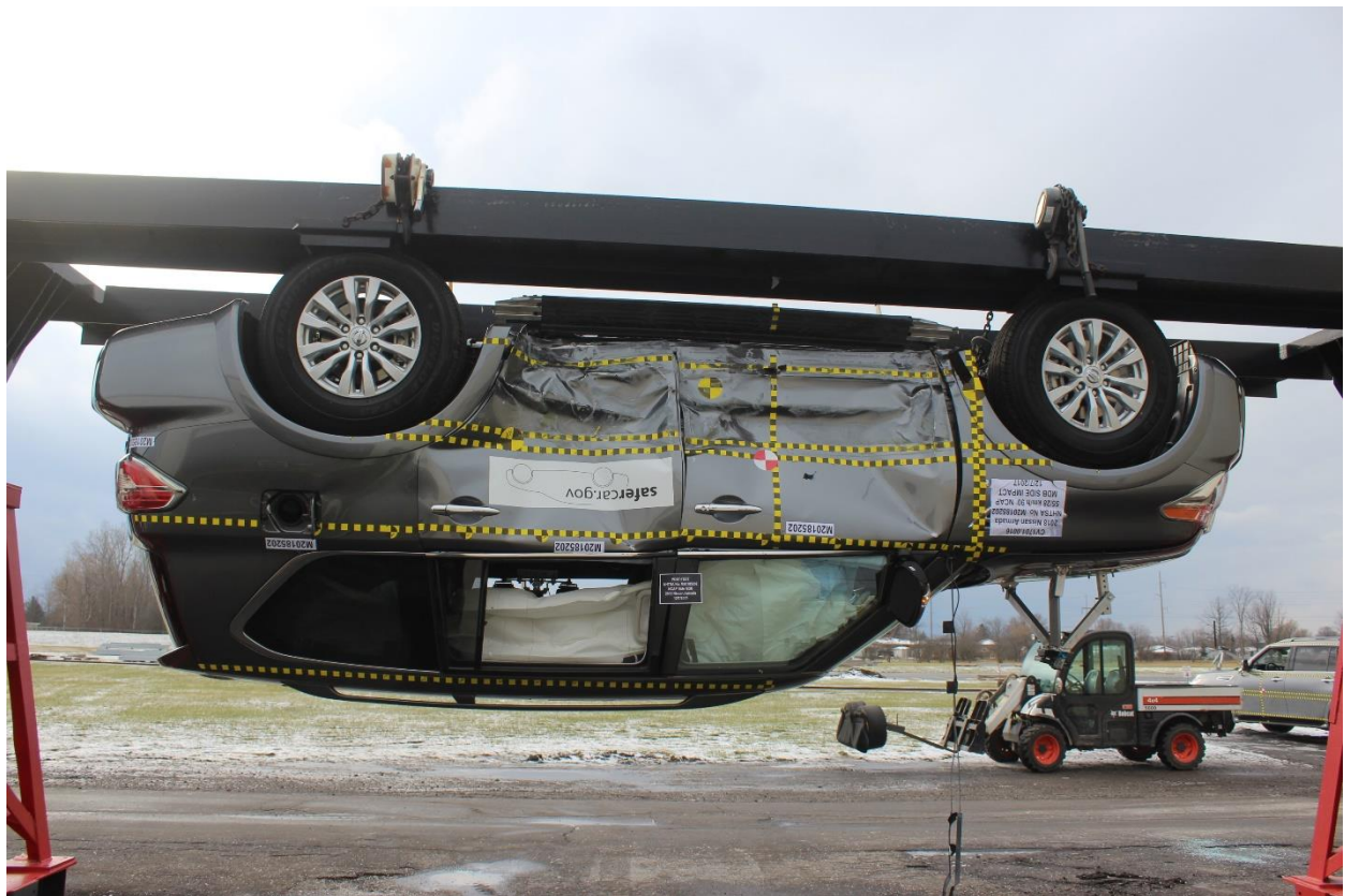
Figure A-98: FMVSS No. 301 Static Rollover 180 Degrees
