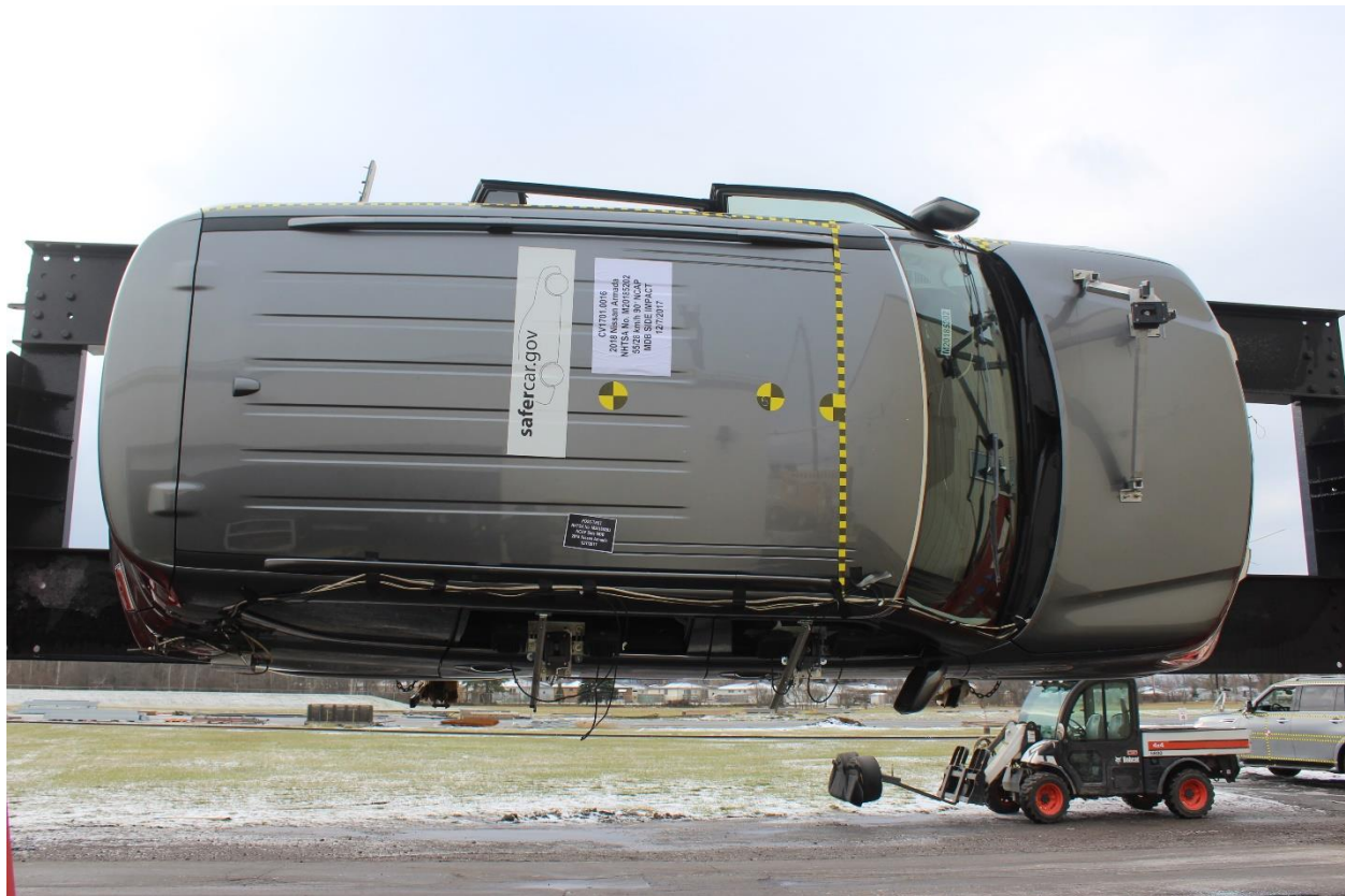
Figure A-99: FMVSS No. 301 Static Rollover 270 Degrees
