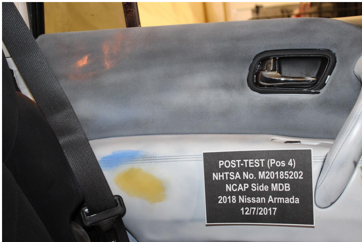
Figure A-77: Post-Test Rear Passenger Dummy Close-Up Torso Contact with Vehicle Interior View
