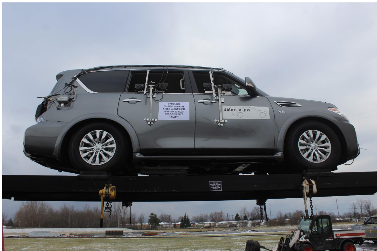
Figure A-96: FMVSS No. 301 Static Rollover 0 Degrees
