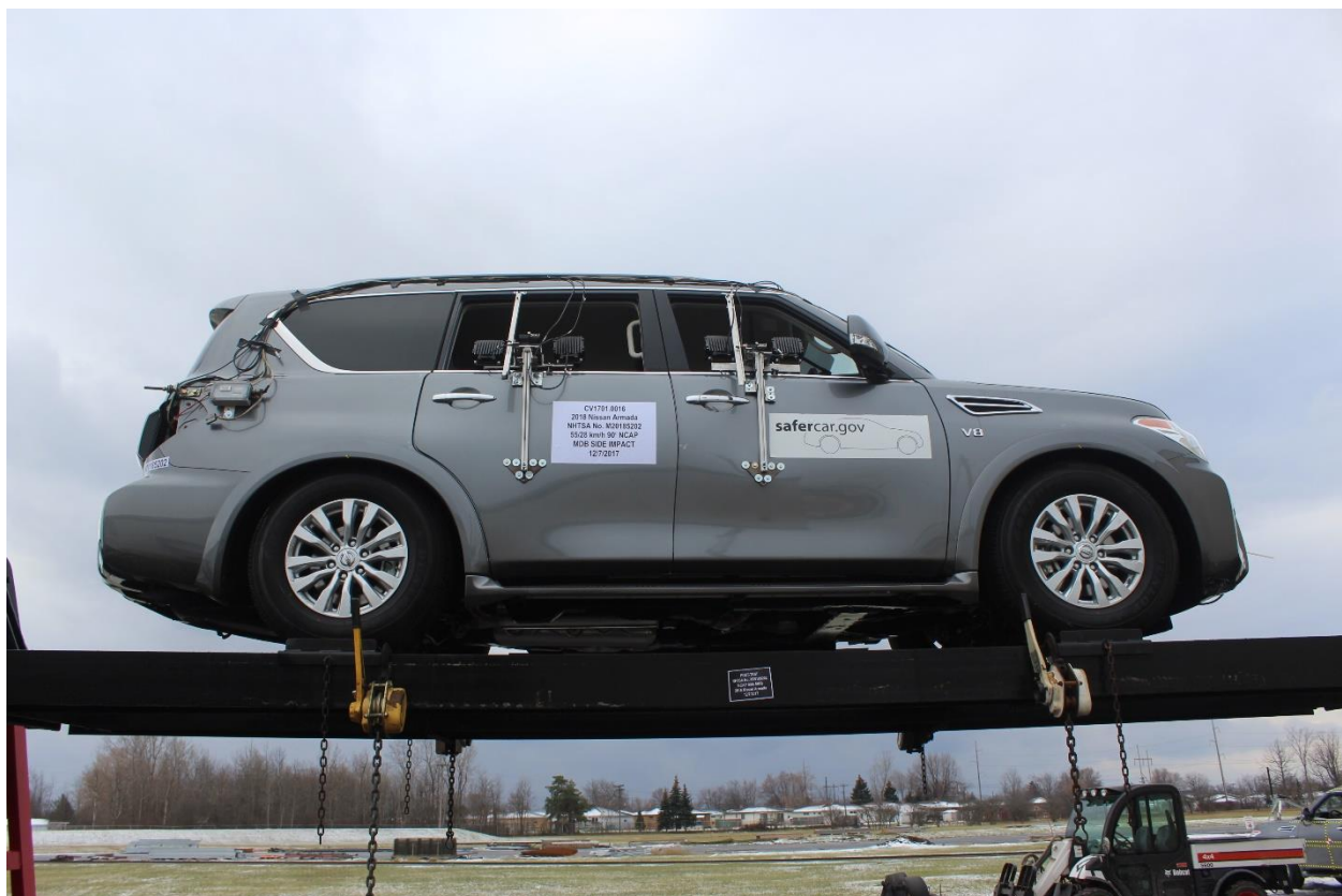
Figure A-100: FMVSS No. 301 Static Rollover 360 Degrees
