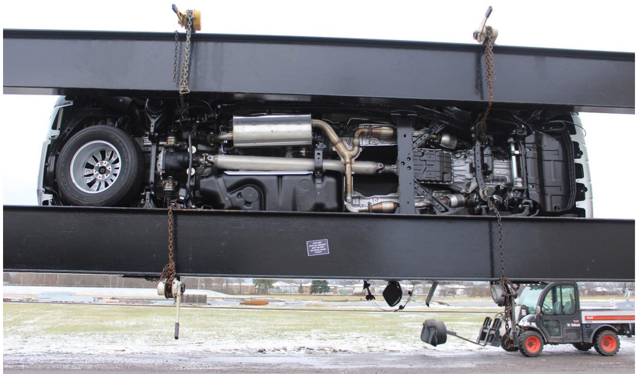
Figure A-97: FMVSS No. 301 Static Rollover 90 Degrees
