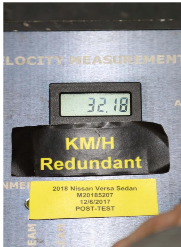
No. 062 Post-Test Primary and Redundant Speed Trap Read Out
