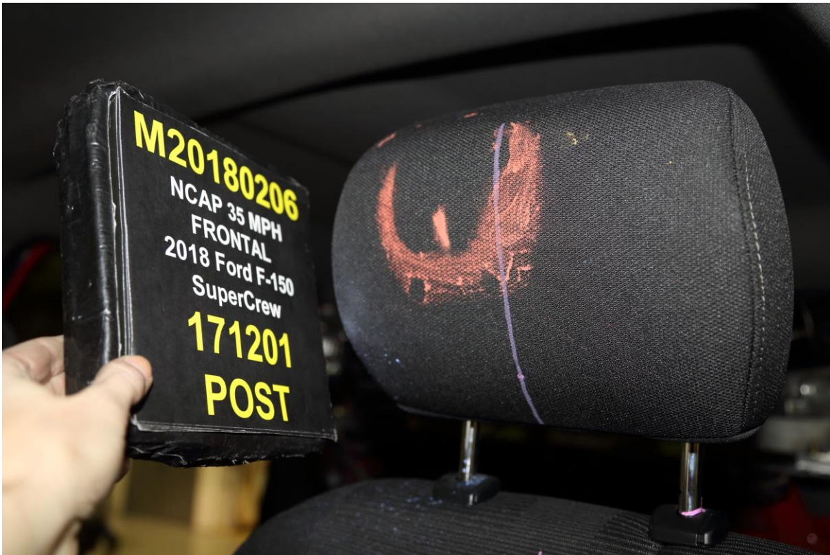
048 Post-Test Driver Dummy Contact With Headrest
