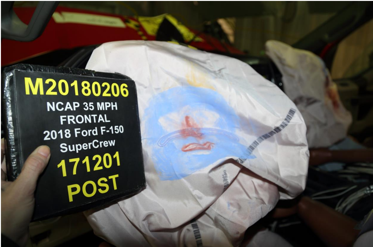
047 Post-Test Driver Dummy Contact With Airbag
