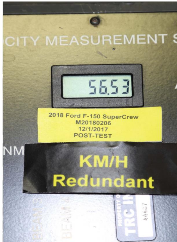
072 Post-Test Speed Trap Readout
