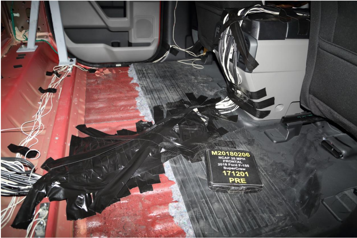
028 Pre-Test Dummy Cable Routing
