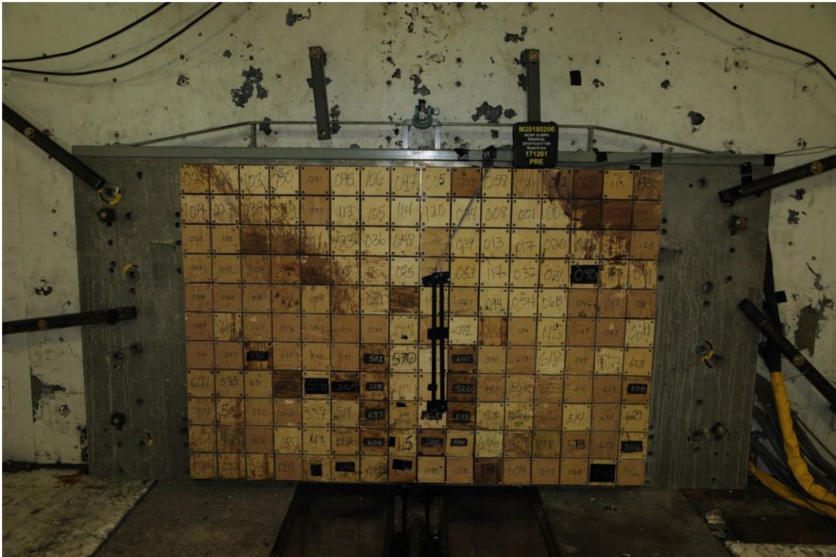
002 Pre-Test Load Cell Wall
