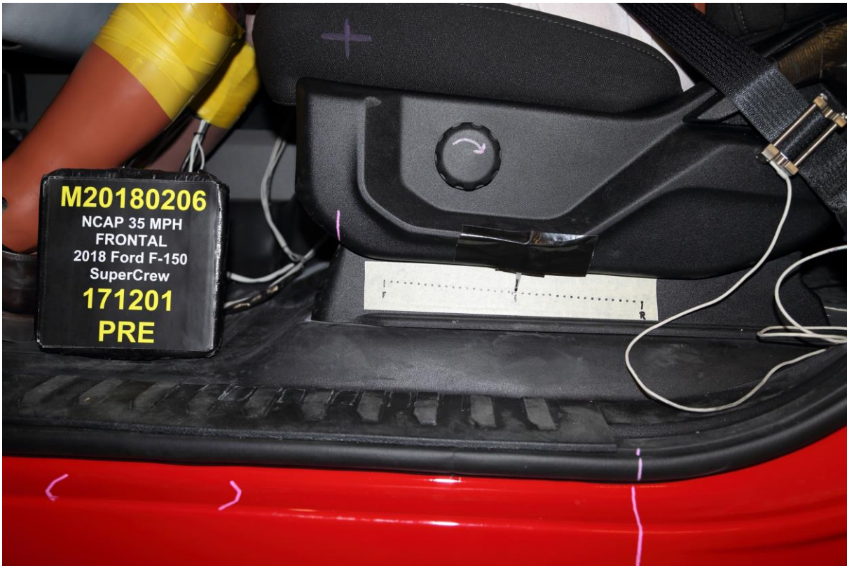
036 Pre-Test Driver's Seat Fore-Aft Markings
