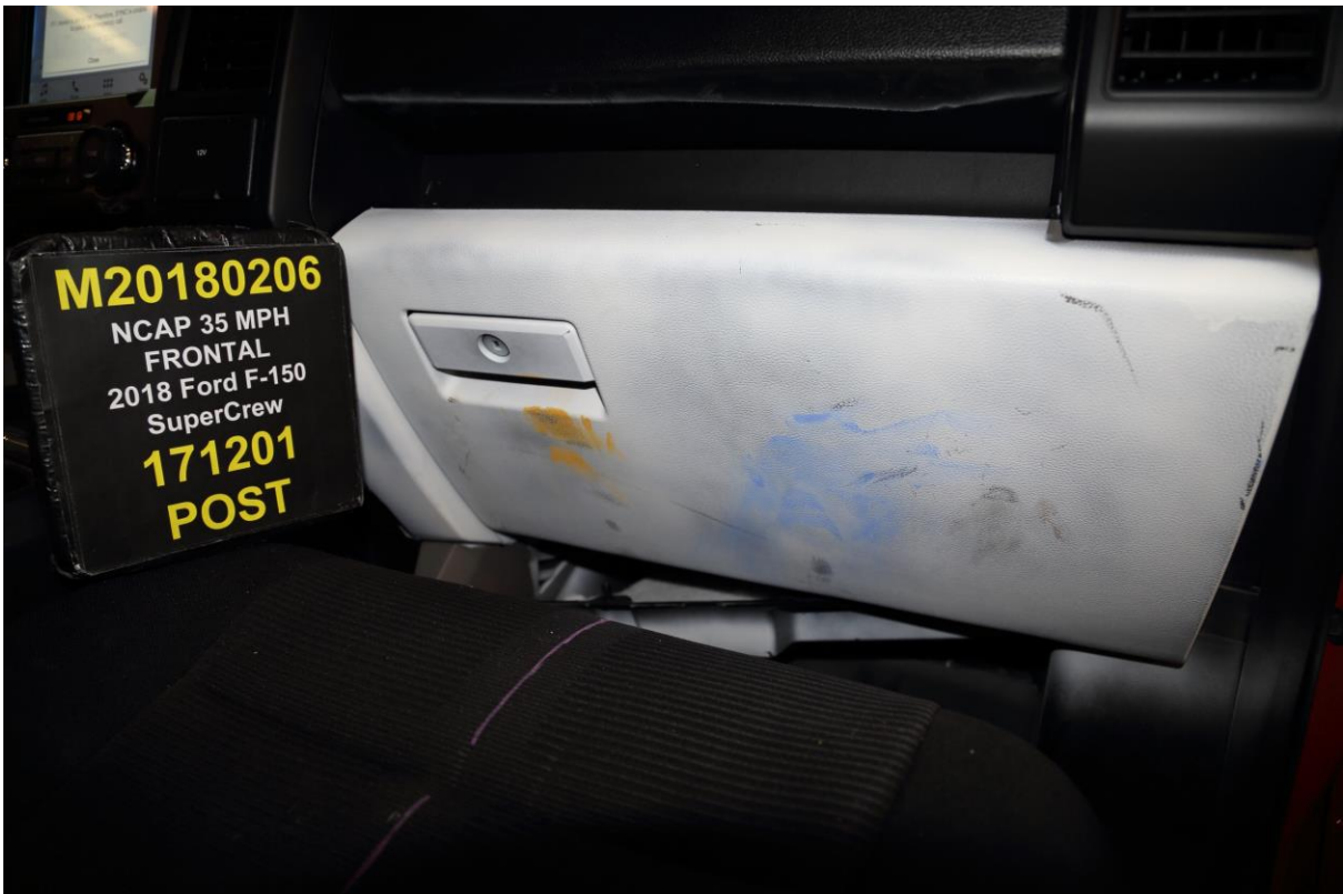
064 Post-Test Passenger's Side Knee Bolster
