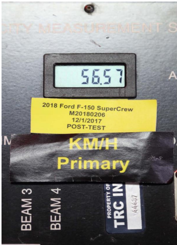
072 Post-Test Speed Trap Readout
