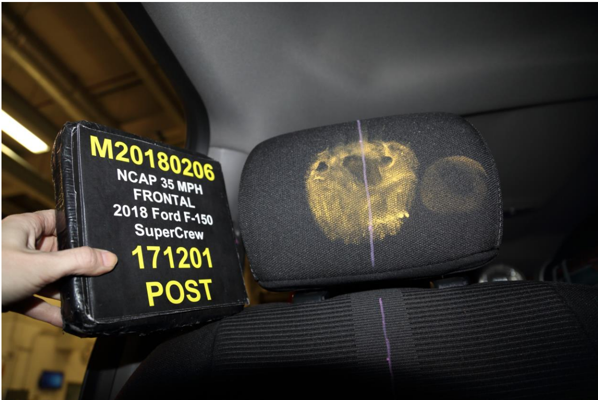
069 Post Test Passenger Dummy Contact With Headrest
