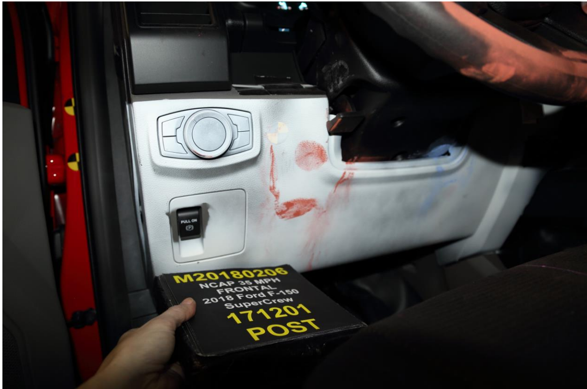
043 Post-Test Driver's Side Knee Bolster
