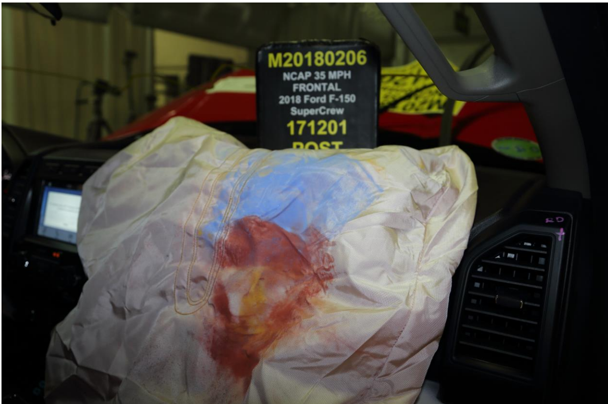
068 Post-Test Passenger Dummy Contact With Airbag
