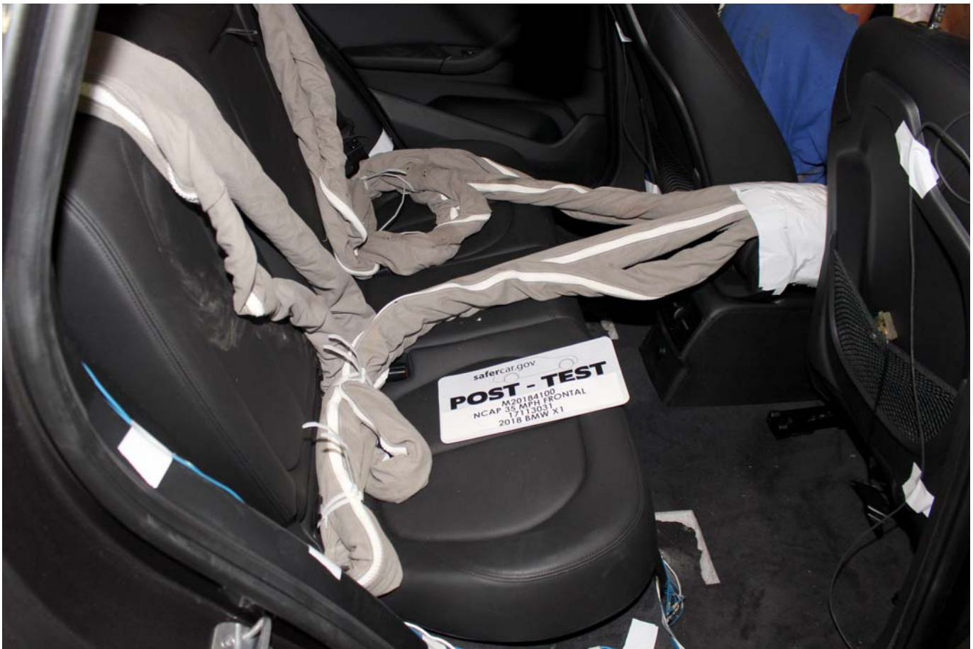
Photo No. 029 - Post-Test Dummy Cable Routing
