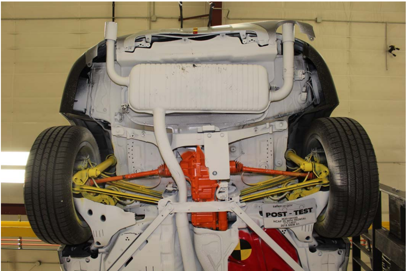
Photo No. 027 - Post-Test Rear Underbody View
