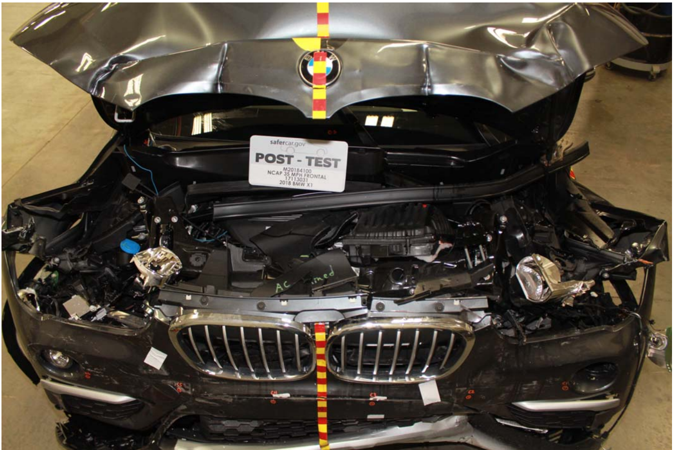
Photo No. 021 - Post-Test Engine Compartment View
