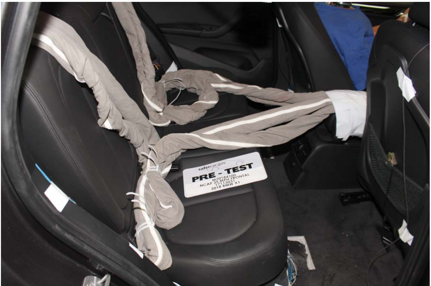
Photo No. 028 - Pre-Test Dummy Cable Routing
