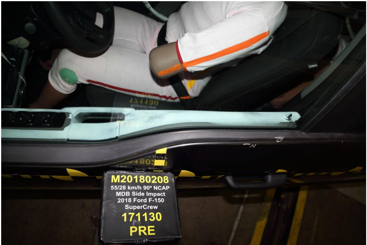
042 Pre-Test Driver Dummy and Door Clearance View
