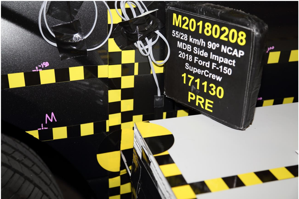
019 Pre-Test Close-Up View of Impact Point Target
