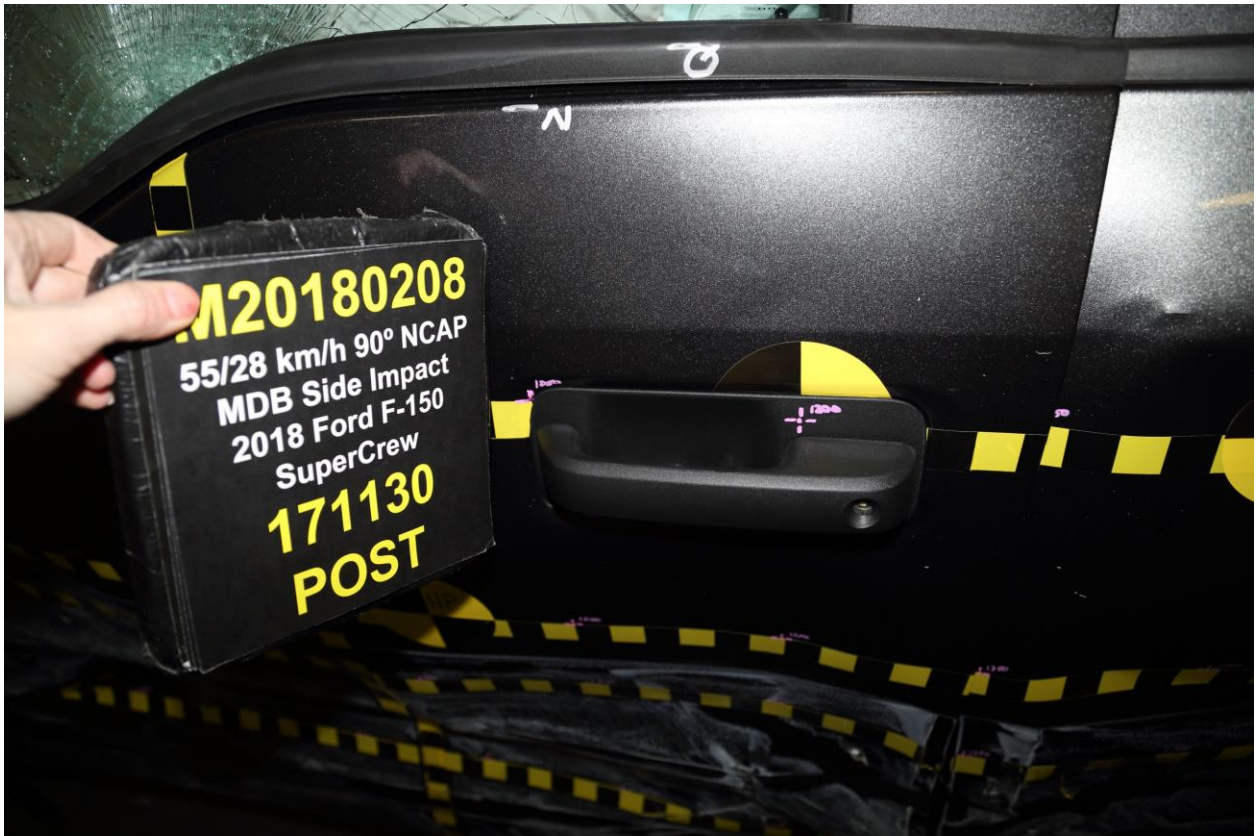
022 Post-Test Left Front Door Latch Close-Up
