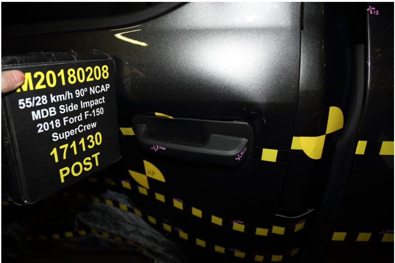
024 Post-Test Left Rear Door Latch Close-Up
