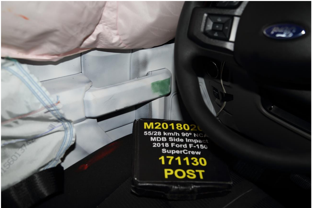
054 Post-Test Driver Dummy Close-Up Knee Contact View
