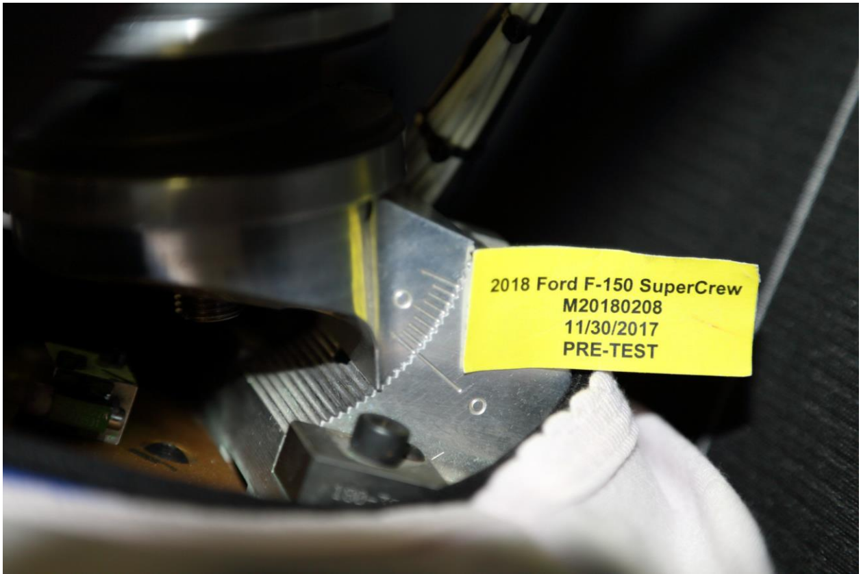
062 Pre-Test View of Rear Passenger Dummy's Neck Showing Position of Adjustable Neck Bracket
