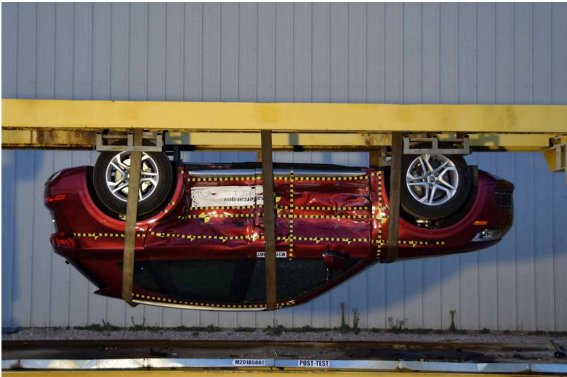
FIGURE 98. FMVSS No. 301 Static Rollover 180 Degrees
