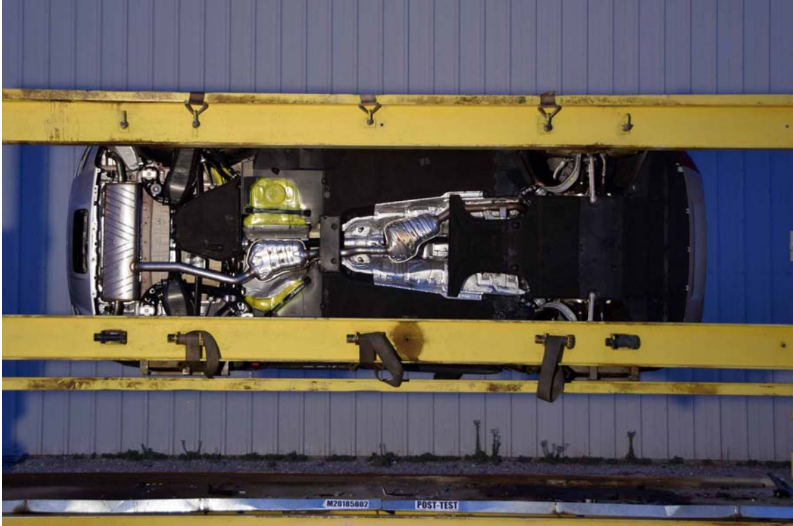
FIGURE 99. FMVSS No. 301 Static Rollover 270 Degrees
