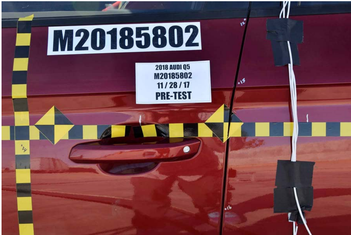
FIGURE 21. Pre-Test Left Front Door Latch Close-Up
