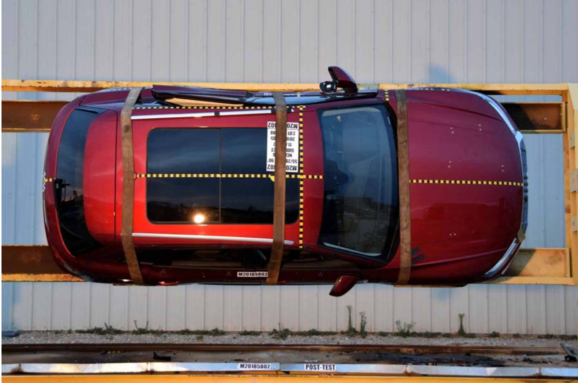
FIGURE 97. FMVSS No. 301 Static Rollover 90 Degrees
