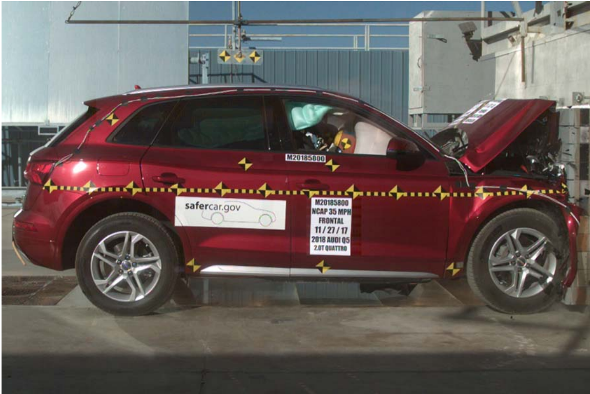
FIGURE 78. 2018 Audi Q5 2.0T Quattro Frontal Impact Event
