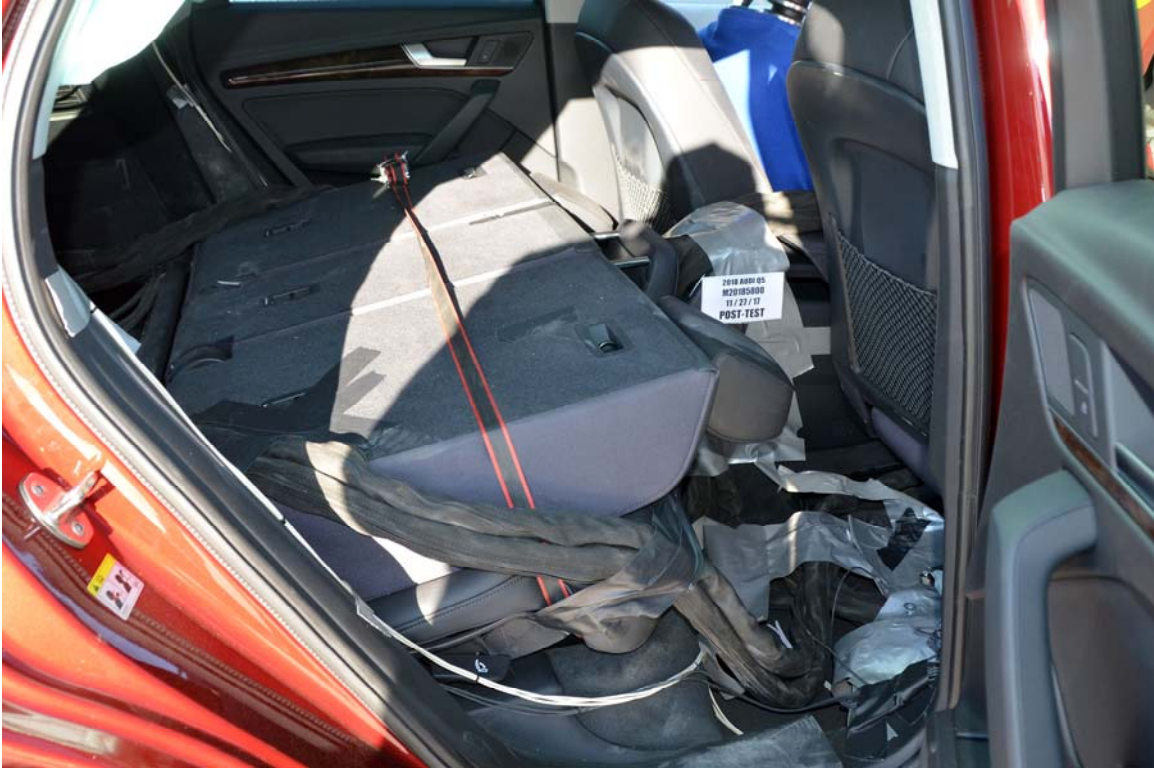
FIGURE 29. Post-Test Dummy Cable Routing
