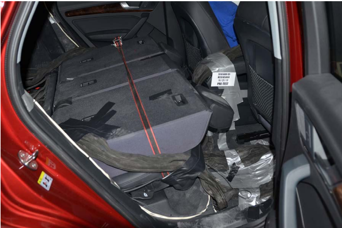
FIGURE 28. Pre-Test Dummy Cable Routing
