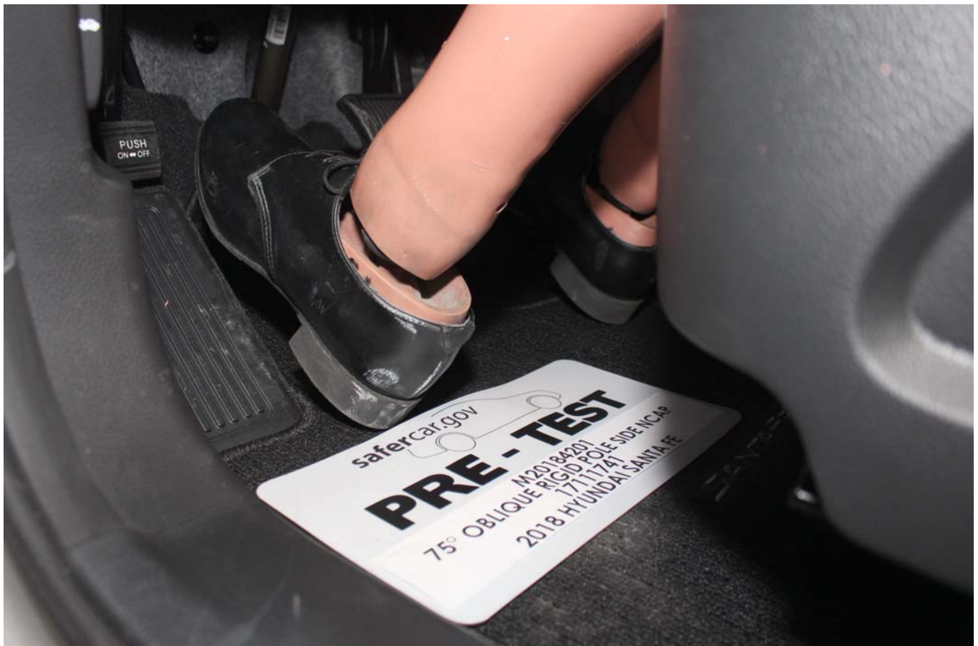
Photo No. 032 - Pre-Test Placement of Dummy Feet
