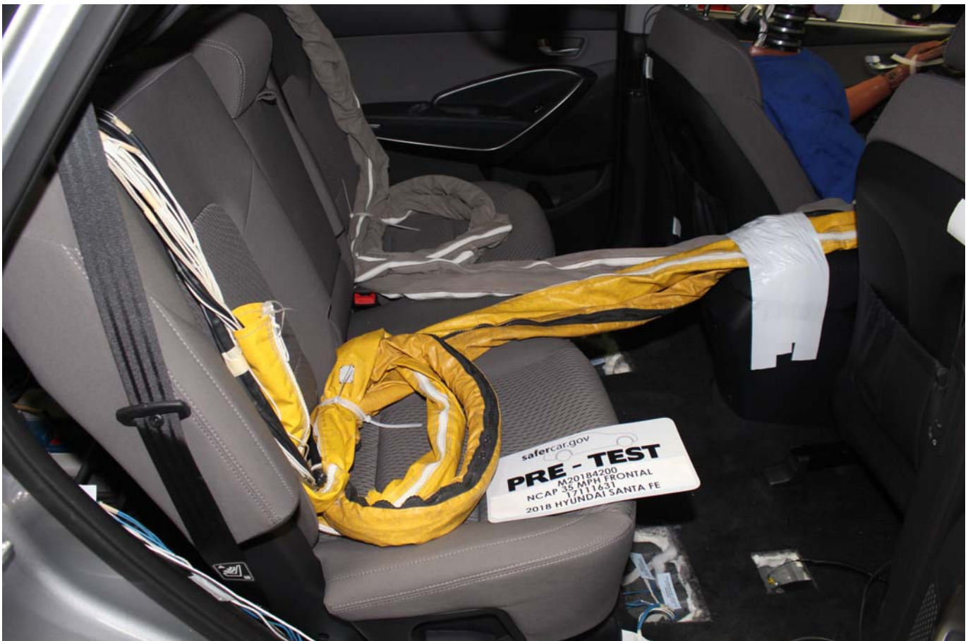
Photo No. 028 - Pre-Test Dummy Cable Routing
