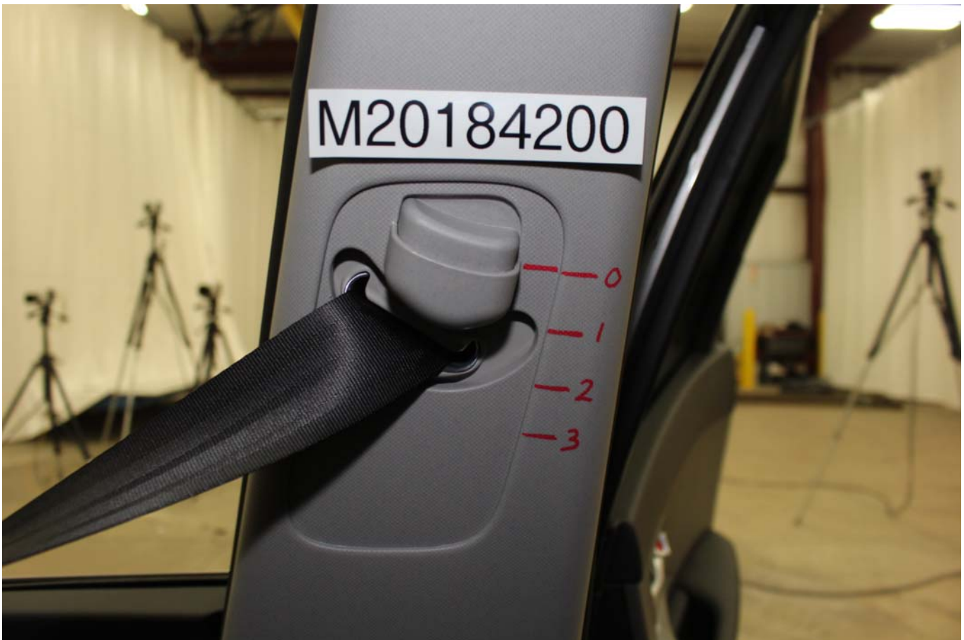
Photo No. 060 - Post-Test View of Belt Anchorage for Passenger Dummy
