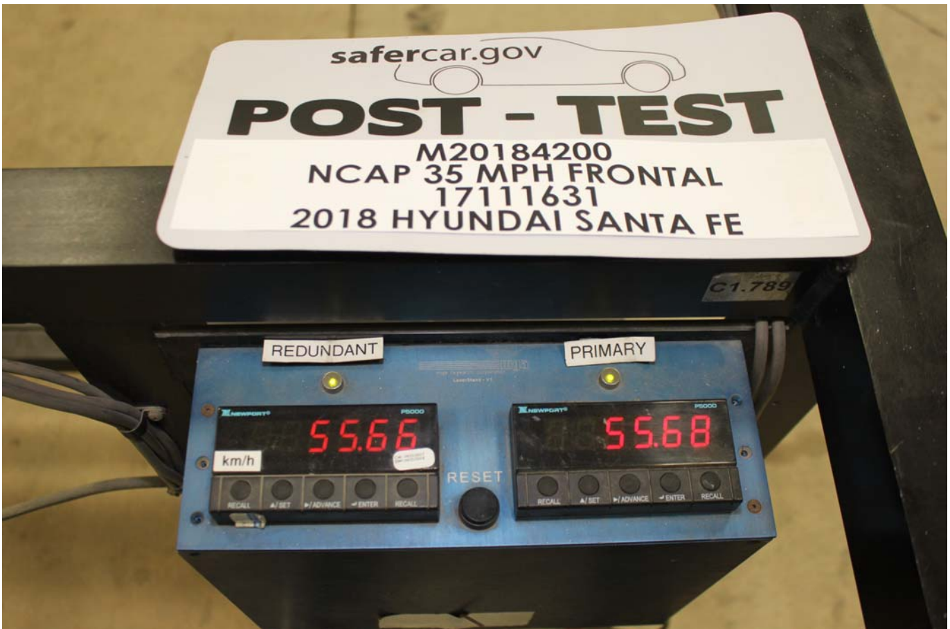
Photo No. 072 - Post-Test Speed Trap Read-Out
