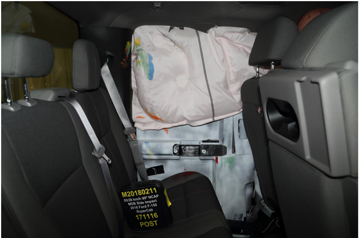
074 Post-Test Rear Passenger Inner Door Panel View
