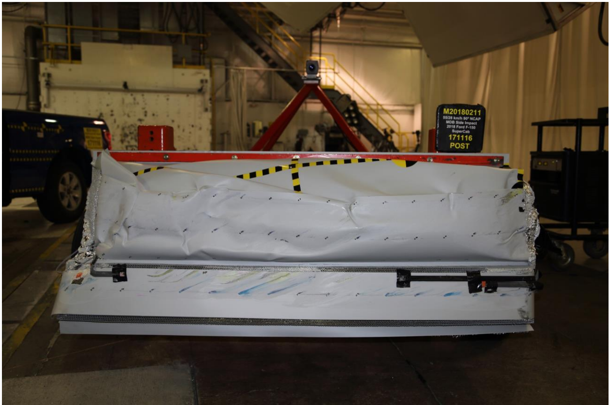
085 Post-Test Front View of MDB Impactor Face
