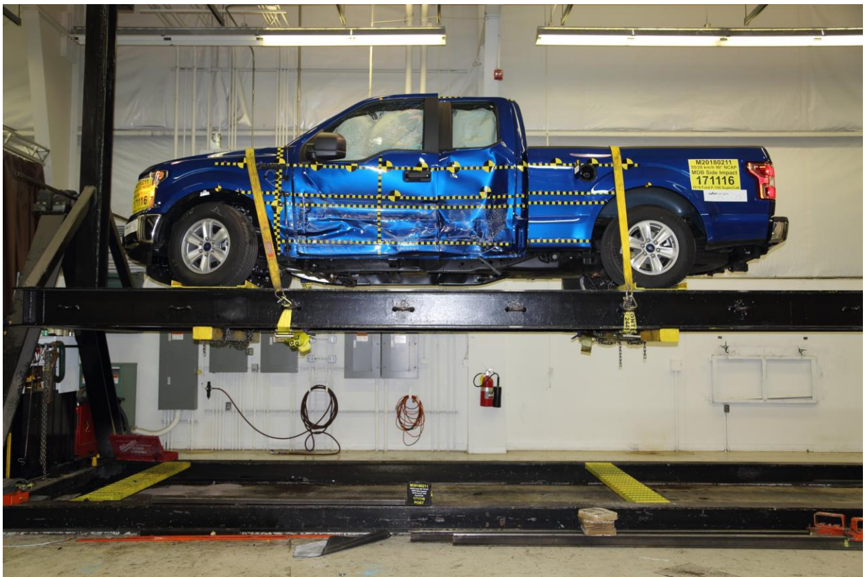
096 FMVSS No. 301 Static Rollover 0 Degrees
