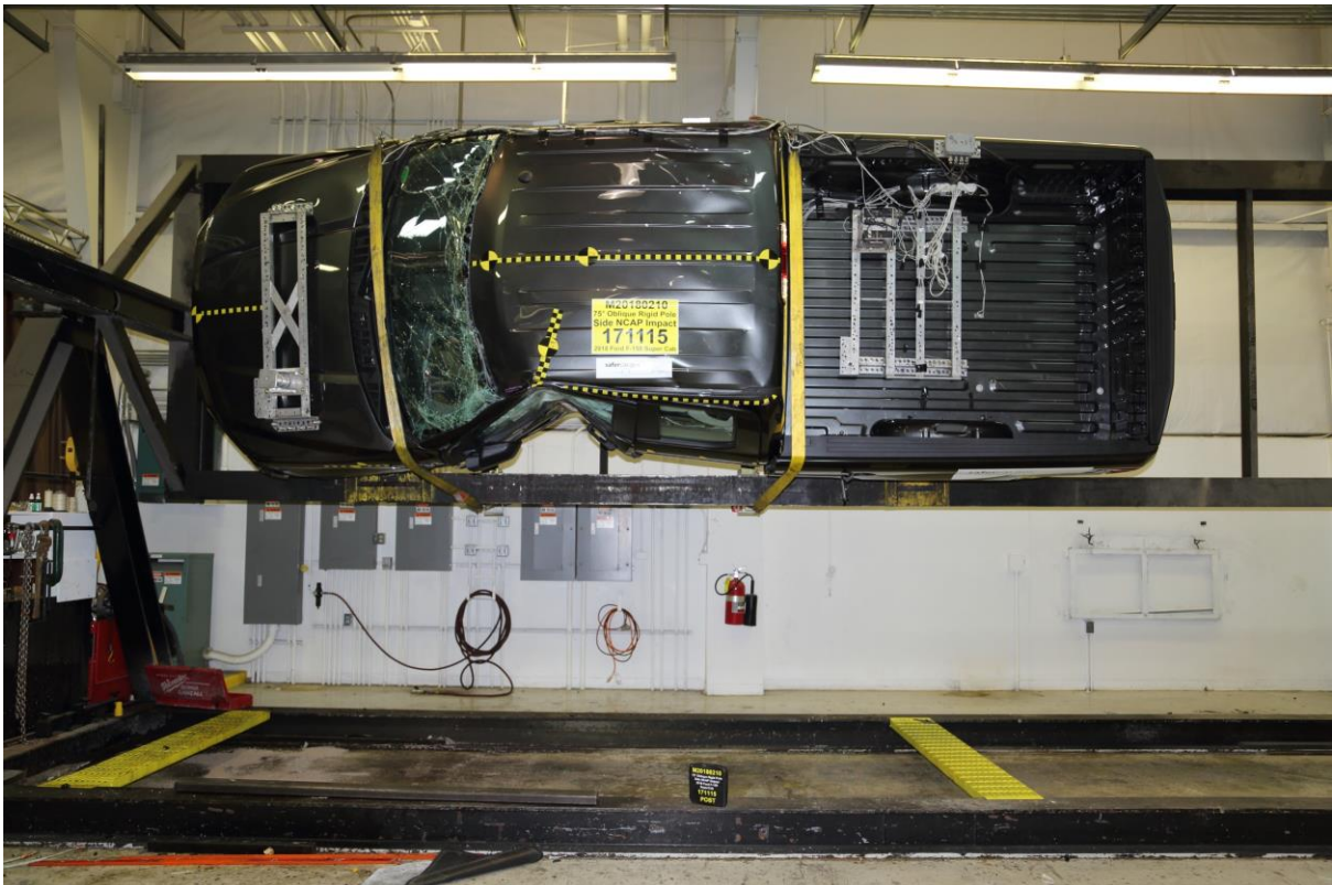
No. 064 FMVSS No. 301 Static Rollover 90 Degrees
