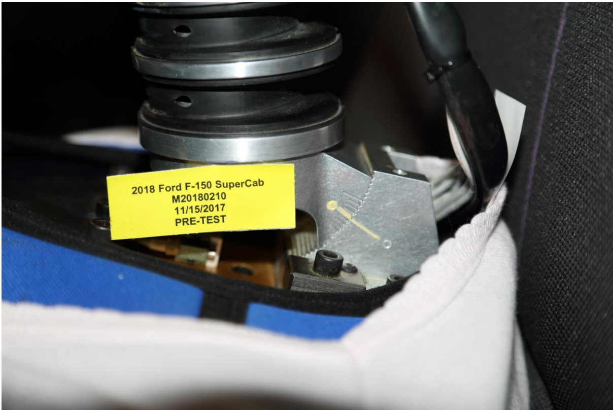
No. 030 Pre-Test Left Side View of Dummy Neck Showing Position of Adjustable Neck Bracket
