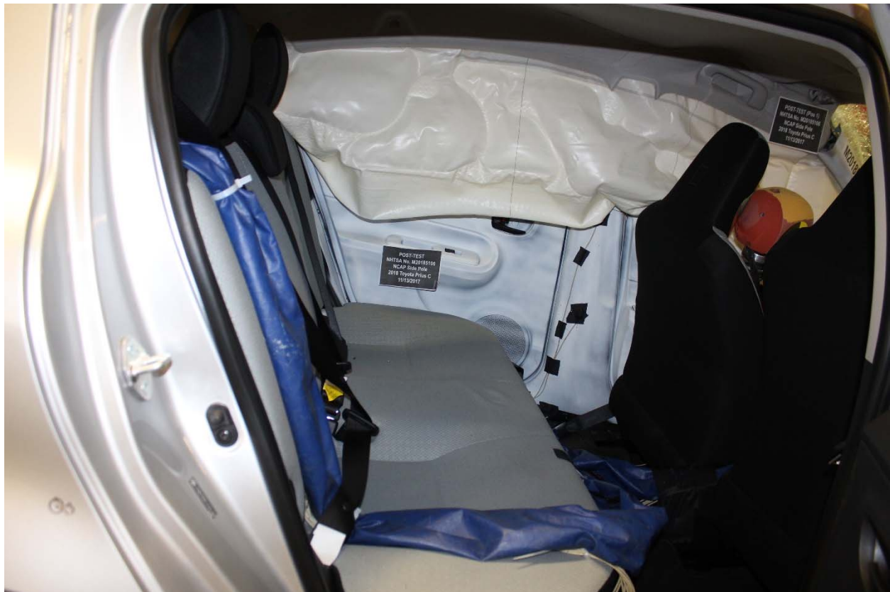
Figure A-33: Post-Impact View of the Vehicle Passenger Compartment Adjacent to Propulsion Battery
