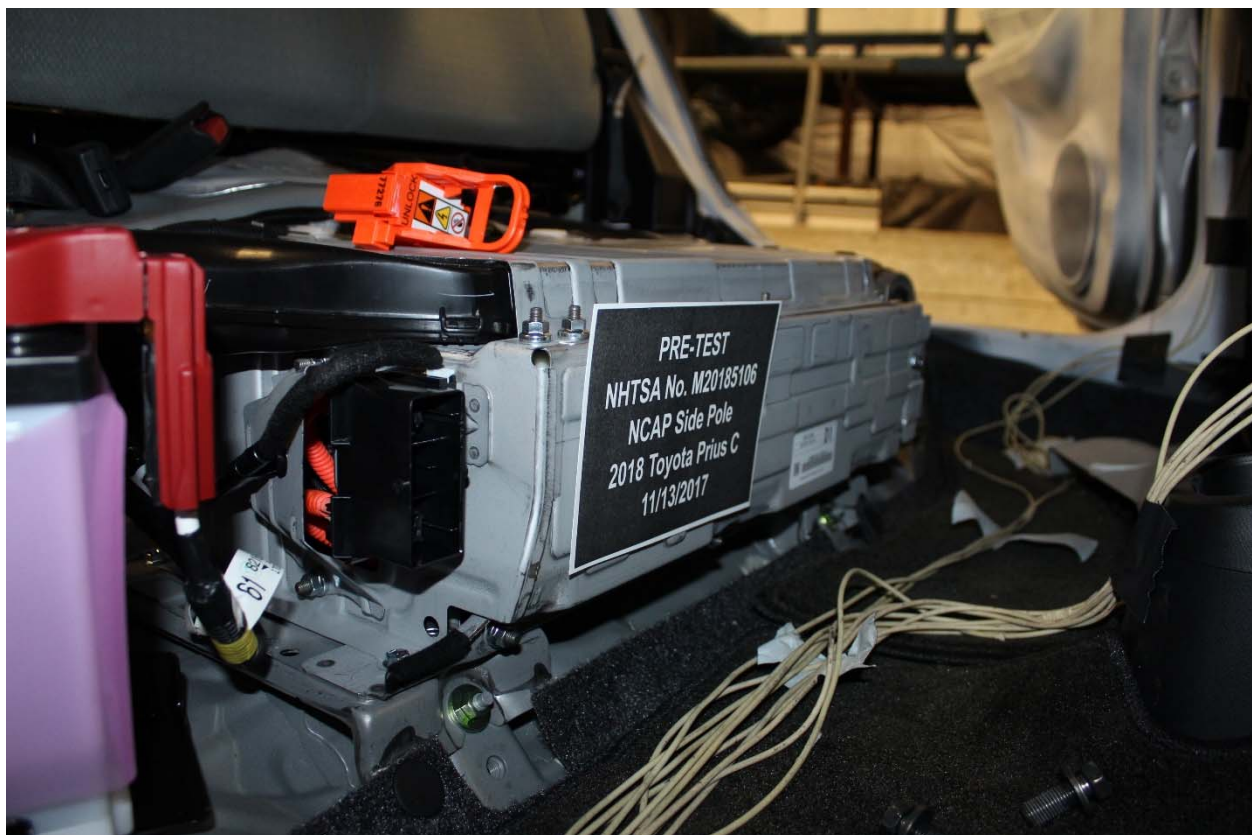
Figure A-8: Manual High Voltage Service Disconnect Removed Location
