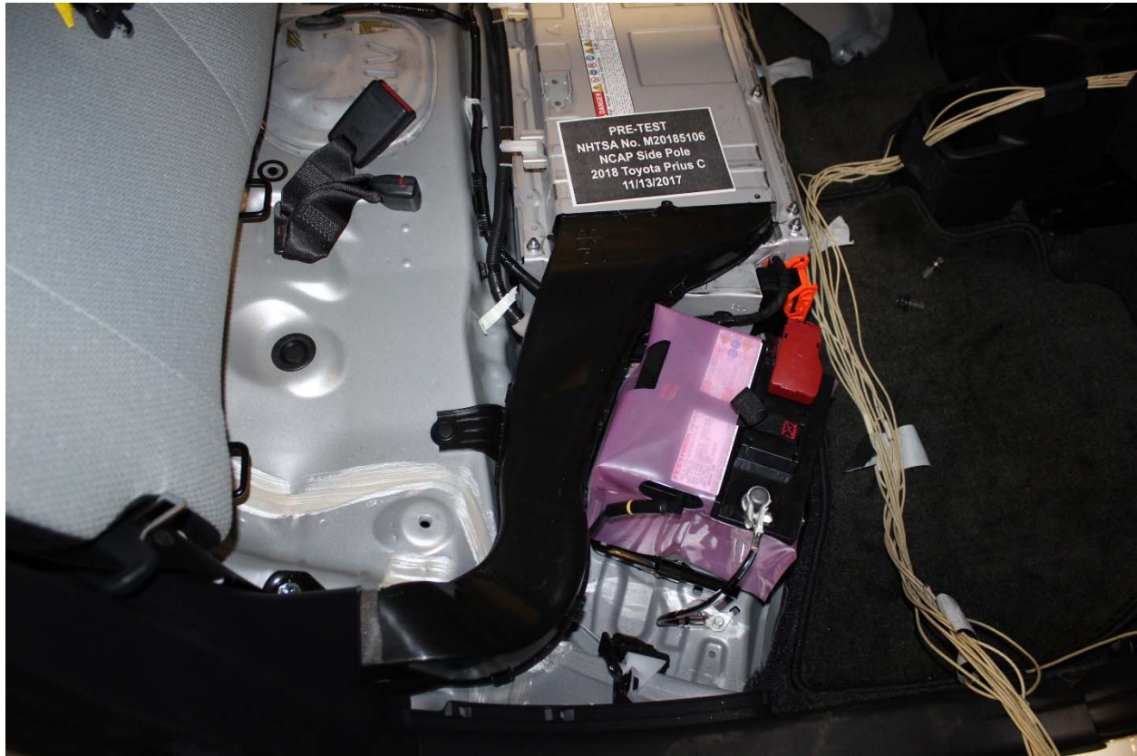
Figure A-19: Pre-Impact View Propulsion Battery Venting System(s)
