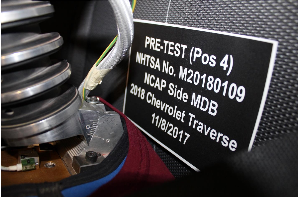
Figure A-62: Pre-Test View of Rear Passenger Dummy's Neck Showing Position of Adjustable Neck Bracket
