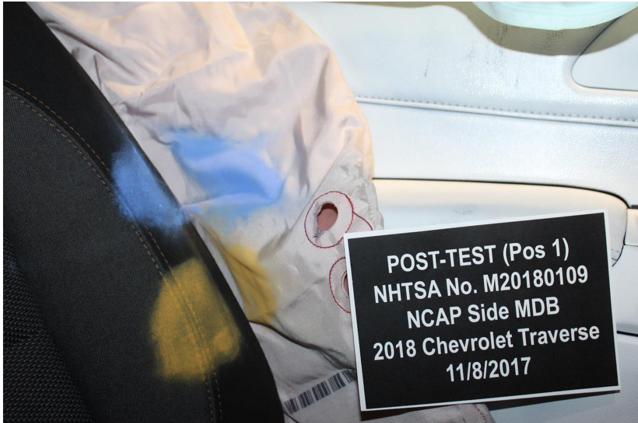
Figure A-51: Post-Test Driver Dummy Close-Up Torso Contact with Side Airbag View
