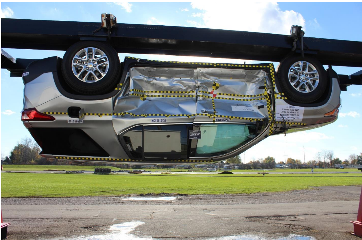
Figure A-98: FMVSS No. 301 Static Rollover 180 Degrees
