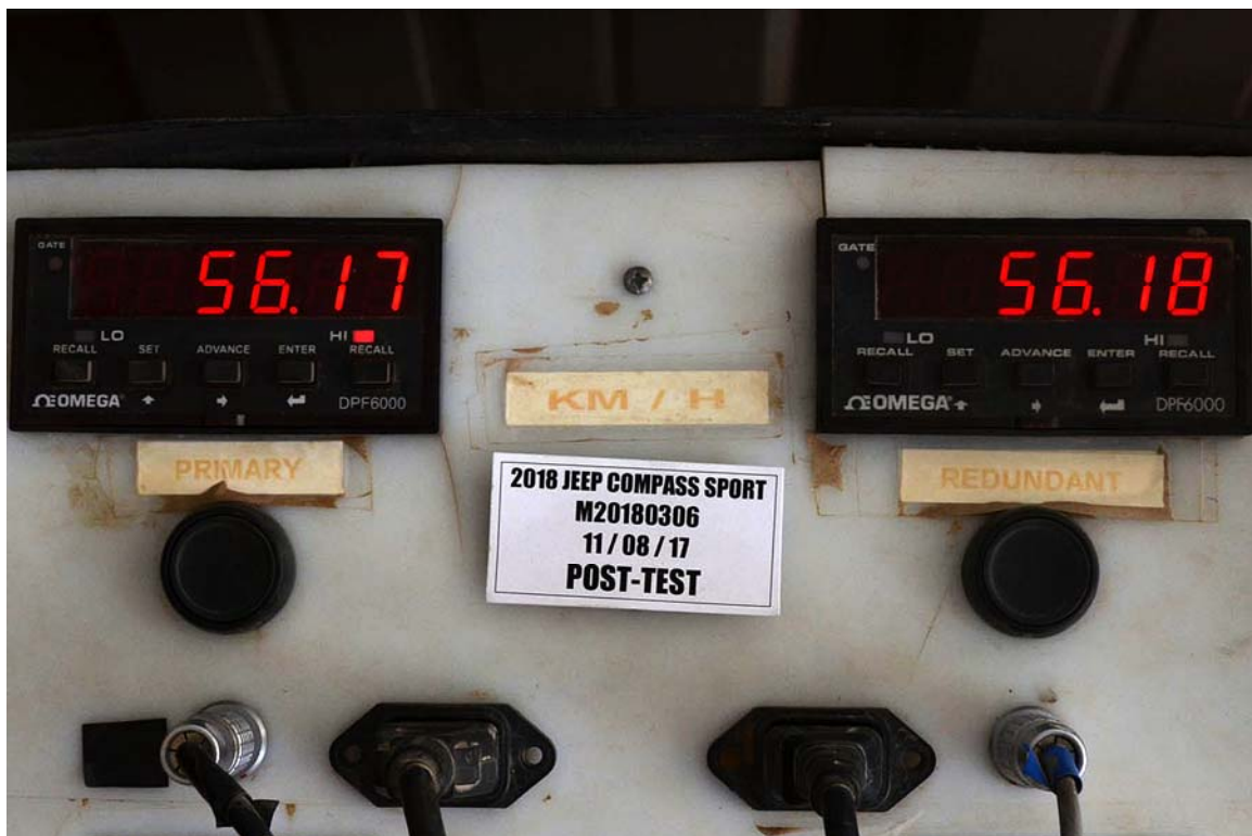
FIGURE 72. Post-Test Speed Trap Read-Out
