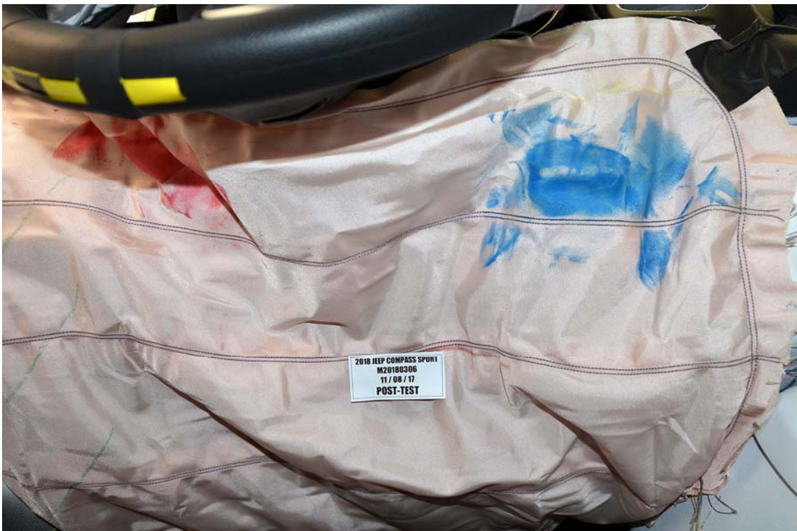
FIGURE 48b. Post-Test Driver Dummy Contact with Knee Airbag
