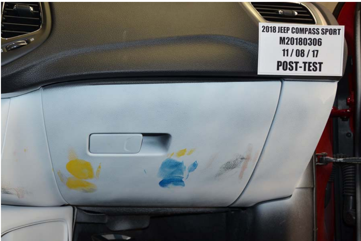
FIGURE 64. Post-Test Passenger's Side Knee Bolster
