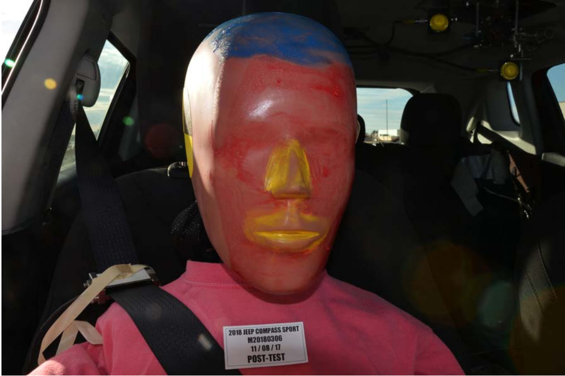
FIGURE 67. Post-Test Passenger Dummy Face
