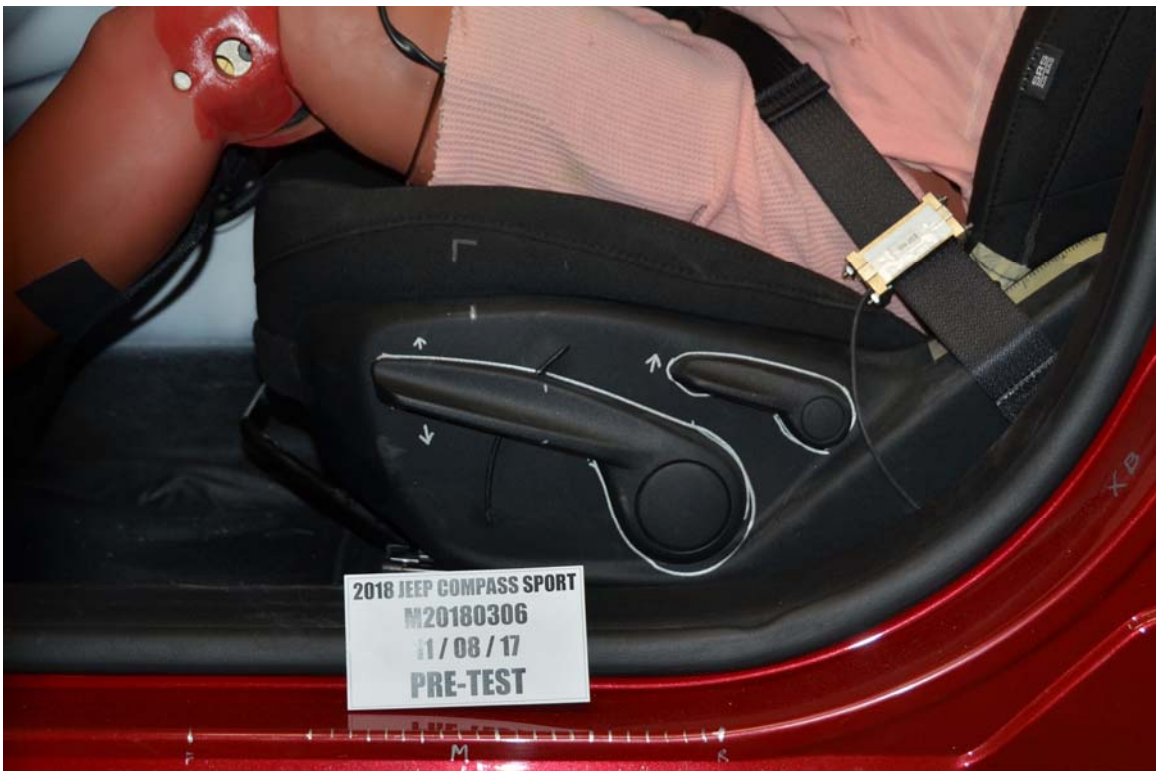
FIGURE 36. Pre-Test Driver's Seat Fore-Aft Markings
