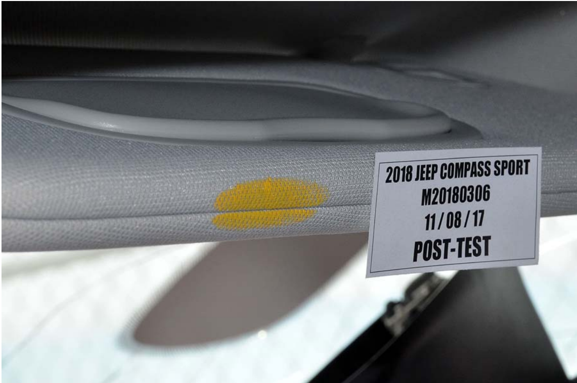
FIGURE 48a. Post-Test Driver Dummy Contact with Sun Visor
