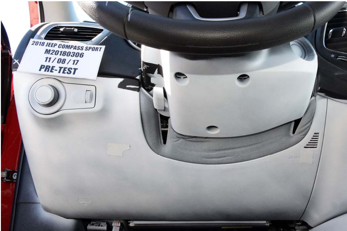
FIGURE 42. Pre-Test Driver's Side Knee Bolster
