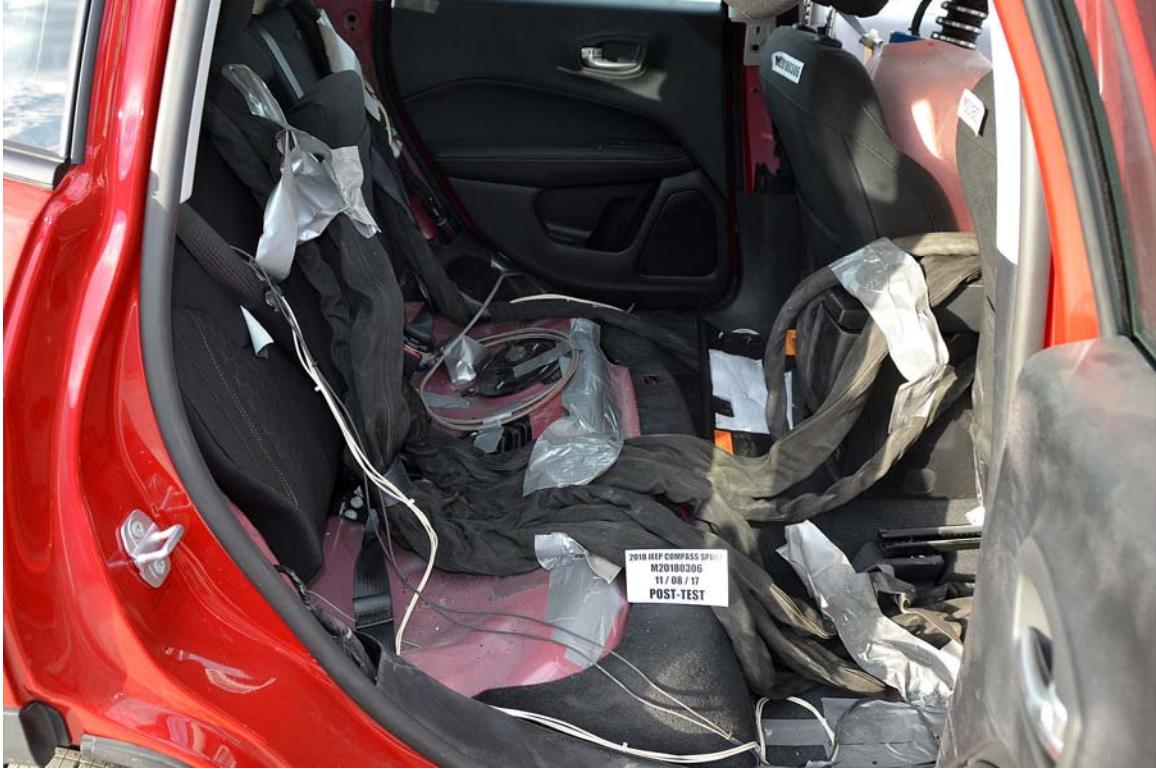
FIGURE 29. Post-Test Dummy Cable Routing
