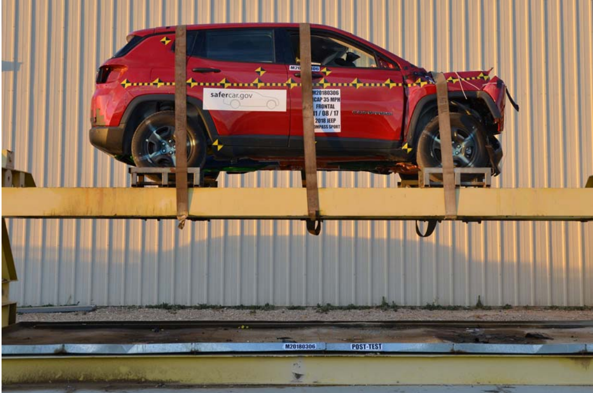
FIGURE 73. Vehicle at 0° on Static Rollover Device
