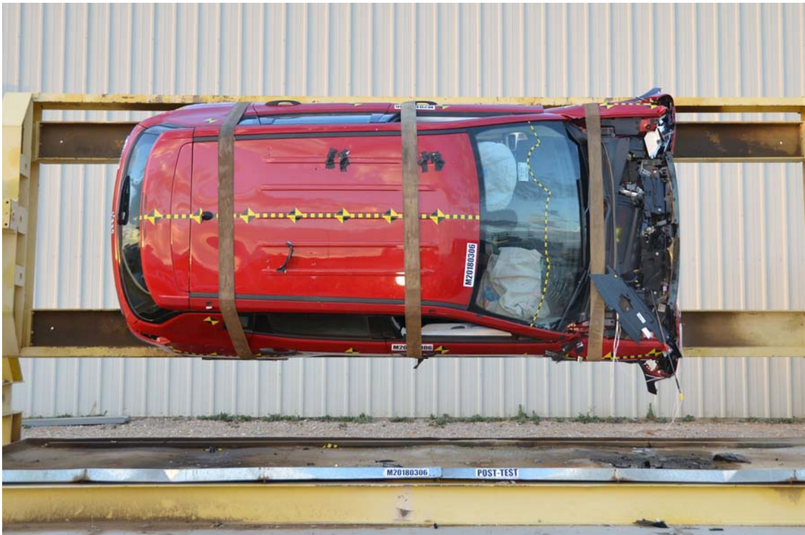
FIGURE 74. Vehicle at 90° on Static Rollover Device
