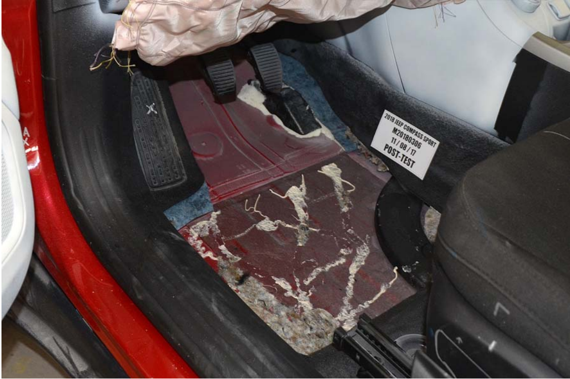
FIGURE 45. Post-Test Driver's Side Floorpan
