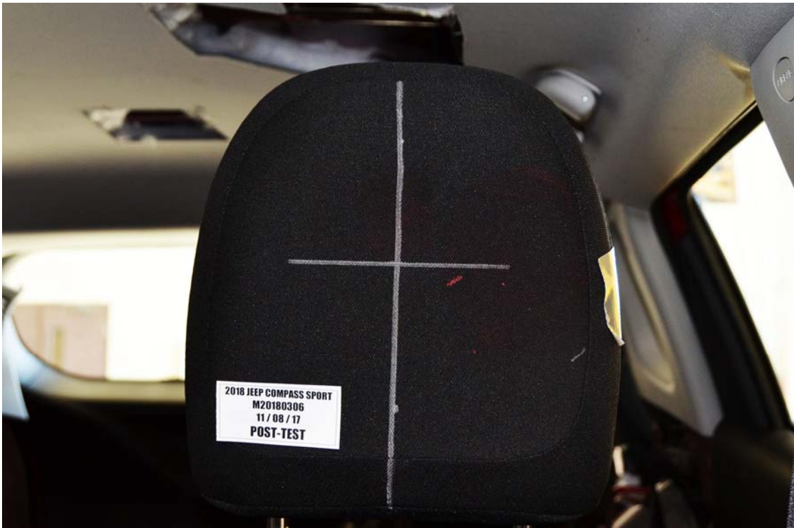
FIGURE 48. Post-Test Driver Dummy Contact with Headrest
