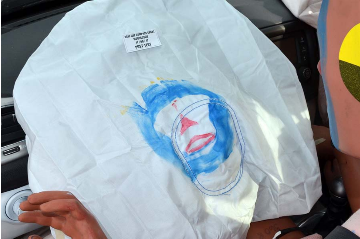
FIGURE 47. Post-Test Driver Dummy Contact with Airbag
