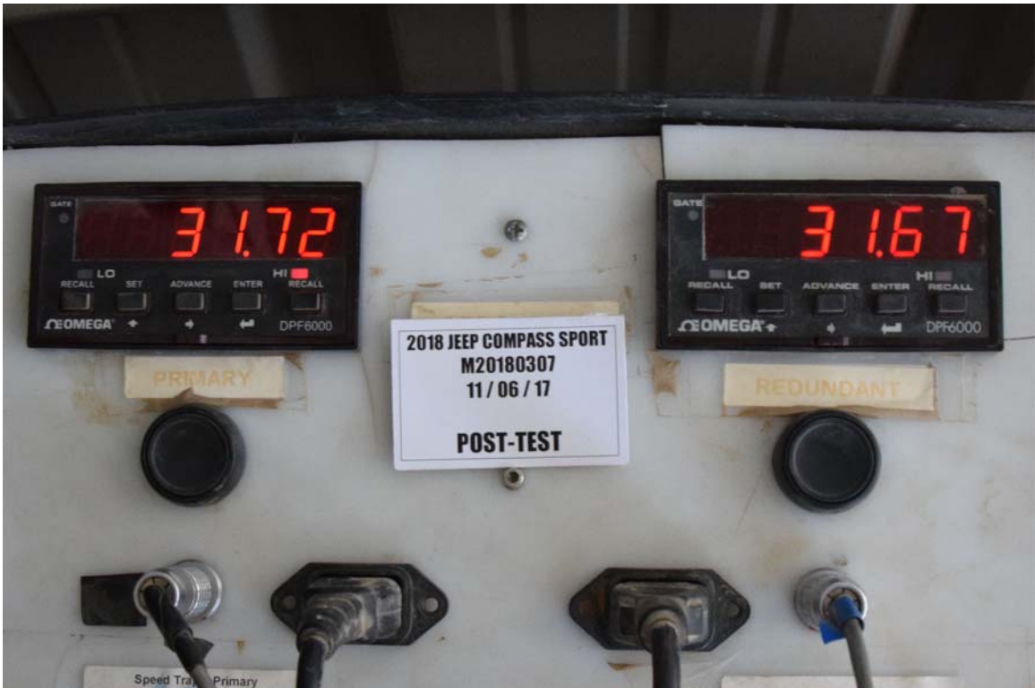
FIGURE 62. Post-Test Primary and Redundant Speed Trap Read-Out
