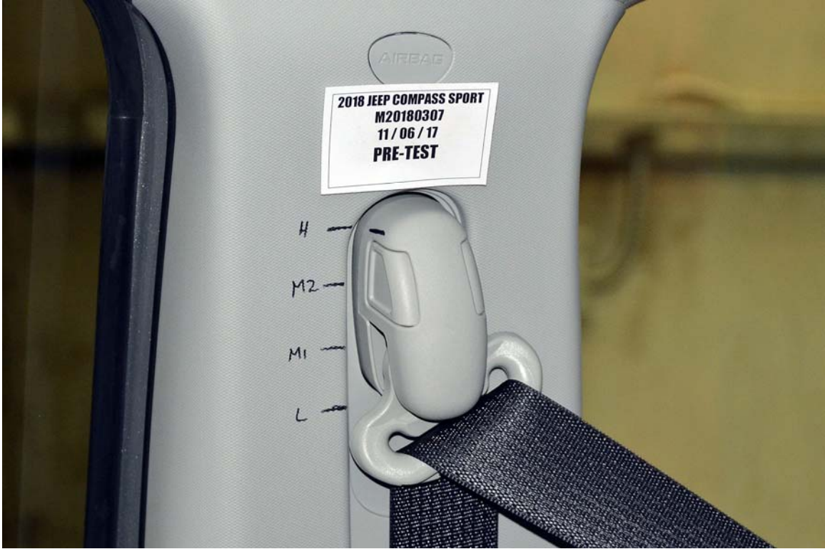
FIGURE 33. Pre-Test View of Belt Anchorage for Dummy
