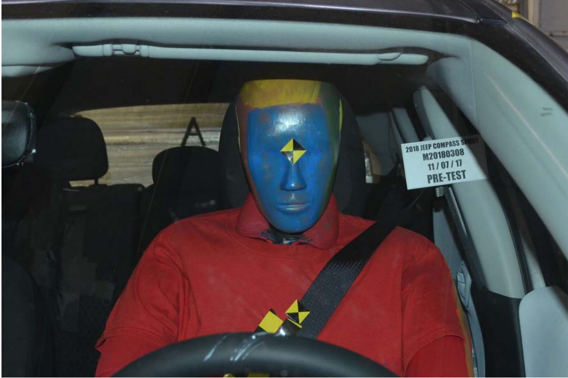
FIGURE 25. Pre-Test Front Close-Up View of Driver Dummy
