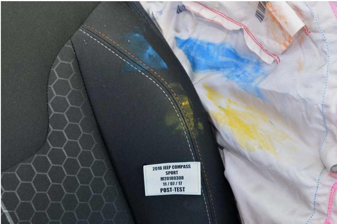
FIGURE 50. Post-Test Driver Dummy Close-Up Torso Contact with Vehicle Interior View
