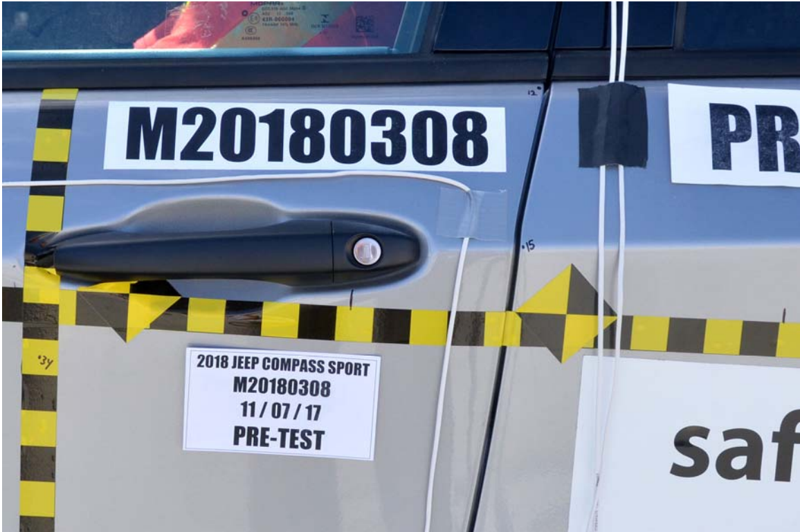
FIGURE 21. Pre-Test Left Front Door Latch Close-Up
