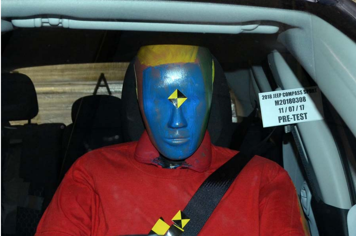
FIGURE 31. Pre-Test Frontal View of Driver Dummy Head and Shoulders in Relation to Head Restraint
