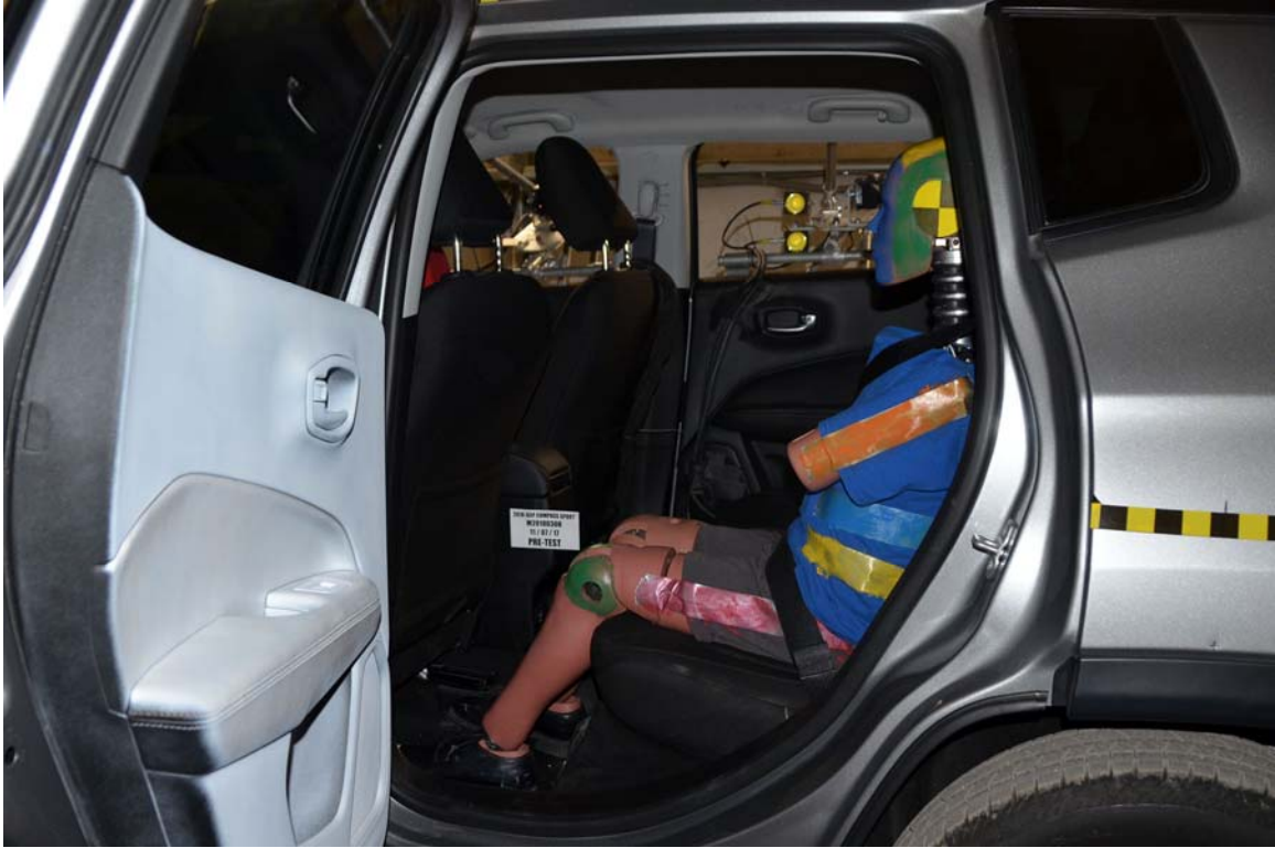
FIGURE 55. Pre-Test Left Side View of Rear Passenger Dummy Showing Belt and Chalking
