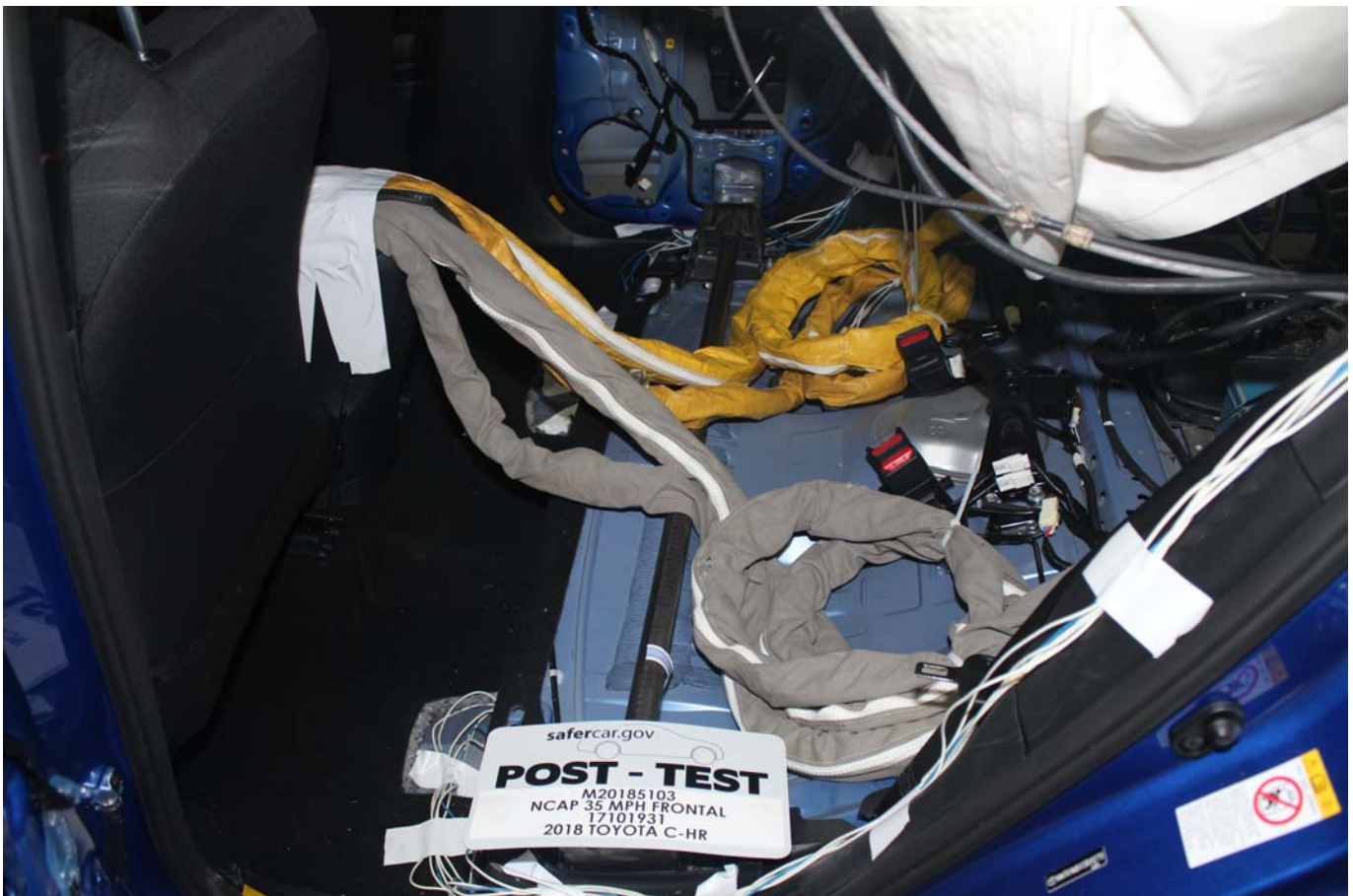
Photo No. 029 - Post-Test Dummy Cable Routing
