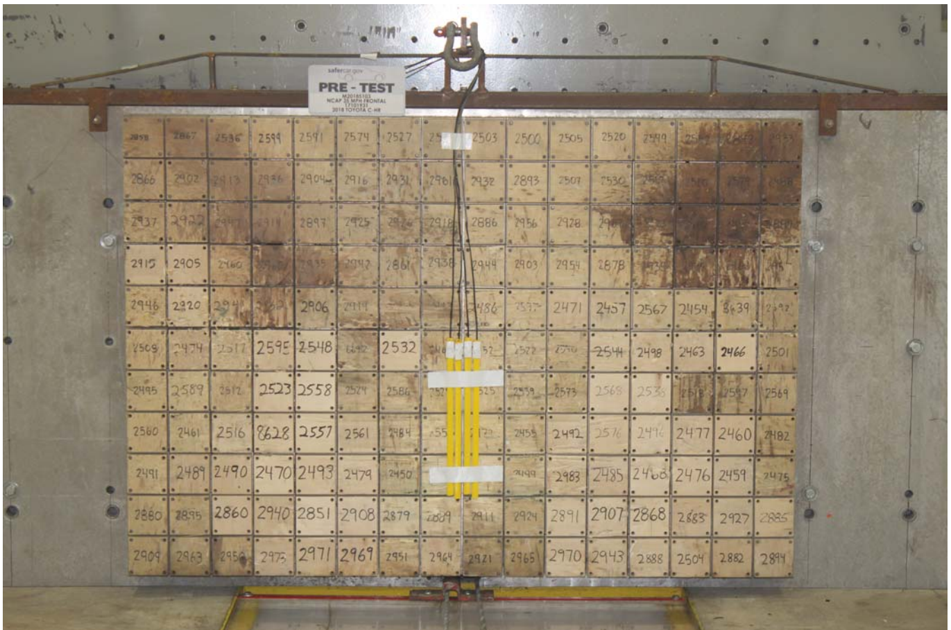
Photo No. 002 - Pre-Test Load Cell Wall
