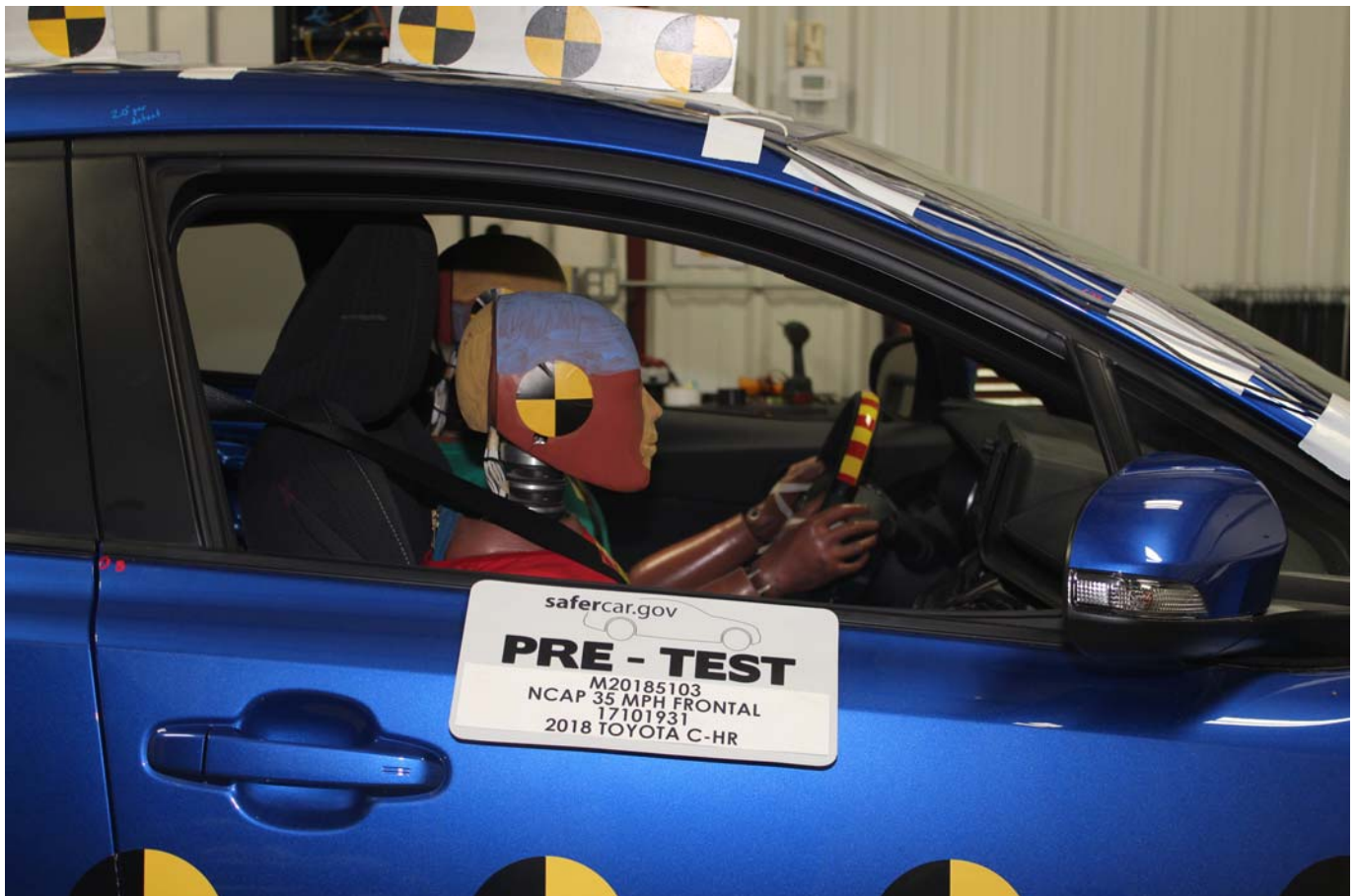
Photo No. 053 - Pre-Test Passenger Dummy Window View
