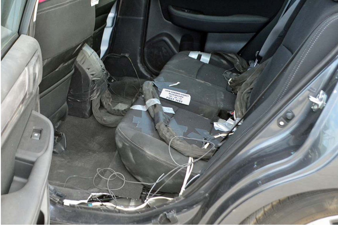
FIGURE 29. Post-Test Dummy Cable Routing
