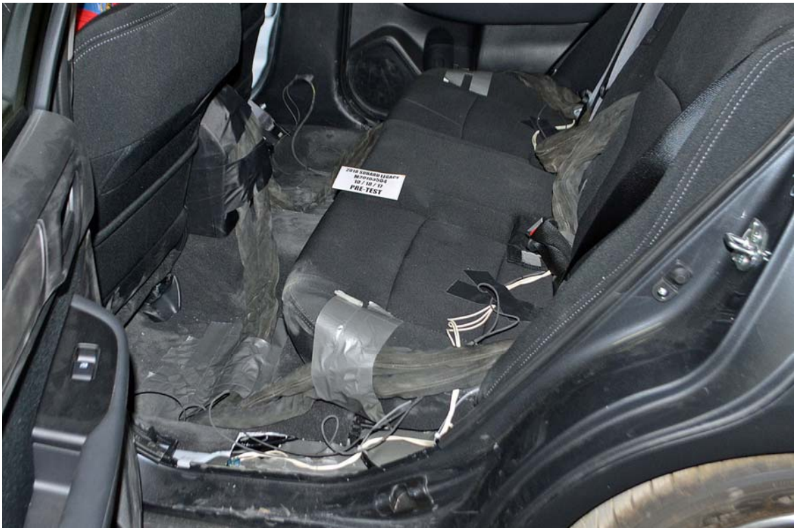
FIGURE 28. Pre-Test Dummy Cable Routing
