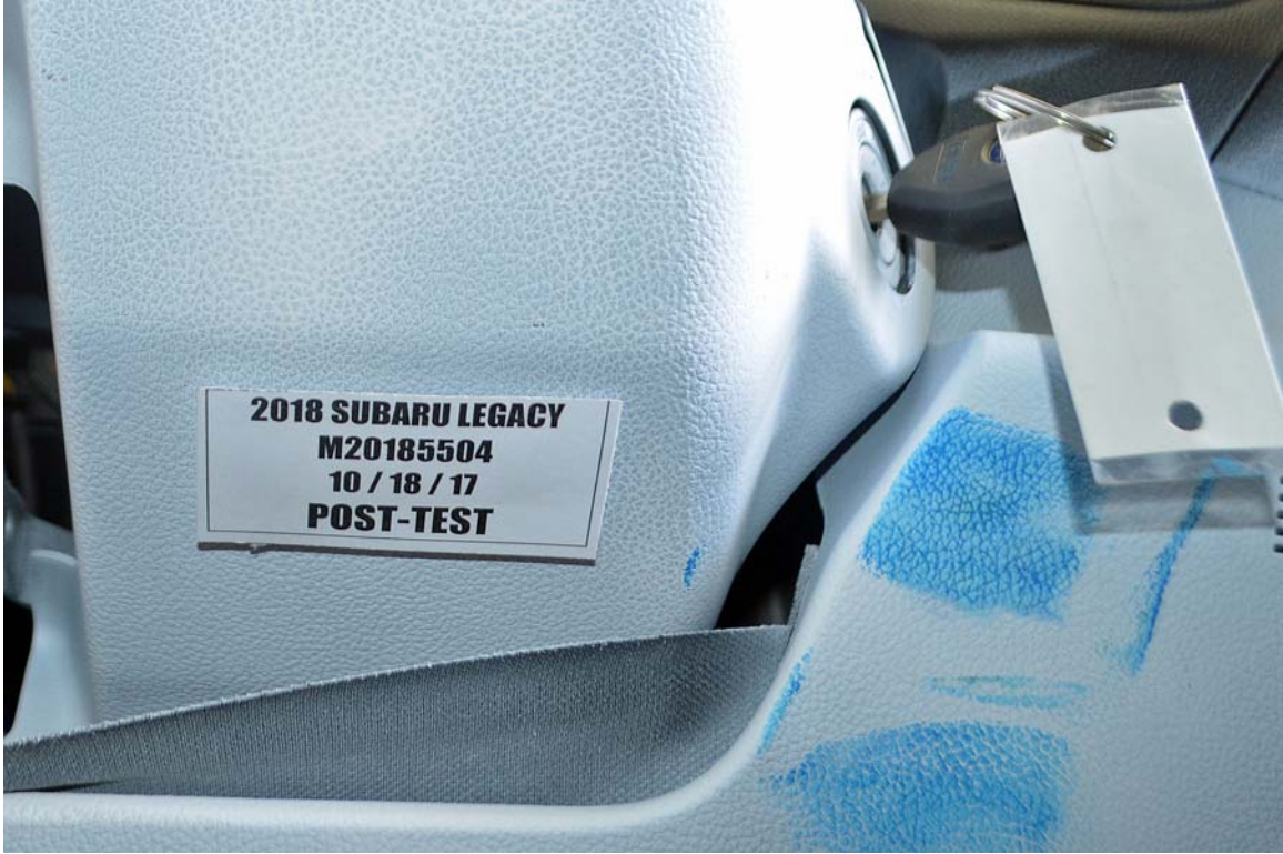
FIGURE 48a. Post-Test Driver Dummy Contact with Steering Column
