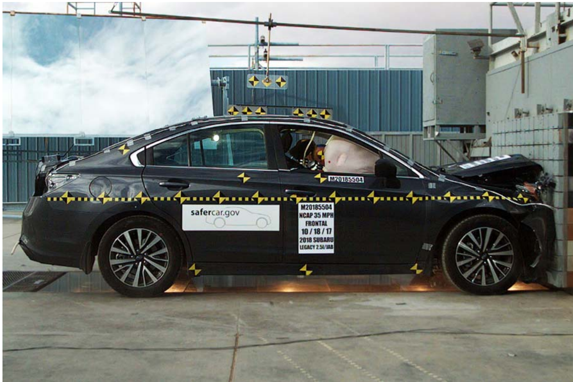
FIGURE 78. 2018 Subaru Legacy 2.5i/JAB Frontal Impact Event
