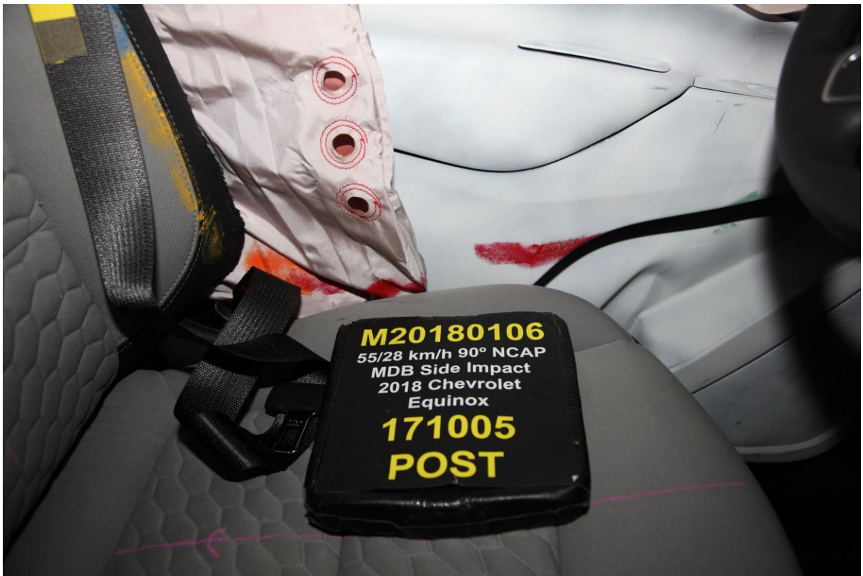
052 Post-Test Driver Dummy Close-Up Pelvis Contact View
