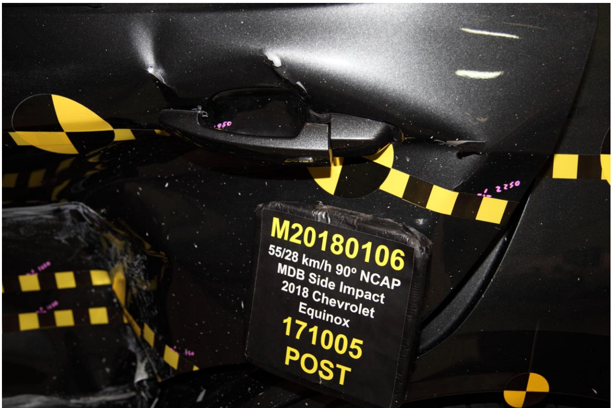
024 Post-Test Left Rear Door Latch Close-Up
