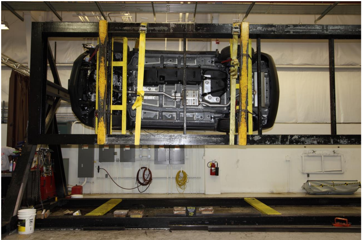
099 FMVSS No. 301 Static Rollover 270 Degrees
