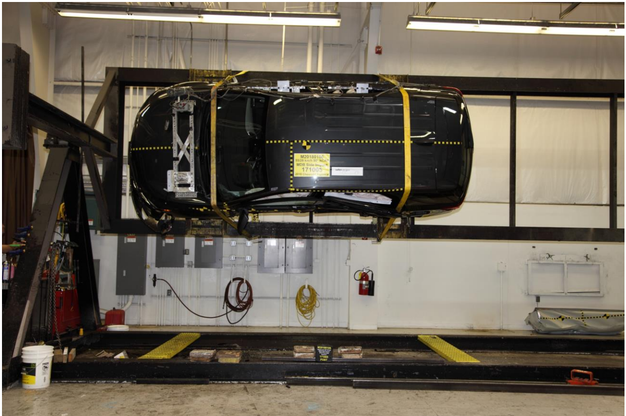
097 FMVSS No. 301 Static Rollover 90 Degrees
