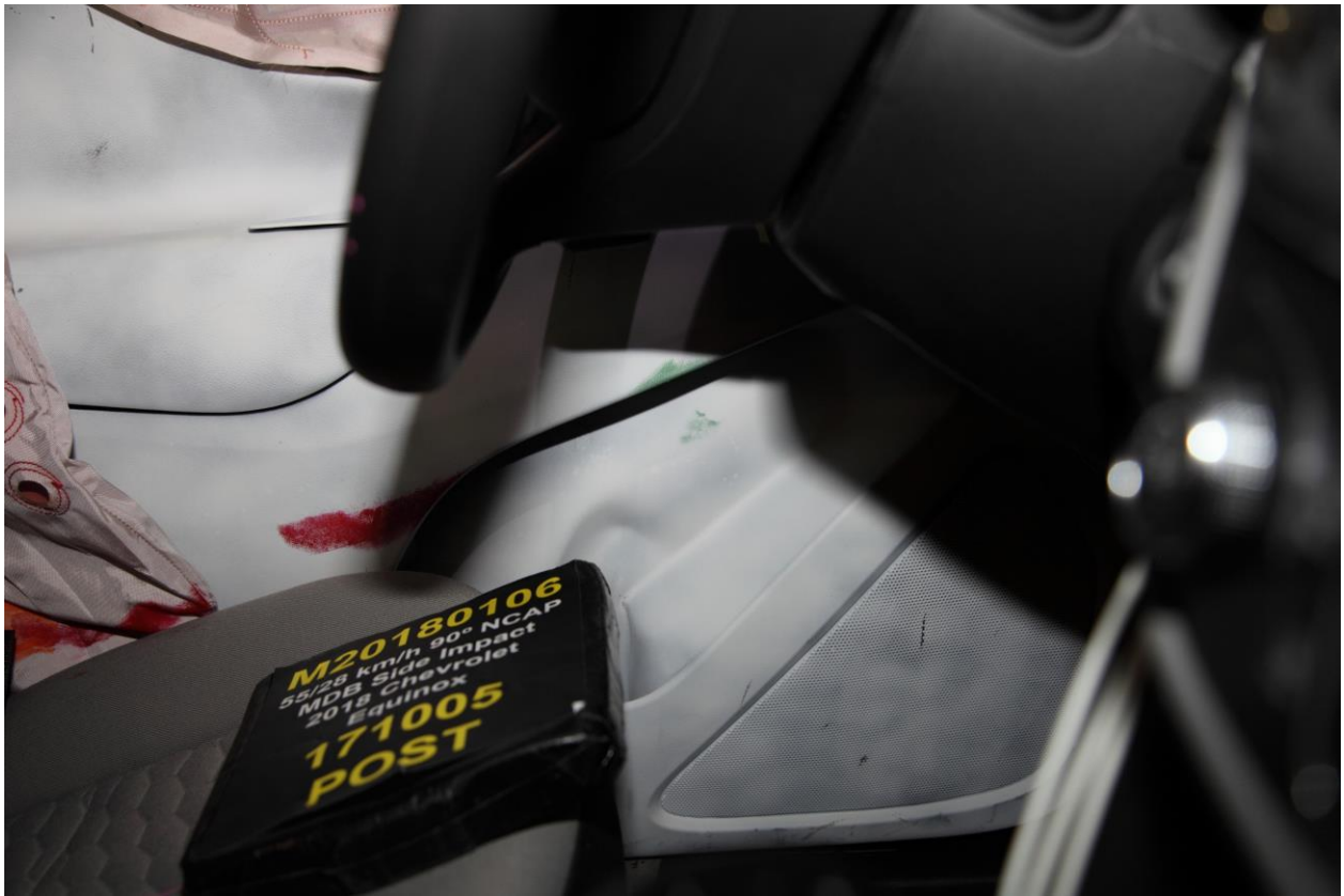
054 Post-Test Driver Dummy Close-Up Knee Contact View
