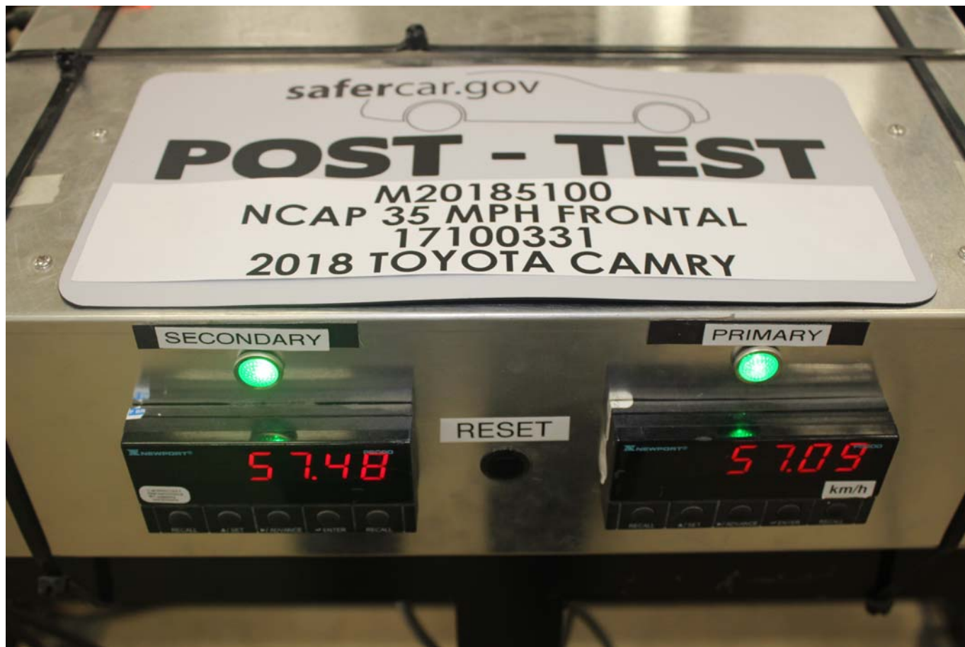
Photo No. 072 - Post-Test Speed Trap Read-Out
