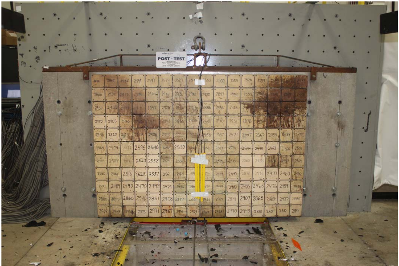
Photo No. 003 - Post-Test Load Cell Wall
