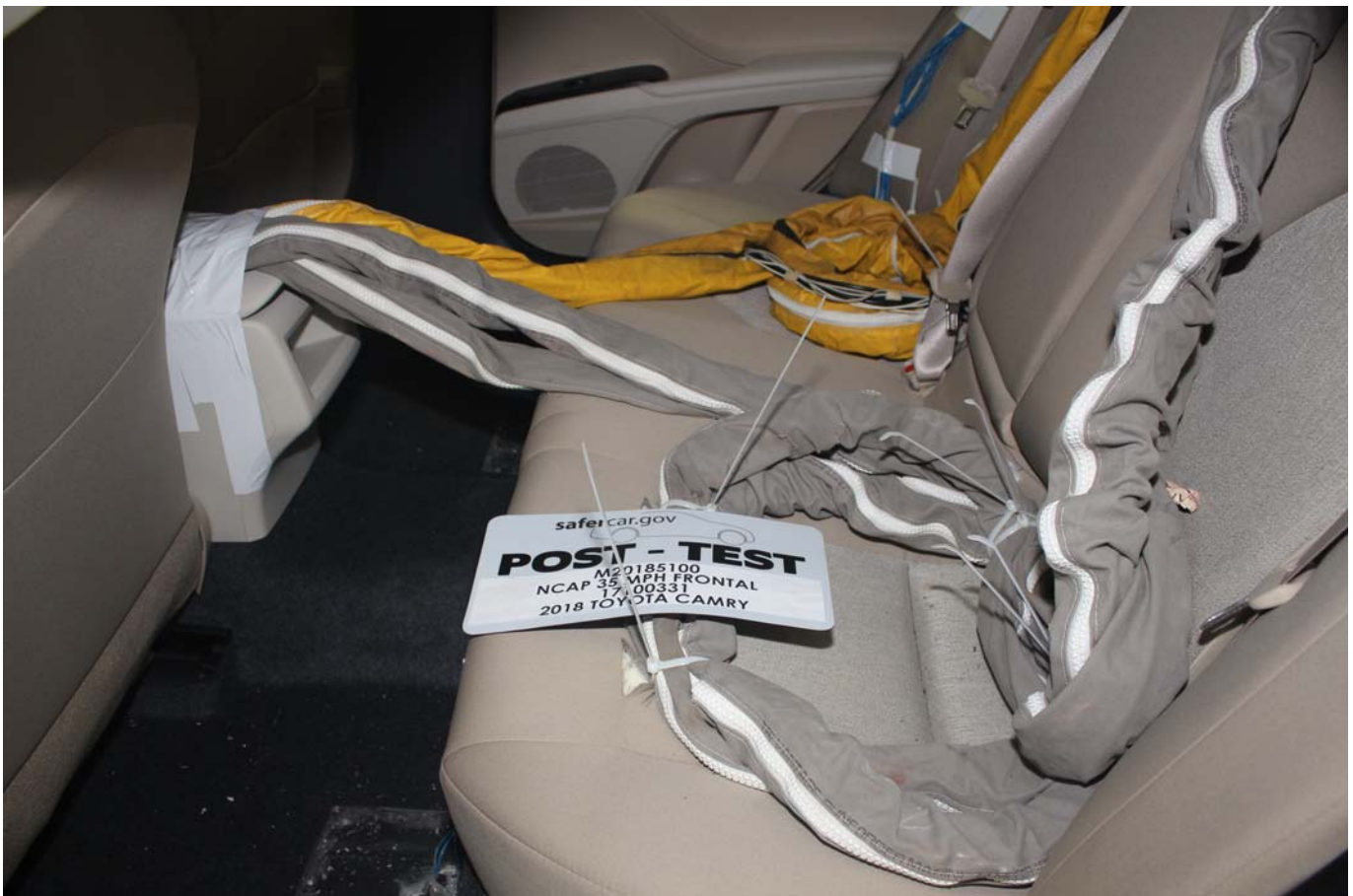
Photo No. 029 - Post-Test Dummy Cable Routing
