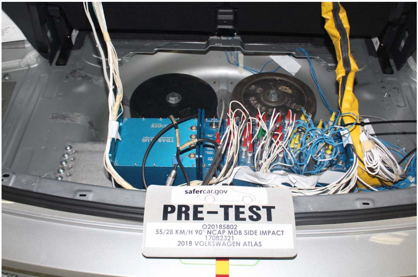
Photo No. 094 - Pre-Test Ballast View
