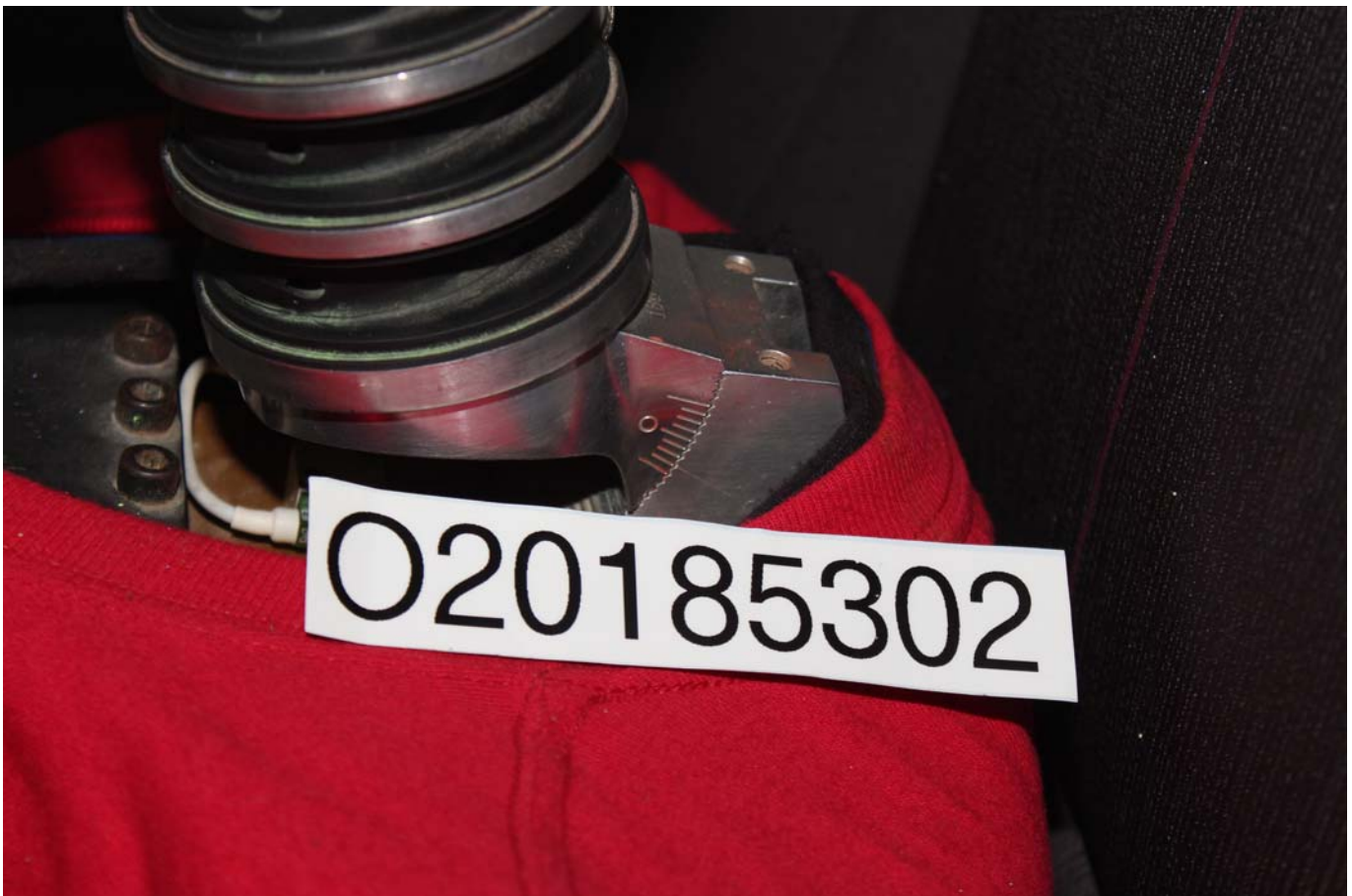
Photo No. 062 - Pre-Test View of Rear Passenger Dummy Neck Showing Position of Adjustable Neck Bracket
