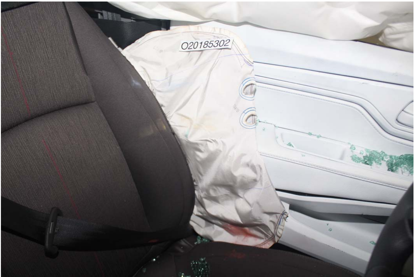
Photo No. 051 - Post-Test Driver Dummy Close-up Torso Contact with Side Airbag View
