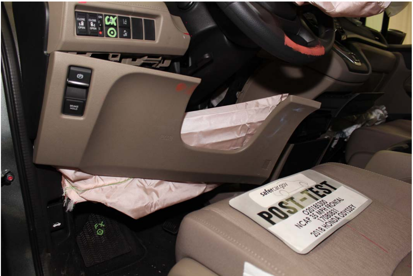
Photo No. 043 - Post-Test Driver Side Knee Bolster (without dummy)
