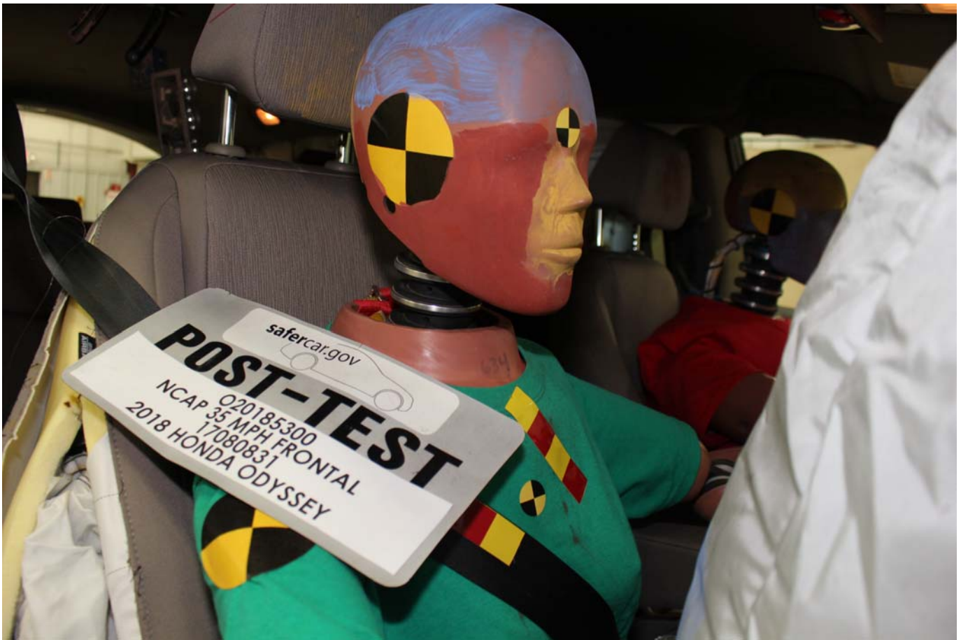
Photo No. 067 - Post-Test Passenger Dummy Face
