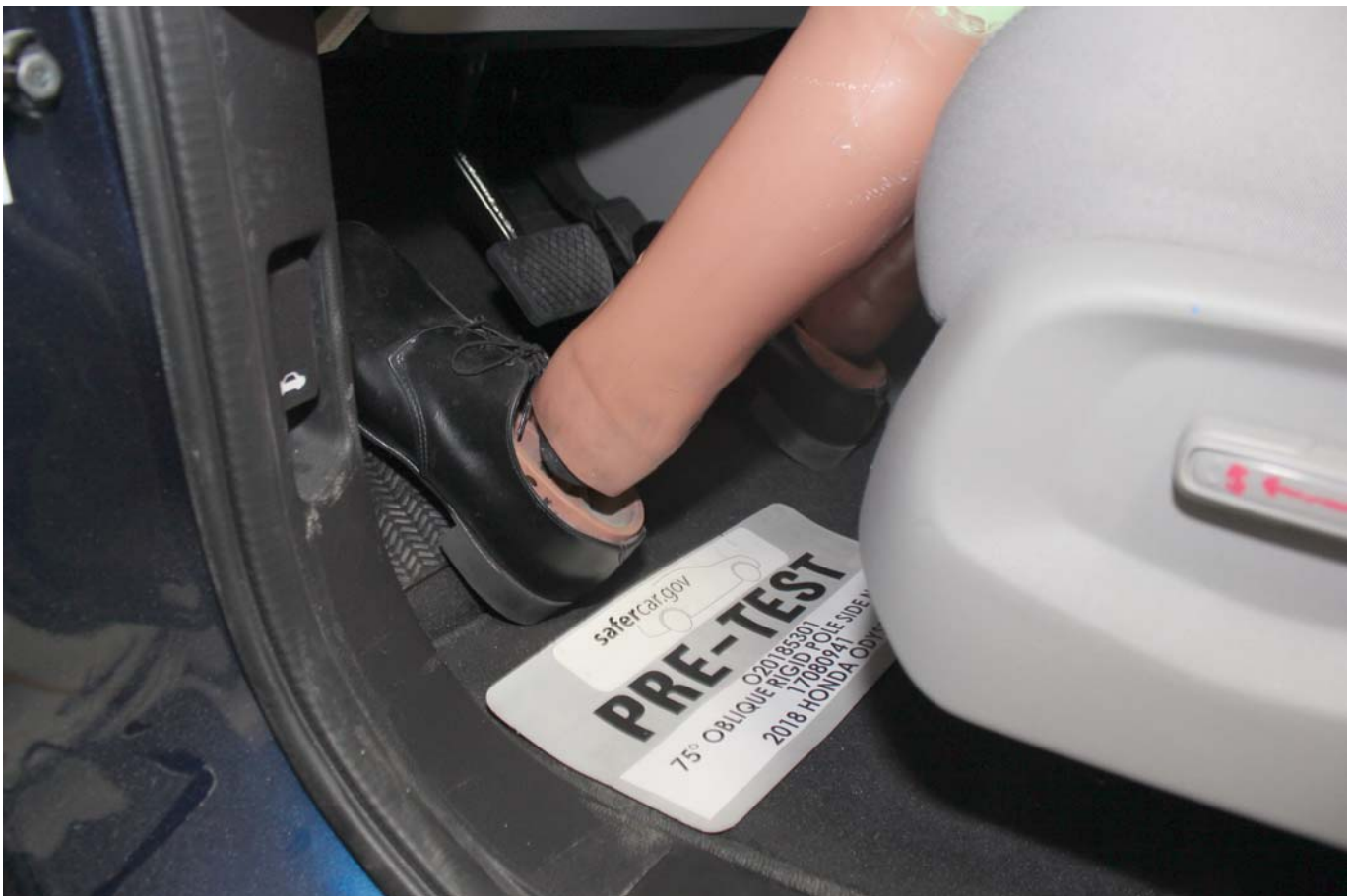
Photo No. 032 - Pre-Test Placement of Dummy Feet
