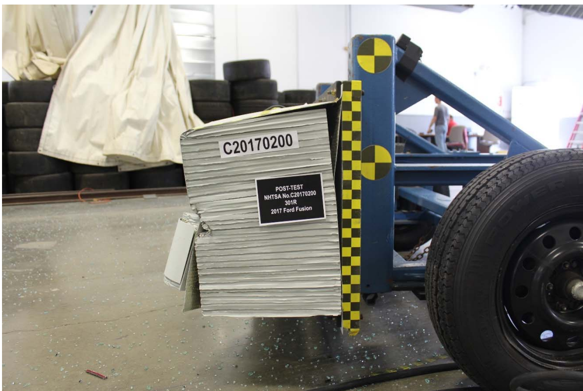
Figure A-22: Post-Test MDB Left Side View
