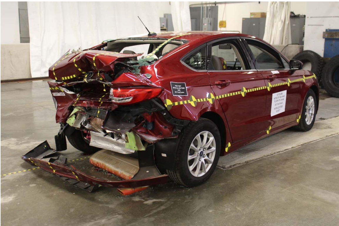
Figure A-16: Post-Test Right Rear 3/4 View
