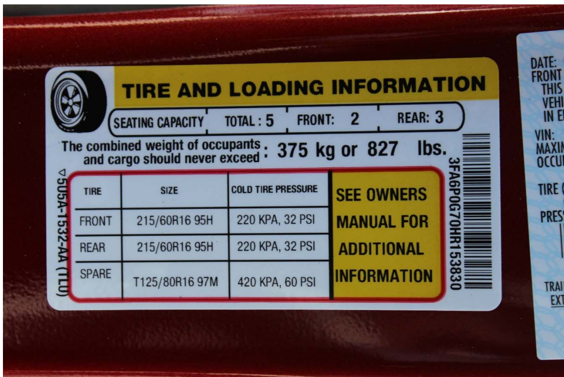
Figure A-2: Vehicle Tire Placard
