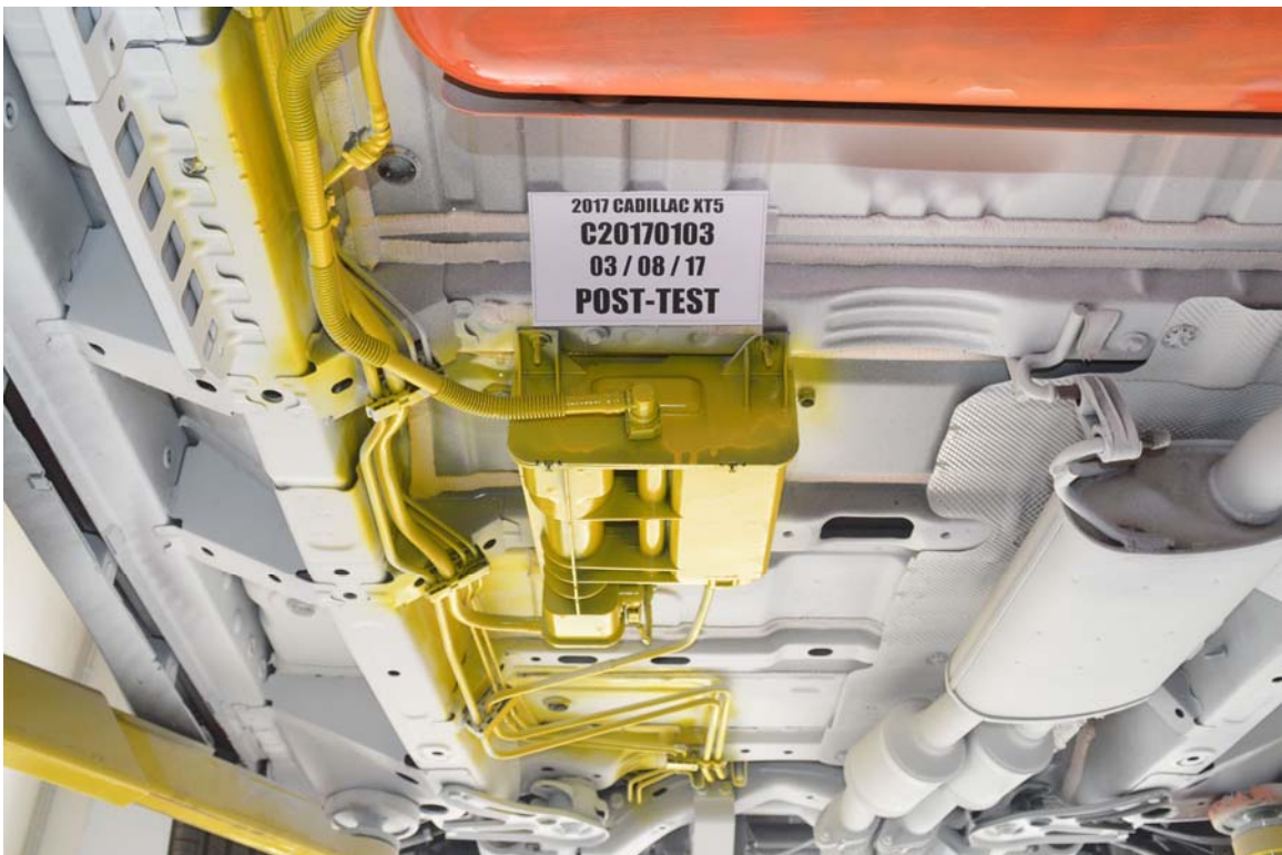
FIGURE 30. Post-Test Underbody View of Fuel Lines
