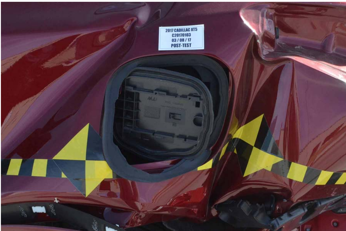
FIGURE 24. Post-Test View of Fuel Filler Cap
