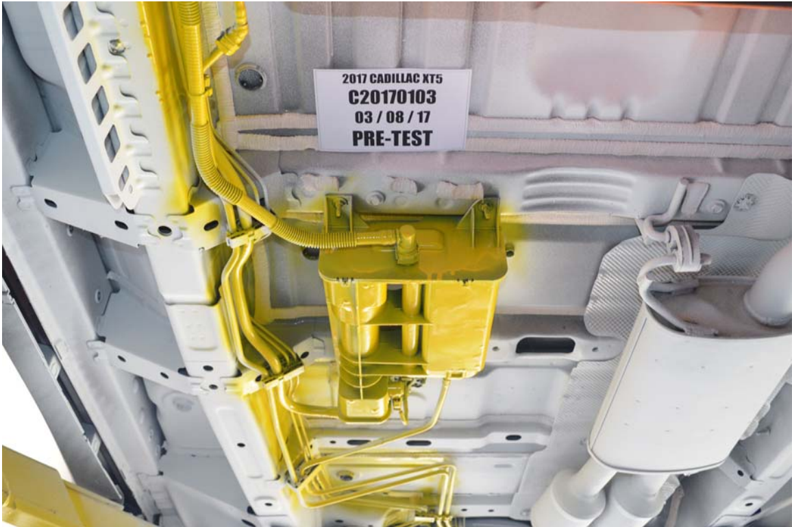
FIGURE 29. Pre-Test Underbody View of Fuel Lines
