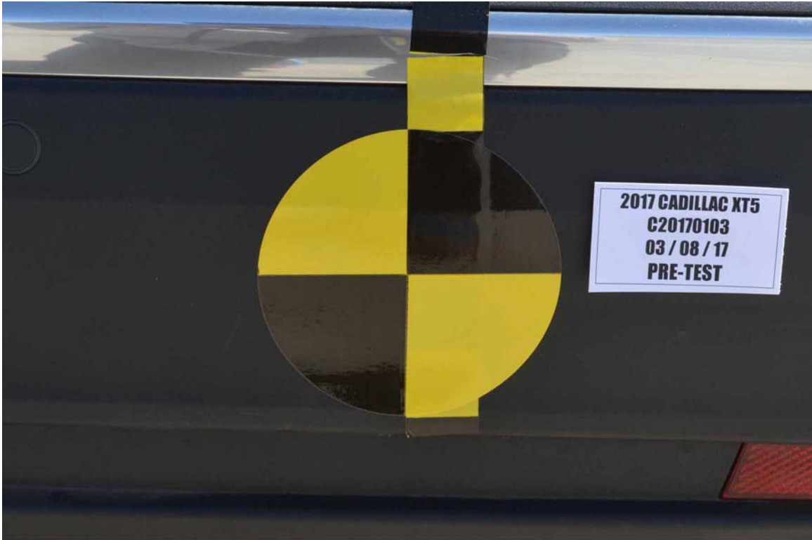
FIGURE 21. Pre-Test Close-Up View of Impact Point Target
