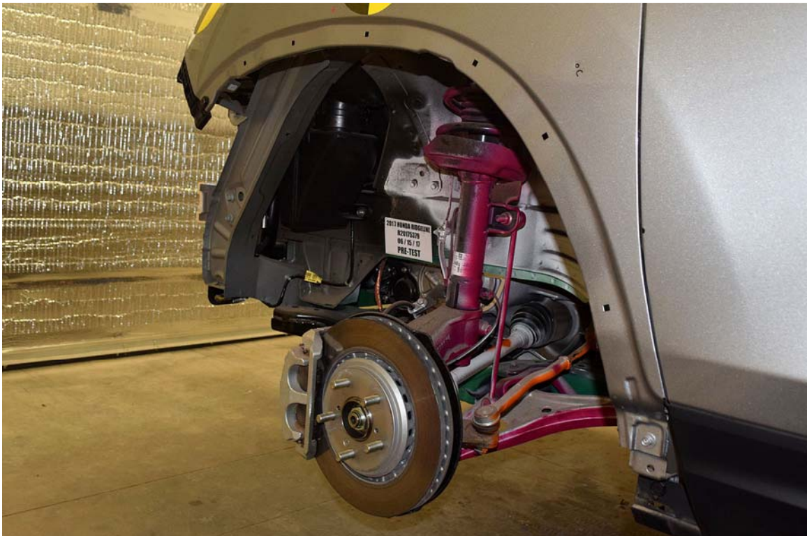
FIGURE 154. Pre-Test Oblique Left Side View of Front of Wheel Well With Parts Removed
