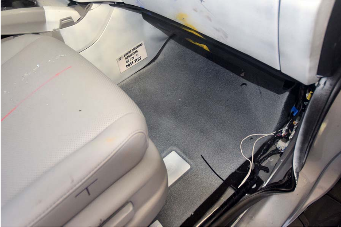
FIGURE 113. Post-Test View of Passenger Floor Pan at Right Sill Level
