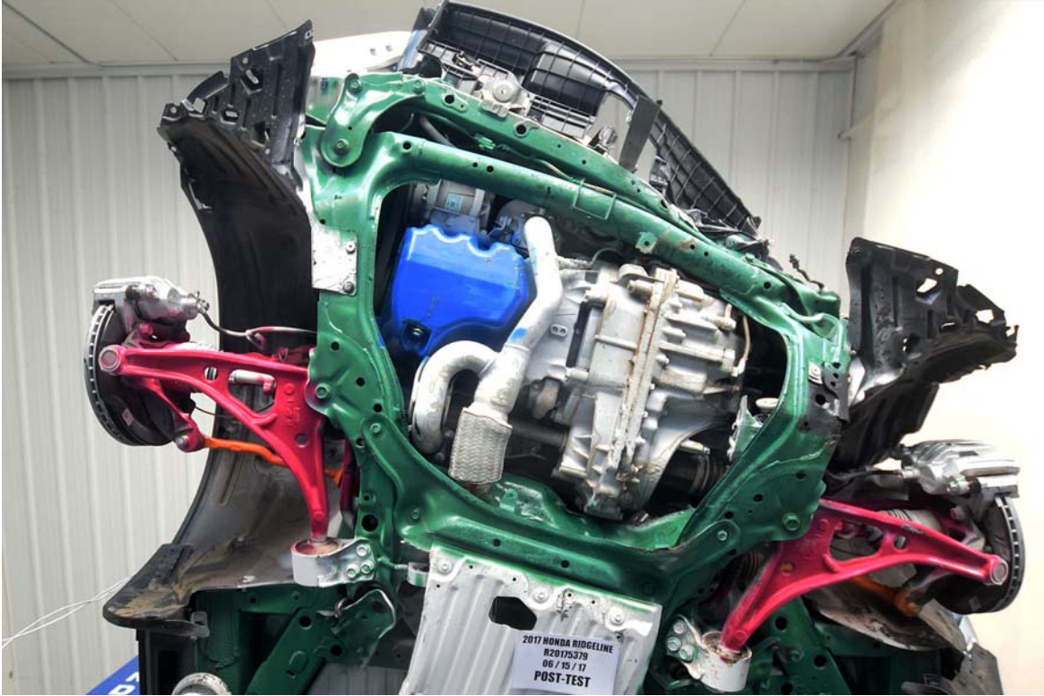
FIGURE 141. Post-Test Bumper to Rail Attachments and Crush Initiators with Parts Removed
