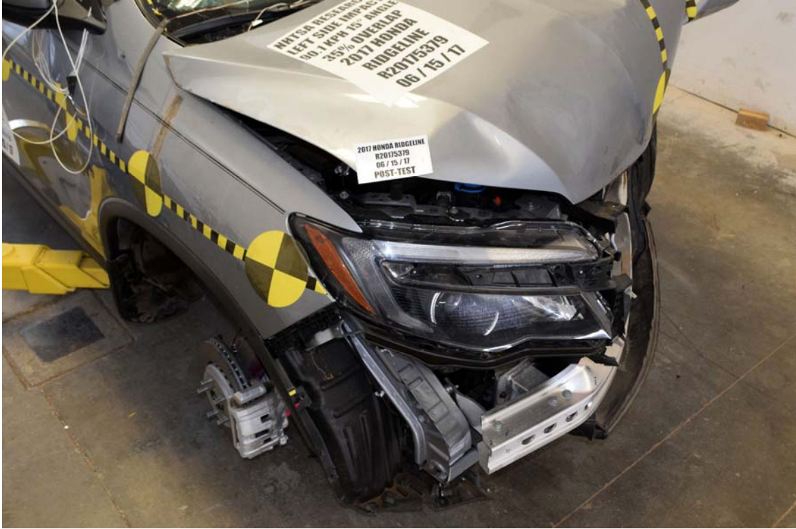
FIGURE 167. Post-Test Oblique View of Right Front of the Vehicle with Parts Removed
