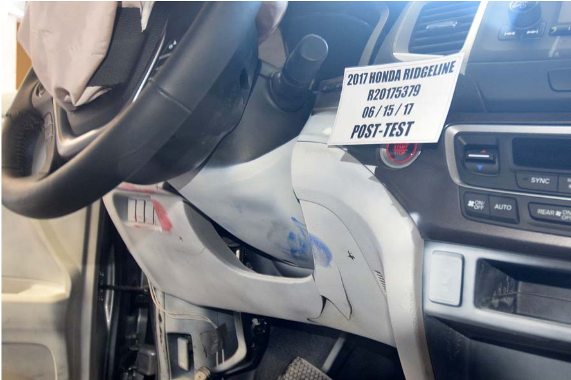
FIGURE 61. Post-Test Right Side View of Driver Knee Bolster
