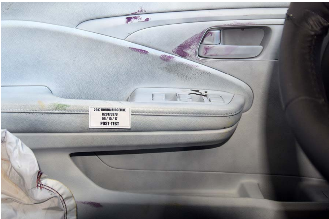
FIGURE 72. Post-Test Driver Dummy Close-Up Torso Contact with Vehicle Interior View
