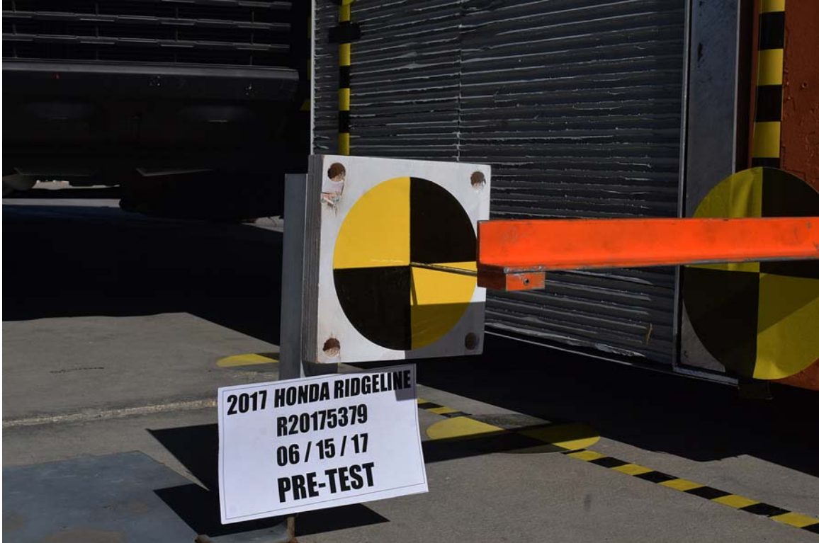
FIGURE 17. Pre-Test Close-up View of Impact Point
