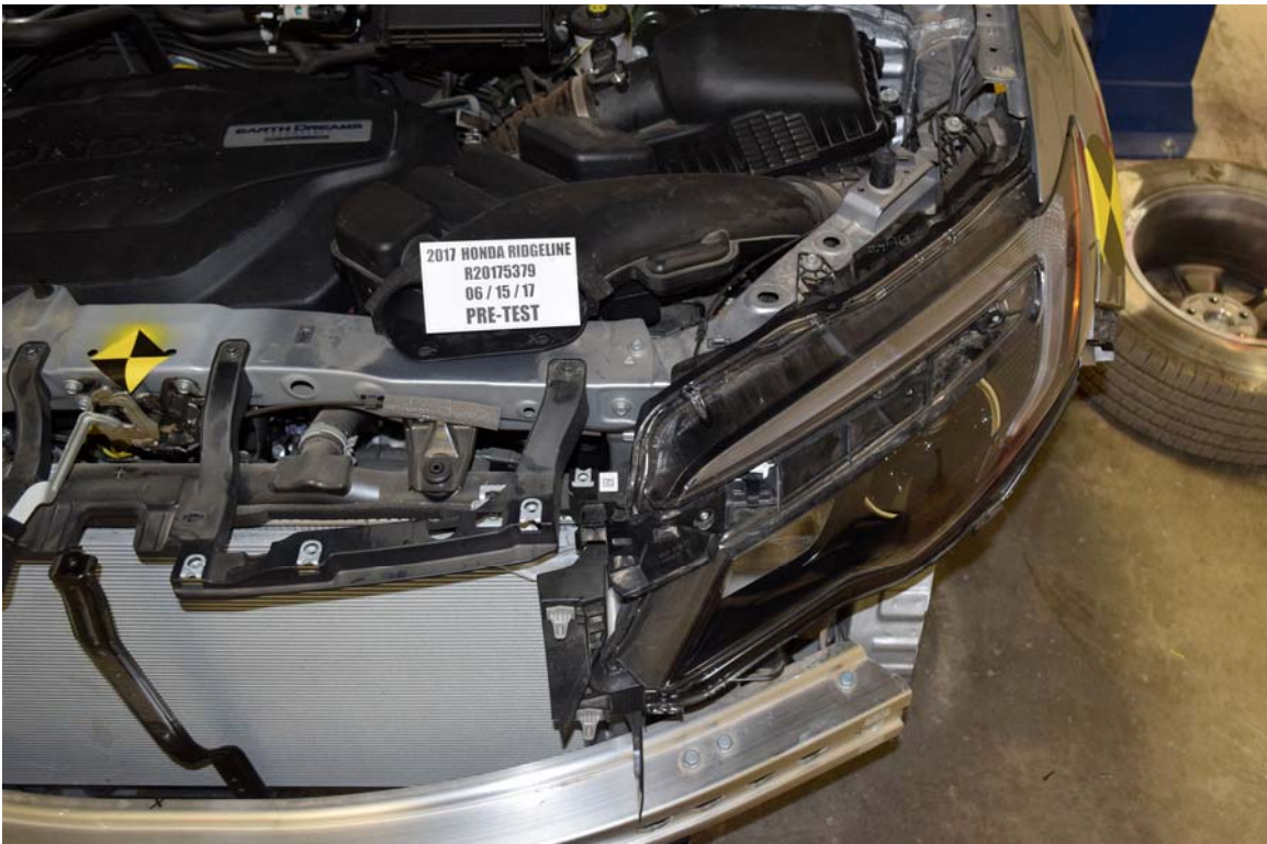
FIGURE 130. Pre-Test Left Side Energy Absorber with Parts Removed
