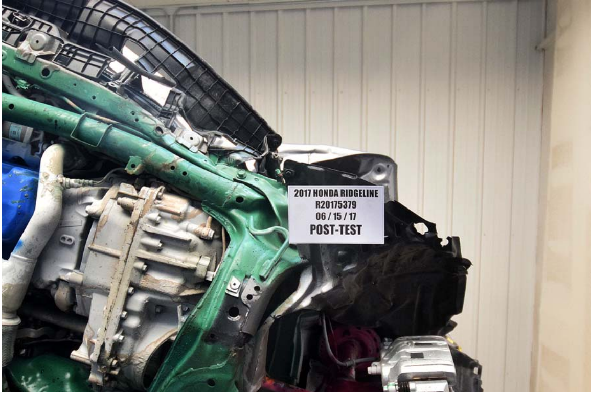
FIGURE 143. Post-Test Driver Bumper to Rail Attachments and Crush Initiators with Parts Removed
