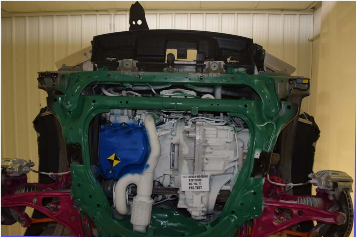
FIGURE 140. Pre-Test Bumper to Rail Attachments and Crush Initiators with Parts Removed
