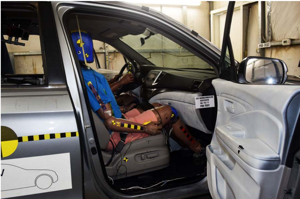
FIGURE 82. Pre-Test Right Side View of Passenger And Interior (Perpendicular View)
