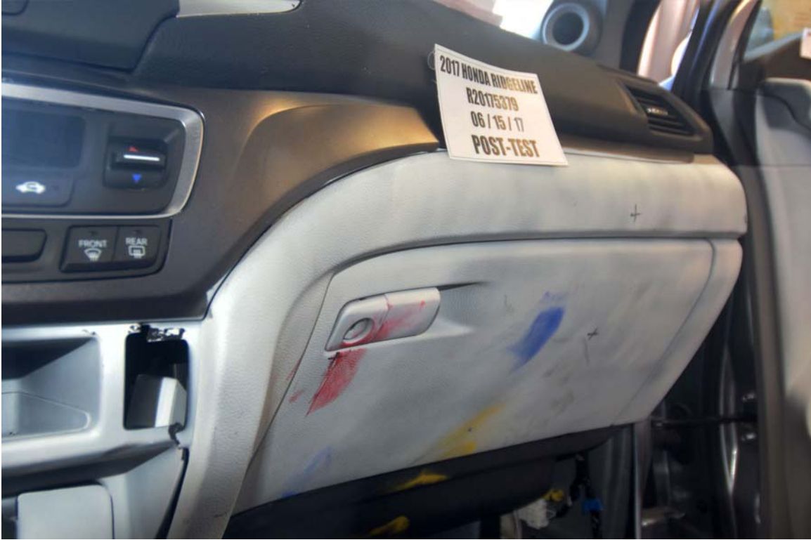
FIGURE 111. Post-Test Left Side View of Passenger Knee Bolster
