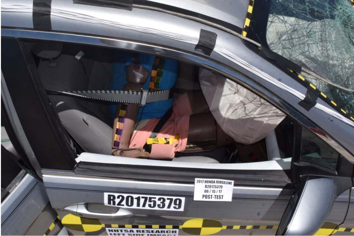
FIGURE 81. Post-Test View of Passenger Door Clearance
