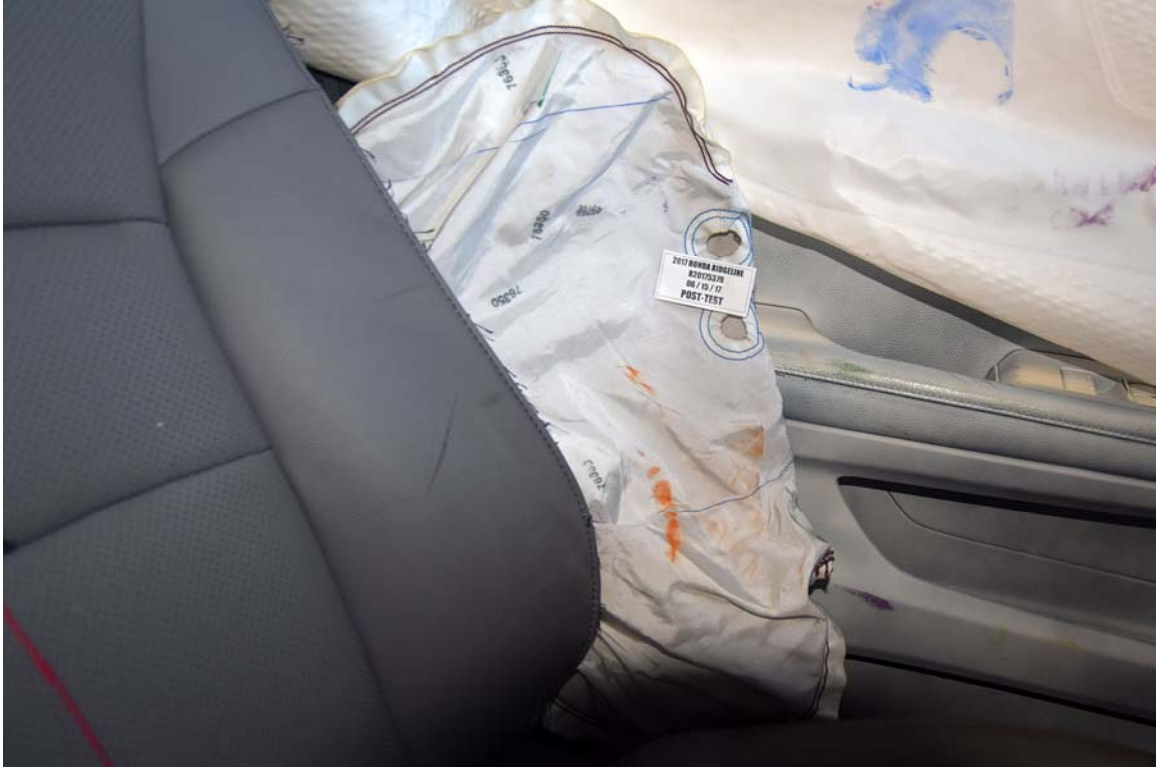
FIGURE 73. Post-Test Driver Dummy Close-Up Torso Contact with Side Airbag View
