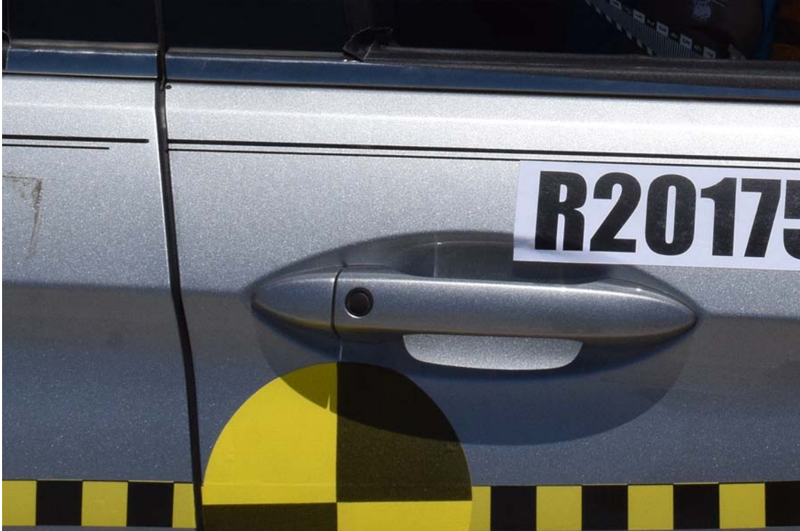
FIGURE 103. Post-Test Close-up View of Passenger Door Latch
