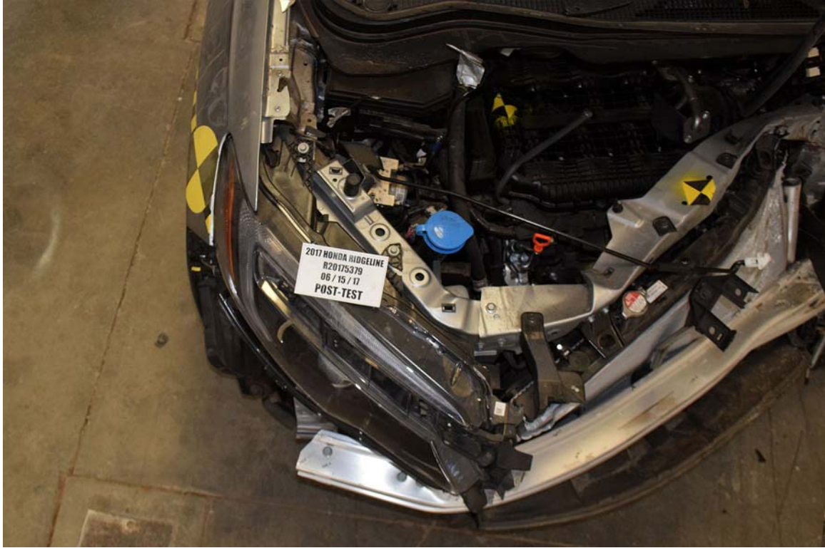
FIGURE 133. Post-Test Right Side Energy Absorber With Parts Removed
