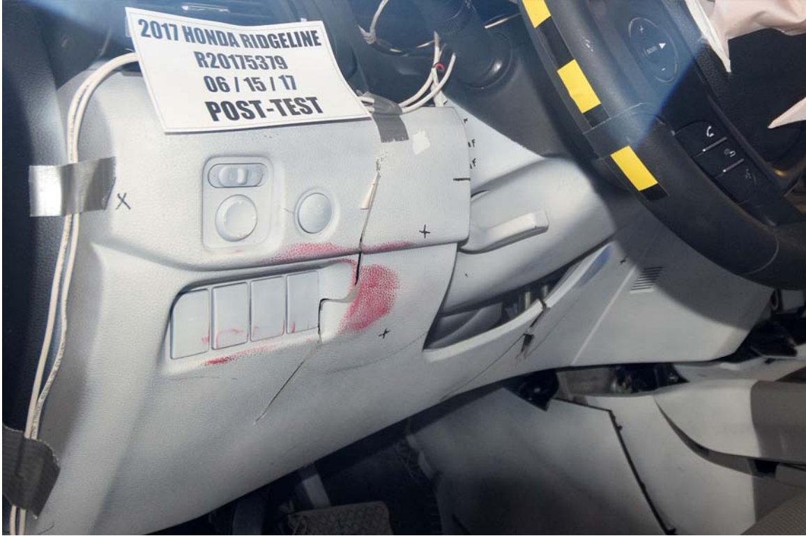
FIGURE 57. Post-Test Left Side View of Driver Knee Bolster
