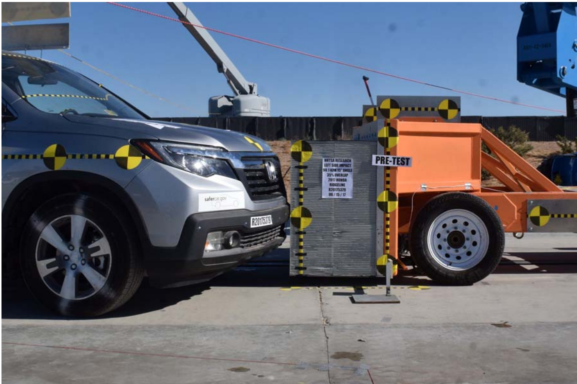
FIGURE 14. Pre-Test Left Side of OMDB Against Target Vehicle at Ideal Impact Point
