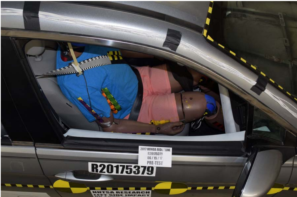
FIGURE 80. Pre-Test View of Passenger Door Clearance
