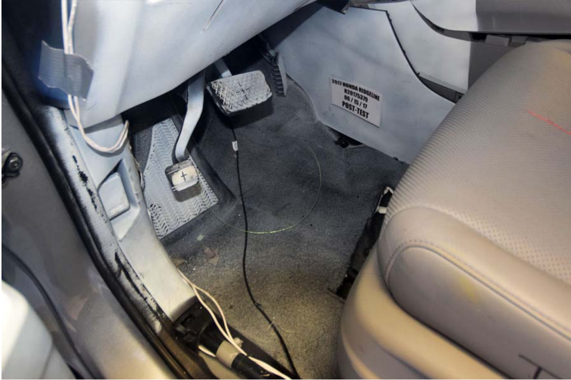
FIGURE 63. Post-Test View of Driver Floor Pan at Left Sill Level
