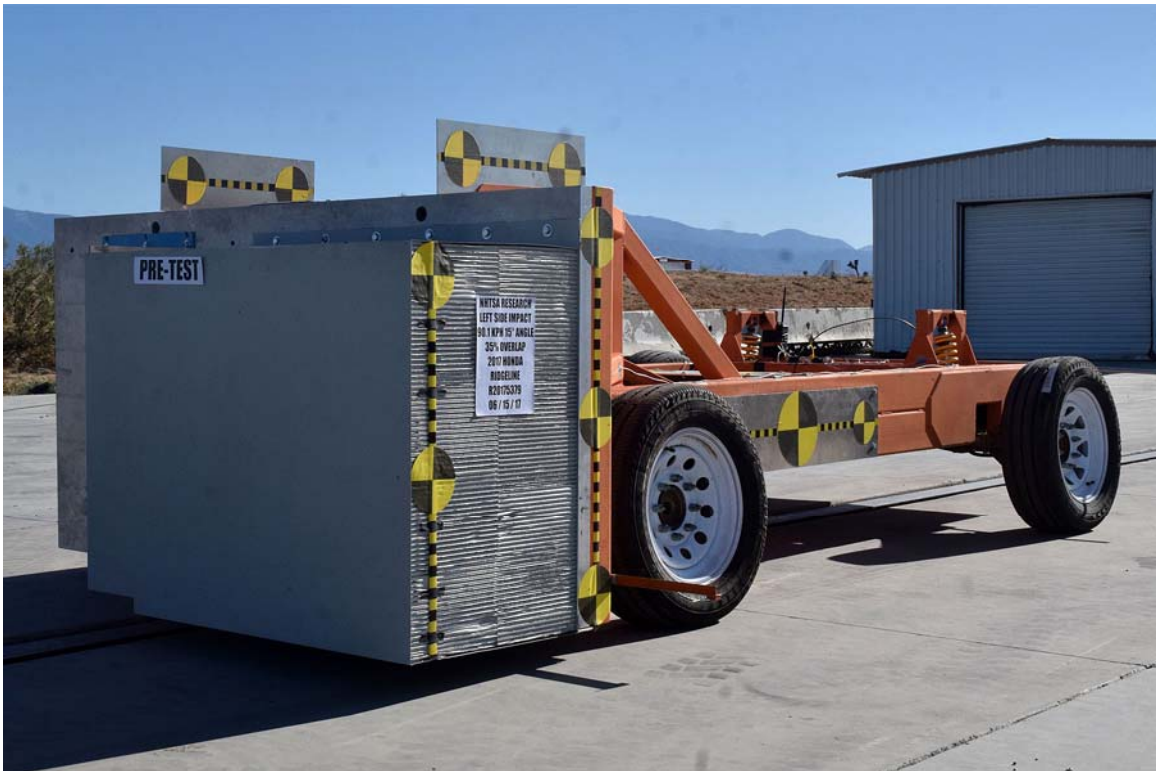
FIGURE 172. Pre-Test Left Oblique View of OMDB
