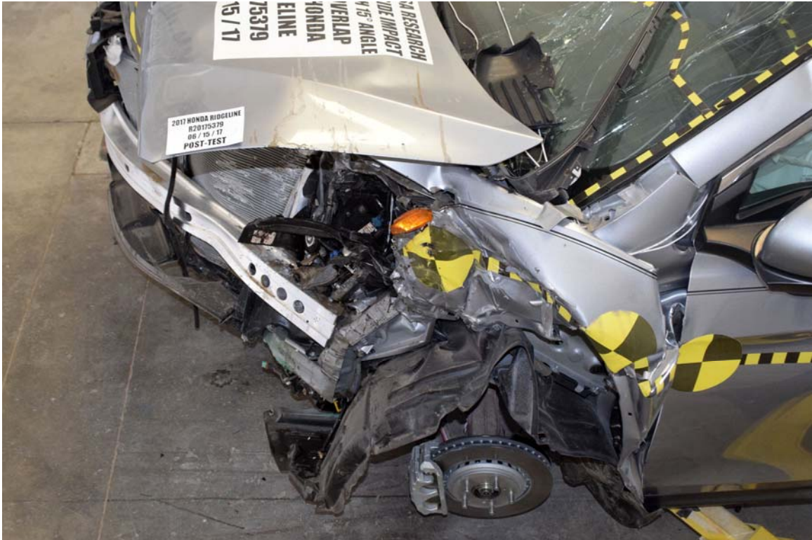
FIGURE 157. Post-Test Oblique View of Left Front Fender from Above with Parts Removed
