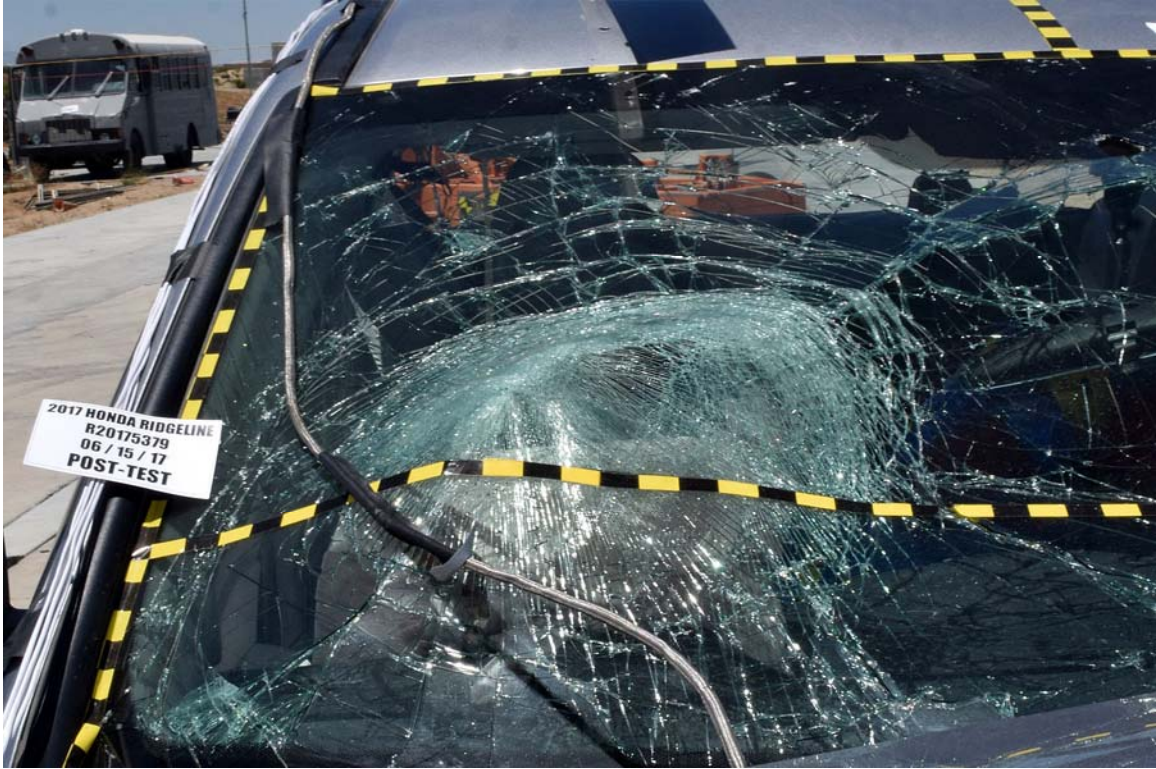
FIGURE 77. Post-Test Passenger Front Windshield View
