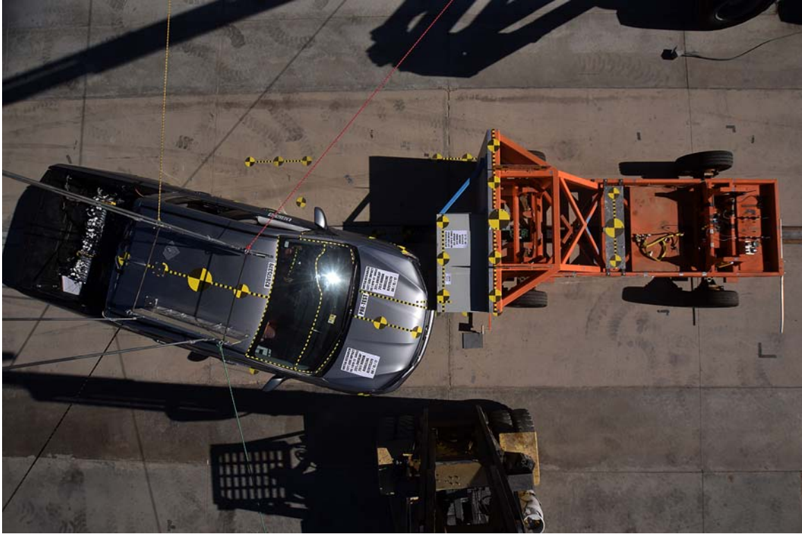
FIGURE 13. Pre-Test Overhead View of OMDB Against Test Vehicle at Ideal Impact Point
