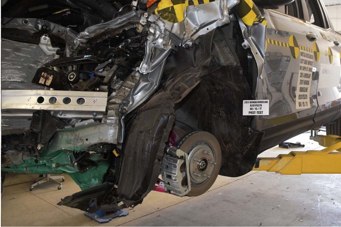
FIGURE 151. Post-Test Oblique Left Side View of Rear of Wheel Well with Parts Removed
