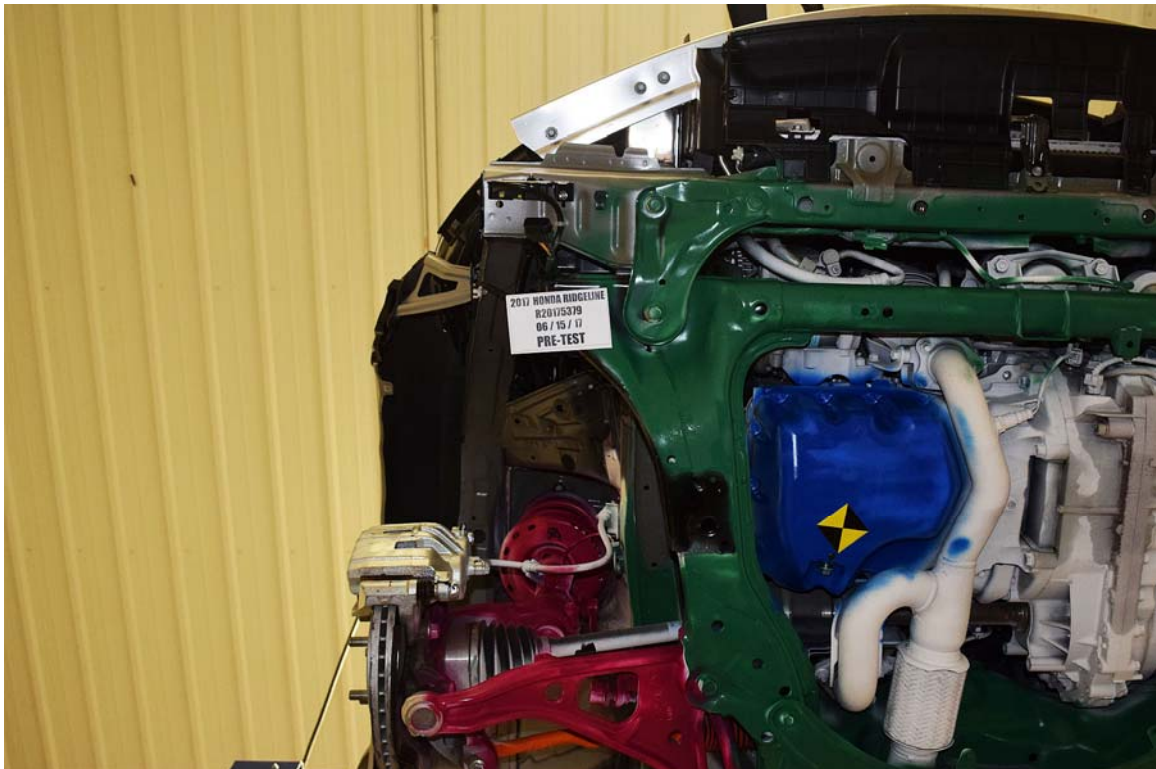
FIGURE 144. Pre-Test Passenger Bumper to Rail Attachments and Crush Initiators with Parts Removed
