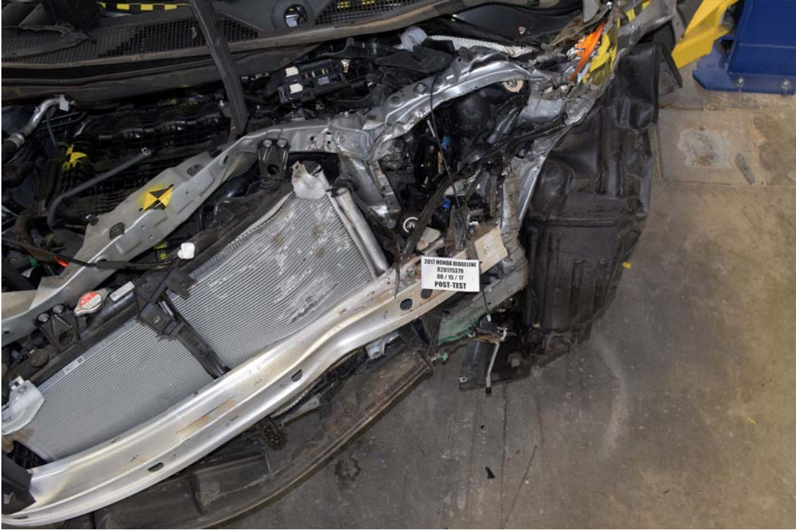
FIGURE 131. Pre-Test Left Side Energy Absorber with Parts Removed
