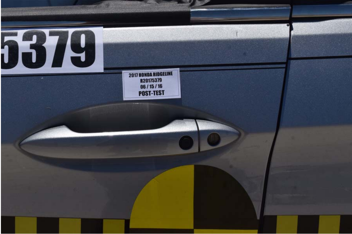
FIGURE 51. Post-Test Close-Up View of Driver Door Latch
