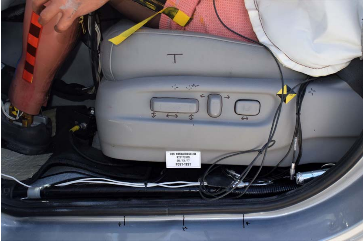
FIGURE 47. Post-Test Driver Seat Fore-Aft Markings
