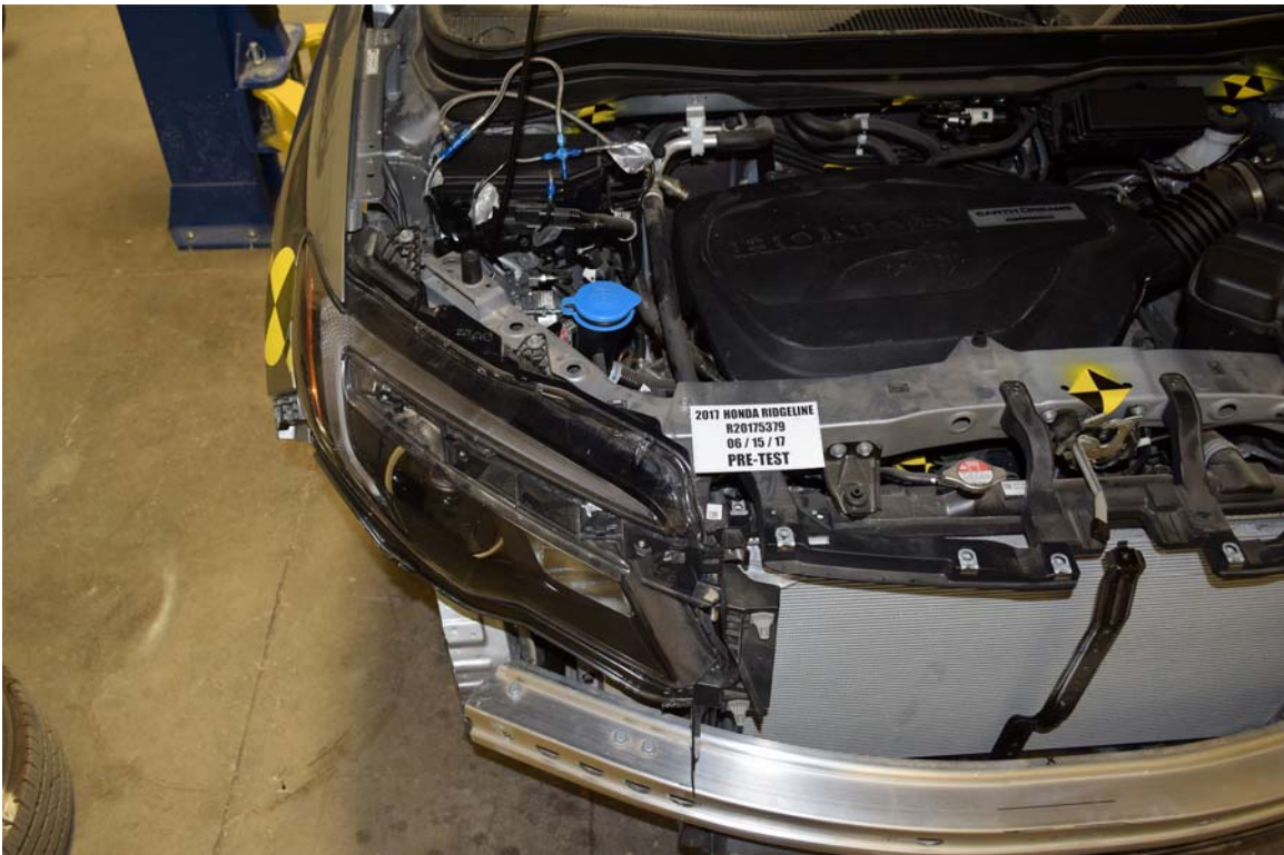
FIGURE 132. Pre-Test Right Side Energy Absorber With Parts Removed
