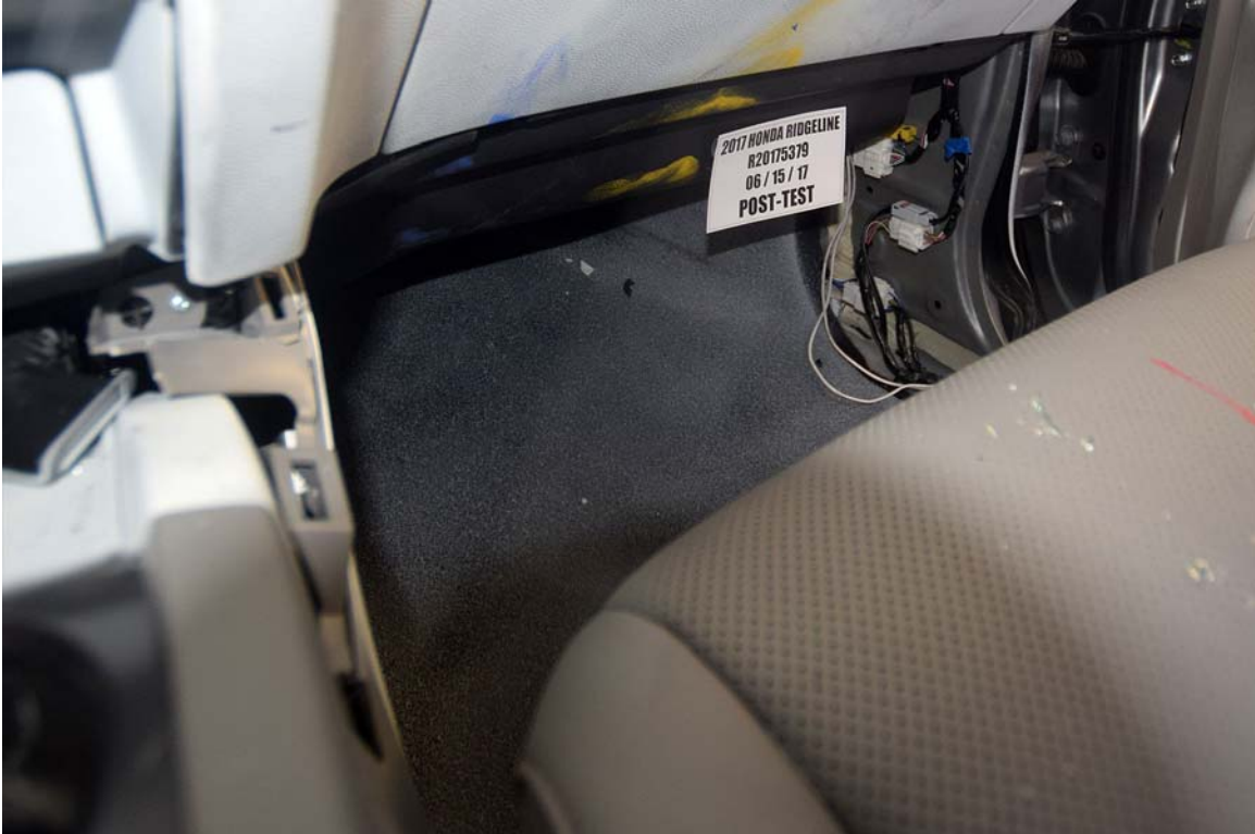
FIGURE 117. Post-Test View of Passenger Floor Pan From Center of Vehicle
