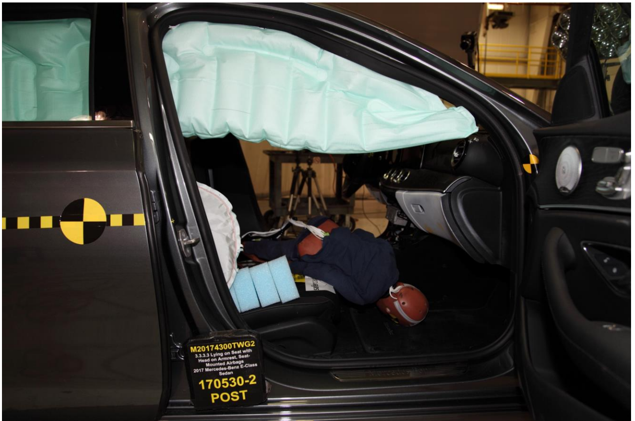
Figure A-25 Post-Test 3 Year Old Dummy - Right Side View (Door Open)
