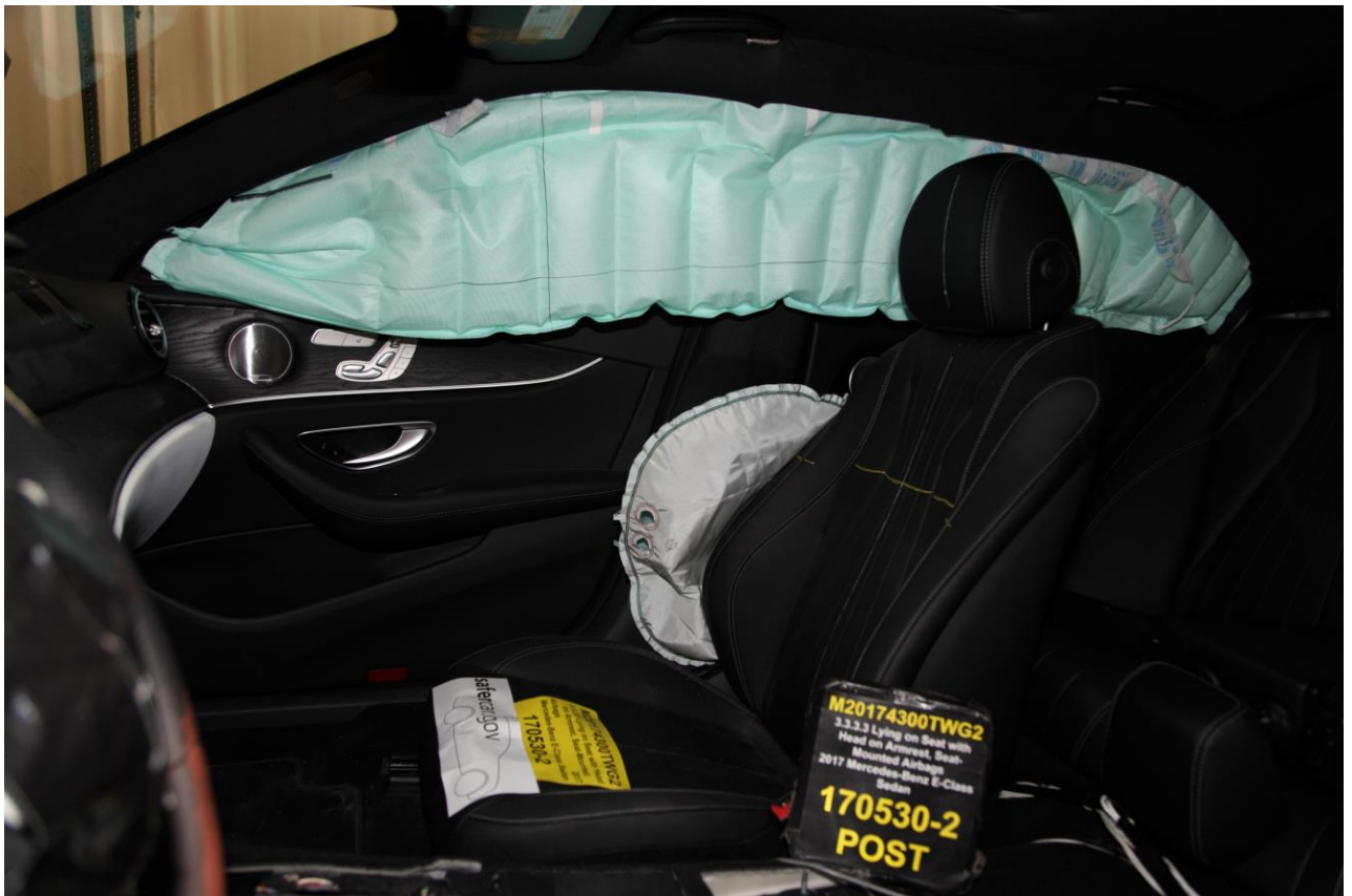
Figure A-26 Post-Test Airbags - Left Side View
