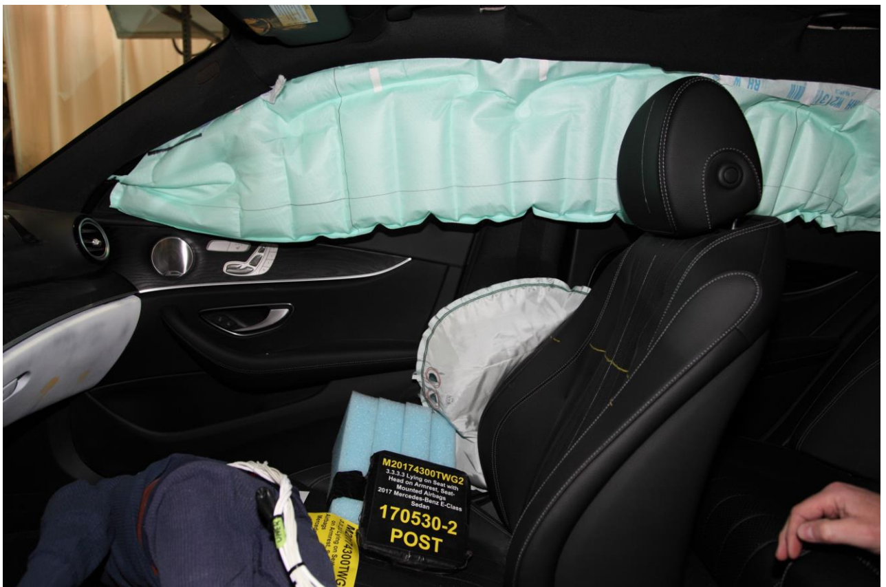
Figure A-12 Post-Test 3 Year Old Dummy - Left Side Close-Up View
