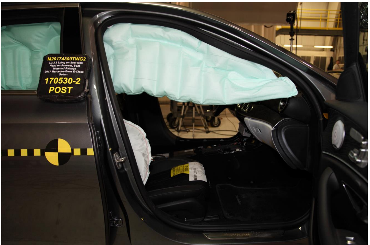
Figure A-29 Post-Test Airbags - Right Side View (Door Open)
