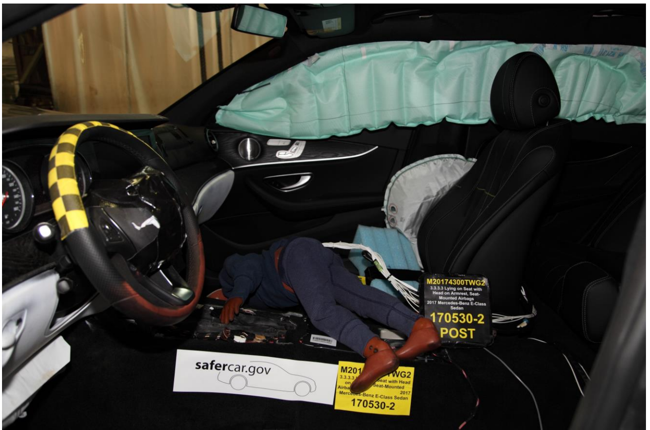
Figure A-10 Post-Test 3 Year Old Dummy - Left Side View
