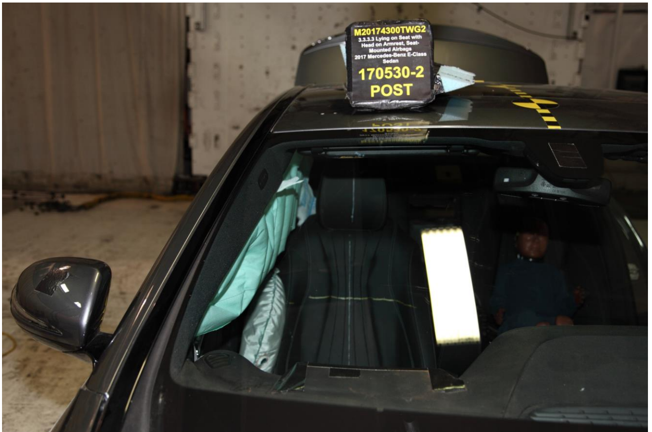
Figure A-28 Post-Test Airbags - Front View
