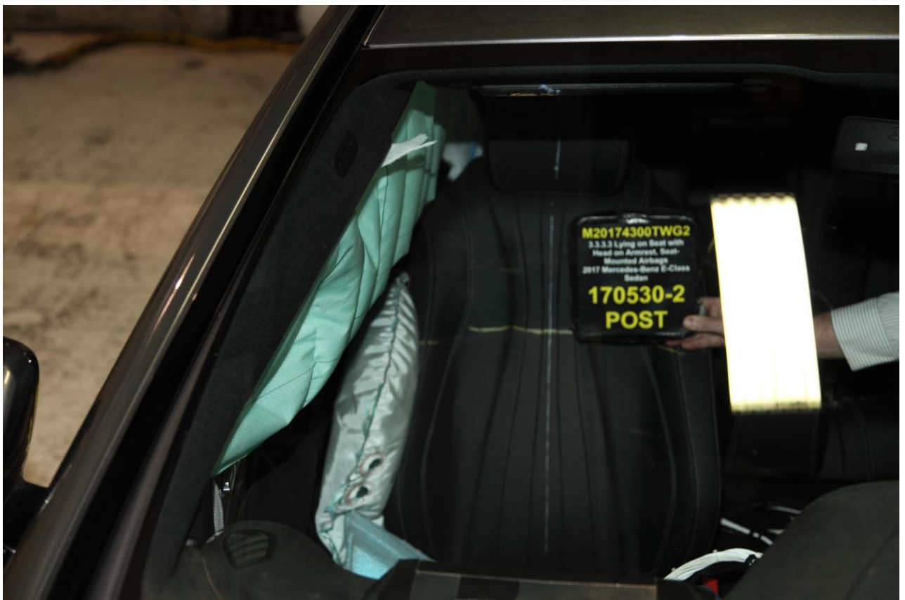
Figure A-27 Post-Test Airbags - Left Front 3/4 View
