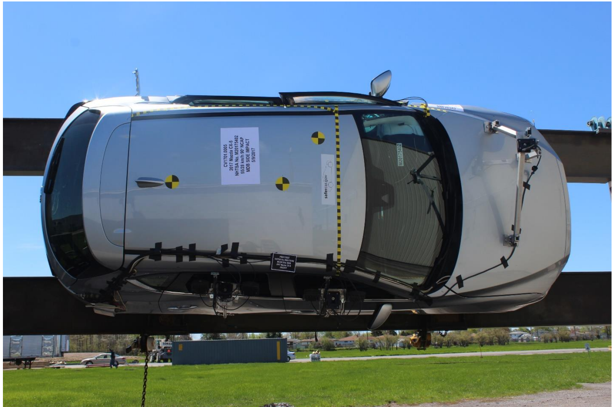
Figure A-99: FMVSS No. 301 Static Rollover 270 Degrees
