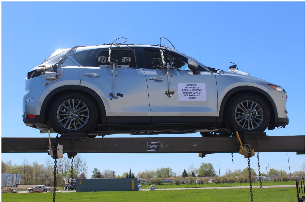
Figure A-100: FMVSS No. 301 Static Rollover 360 Degrees
