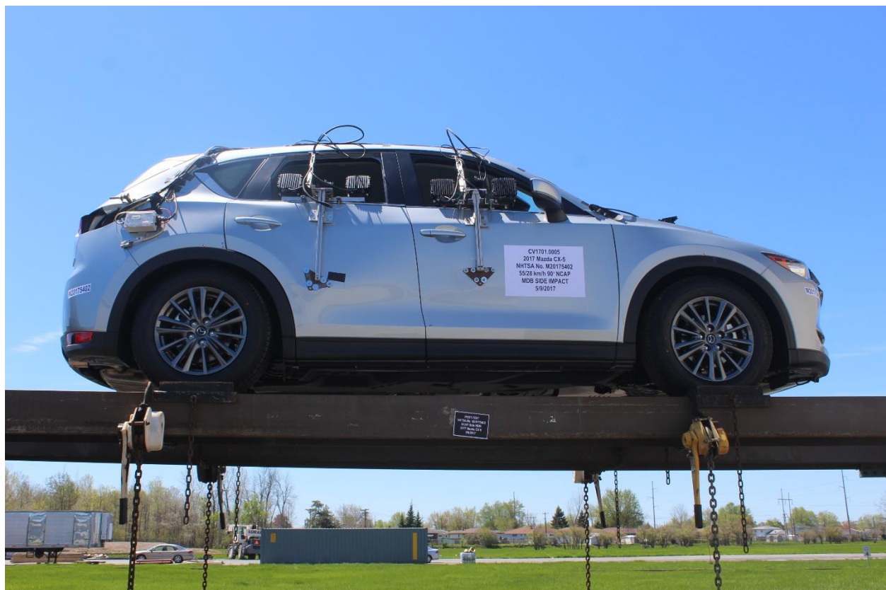
Figure A-96: FMVSS No. 301 Static Rollover 0 Degrees
