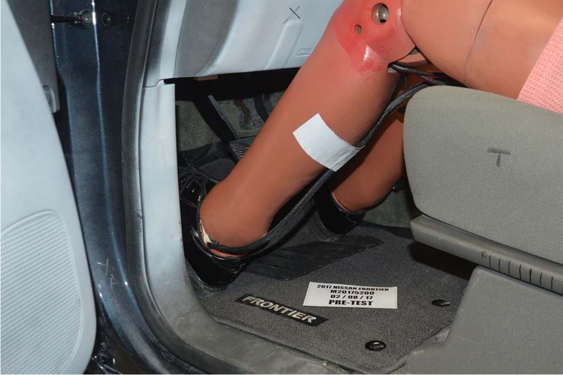
FIGURE 40. Pre-Test Driver Dummy Feet
