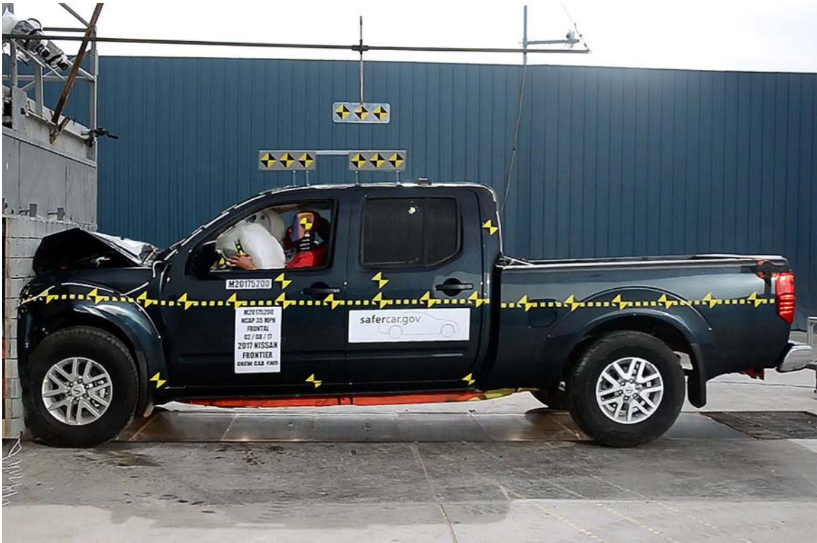
FIGURE 78. 2017 Nissan Frontier Crew Cab 4WD Frontal Impact Event
