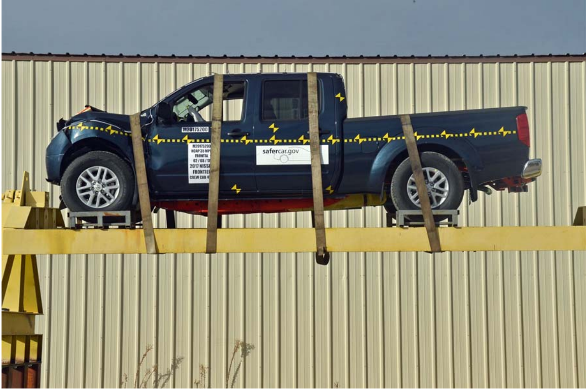
FIGURE 73. Vehicle at 0° on Static Rollover Device
