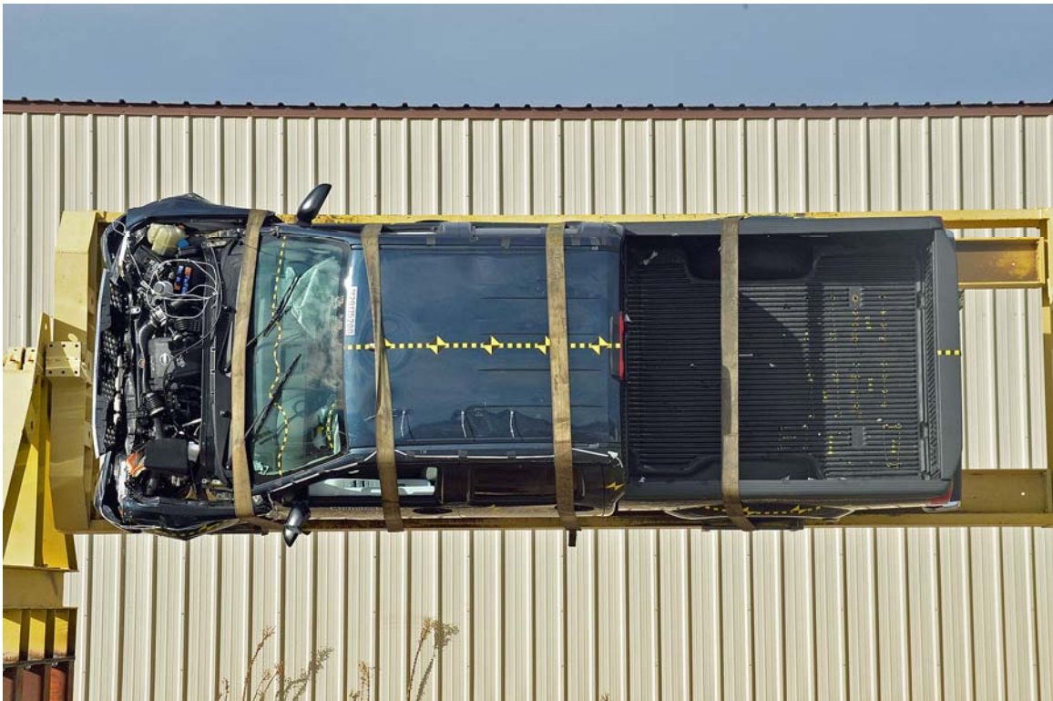
FIGURE 74. Vehicle at 90° on Static Rollover Device
