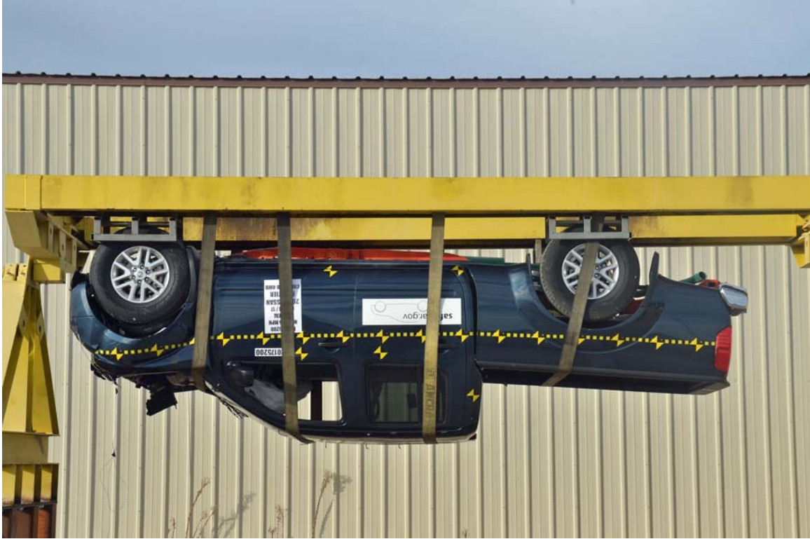
FIGURE 75. Vehicle at 180° on Static Rollover Device
