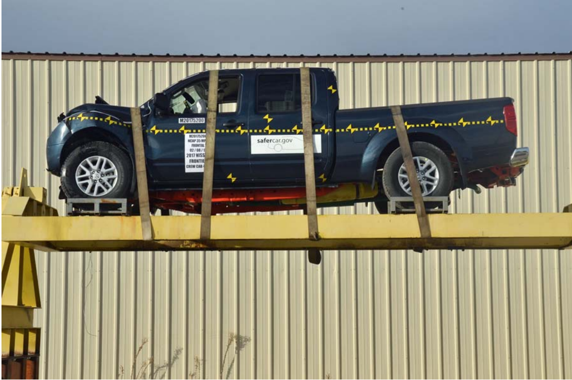
FIGURE 77. Vehicle at 360° on Static Rollover Device
