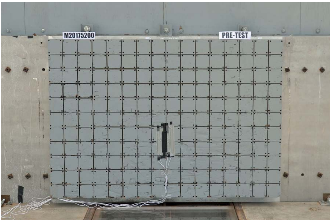
FIGURE 2. Pre-Test Load Cell Wall
