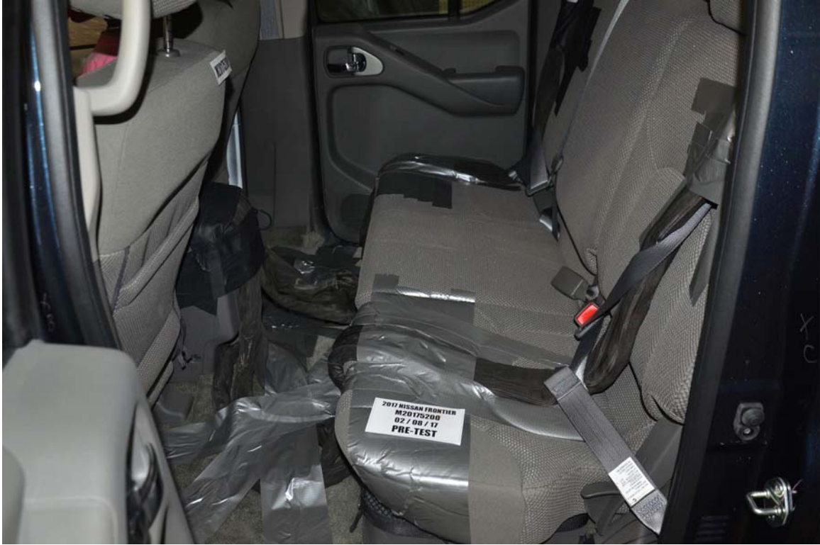
FIGURE 28. Pre-Test Dummy Cable Routing
