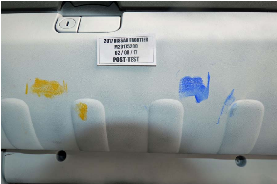
FIGURE 69b. Post-Test Passenger Dummy Contact with Knee Bolster
