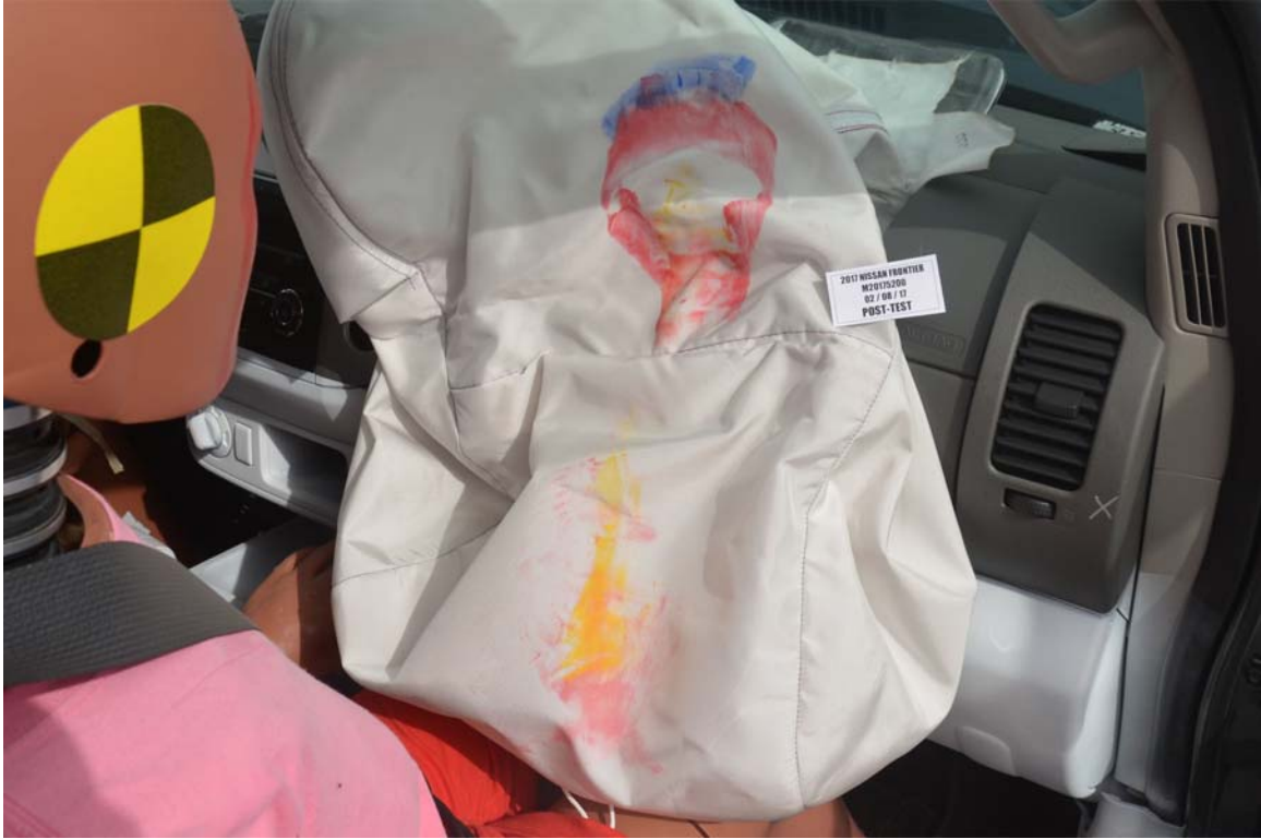
FIGURE 68. Post-Test Passenger Dummy Contact with Airbag
