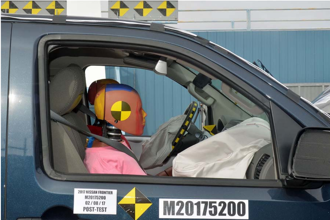
FIGURE 54. Post-Test Passenger Dummy Window View
