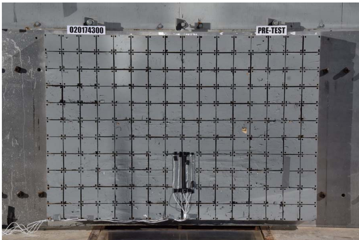
FIGURE 2. Pre-Test Load Cell Wall
