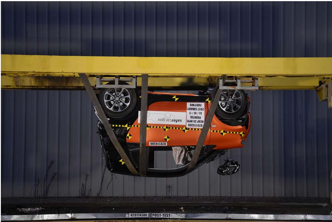
FIGURE 75. Vehicle at 180° on Static Rollover Device
