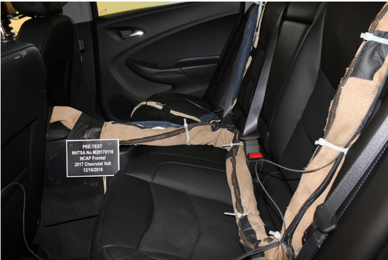
Figure A-28: Pre-Test Dummy Cable Routing
