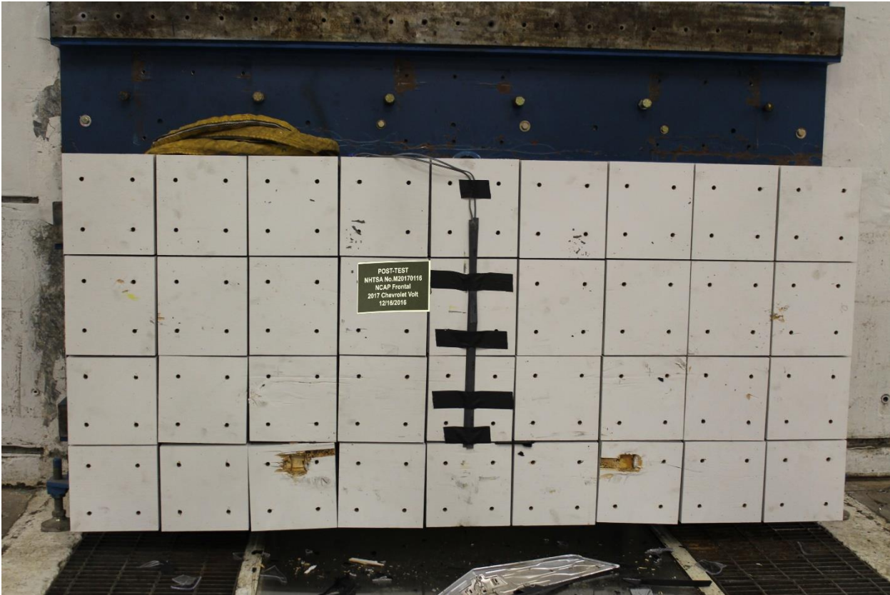
Figure A-3: Post-Test Load Cell Wall
